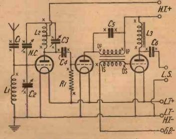
Fig. 2. Testing points in a typical circuit
