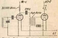
Fig. 4. Better quality is to be obtained by using a resistance feed
