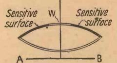
Fig. 1. The Karolus type of cell, where light passes through the circular gap or window W in the potassium, falls on the photograph A B, and is reflected back on to the photo-sensitive surface
