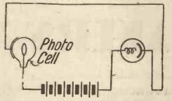
Fig. 1. An experiment with a neon lamp
