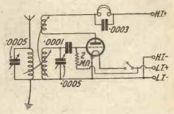
In the "B.B.C. One-valuer" (AMATEUR WIRELESS No. 388, blueprint No. AW208), we have the very simplest type of set, and one suitable for working with phones at moderate distances from a main station. The tuning arrangements provide the greatest selectivity, which is a factor of the utmost importance when the set is being operated close to such a powerful station as Brookmans Park. It is important to note that this receiver is made up on a circuit officially recommended by the B.B.C.
