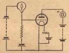
Fig. 3. The circuit used for movietone talking films
