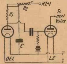
Variable resistance in filter circuit
