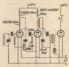
Fig. 5. When the anode current is very heavy a choke feed should be used
