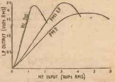
Fig. 2. Curves showing L.F. output obtained by various detector valves
