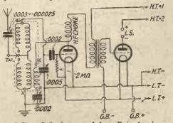
CB- CB+ "One of the best two's' yet," is the slogan which was applied to the "Talisman Two" (AMATEUR WIRELESS, No. 373, blueprint AW194) and it is amply justified. This is a very simple little set to build, and it gives amazing results. It used the new Talisman coil for tuning, and selectivity is very good. The control of the set is simple, and it is the very set for the family. The circuit is shown above.
