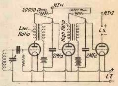
Fig. 2. When there are two stages, the first may have a low-ratio and the second a high-ratio transformer
