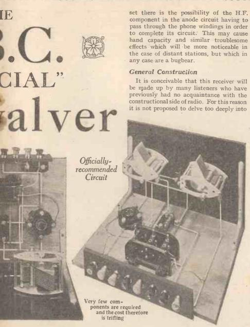
coil for reaction, which gives a boost up to signal strength, up to the point of oscillation, beyond which one should not go. Each coil is tuned by means of a .0005microfarad condenser. These two condensers are placed on the panel.
