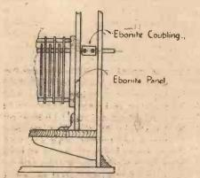
Fig. 2. Condenser mounted on small secondary ebonite panel
