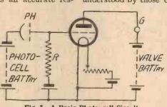
Fig. 1. A Basic Photo-cell Circuit
