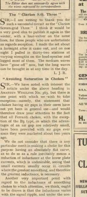
to be drawn is that the inductance varies with the signal ripple, and under the conditions that are sometimes used for measuring this inductance-for example, when employing thermal instruments-the ripple voltage must be considerable, and therefore the inductance indicated is greater than the effective inductance under working, FERRANTI, LTD. conditions.
