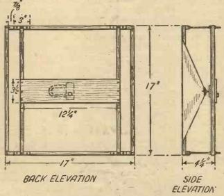
**Elevation and Section of the Speaker Frame**
