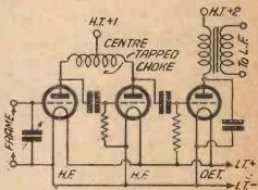
Fig. 2. Simple way of saving an H.F. choke
