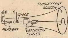
Fig. 1. Cathode-ray Oscillograph
