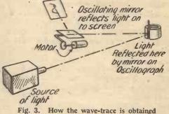
and the wave form will appear to grow or to diminish. If we do other things to the circuit, we can observe the results in much the same way. We can even, if we like, arrange two oscillographs throwing a spot of light on to the same screen, one of which records the voltage across the circuit and the other the current. Another very popular oscillograph is the cathode ray type. In this a pencil of electrons is produced from a heated filament. I will describe this at length in a further article.
