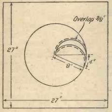
Diagram showing method of cutting diaphragm
