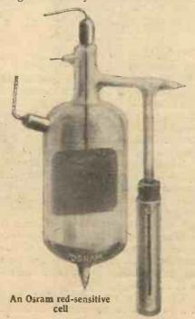
bulb. The cathode is a circular wire grid, arranged above the metalised inner surface of the bulb so that while it offers the least impediment to incoming light it is sufficiently close to attract the electrons emitted from the cathode.
