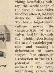
it is in them that we require a very long straight portion of the characteristic. Supposing that the plate voltage is falling whilst that of the grid battery remains up to the mark, each of the notemagnifying valves may be turned into a bottom-bend detector, suppressing or seriously mangling the negative halves of the waves.
