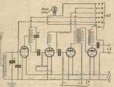
omitted. We reproduce herewith the diagram showing the complete connections. The neon lamp should be connected directly across the H.T. positive terminal to the last valve and H.T. negative, as shown in the accompanying diagram.
