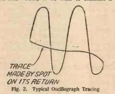
current at a frequency of 10,000 cycles per second, we can arrange our deflecting force to have a frequency of, say, 2,500 cycles per second, giving us four complete oscillations without any difficulty. Consequently, by the use of an arrangement of this sort, we are able to examine periodical varia-
