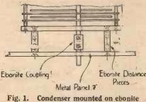
Fig. 1. Condenser mounted on ebonite stand-off insulators
