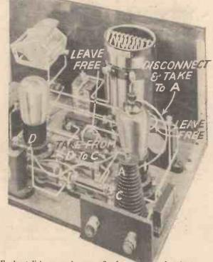
For long-distance work remove flex from A and take to terminal of S.G. valve; remove wire from C and take to D; connect wire No. 38 to B and wire No. 37 to A
