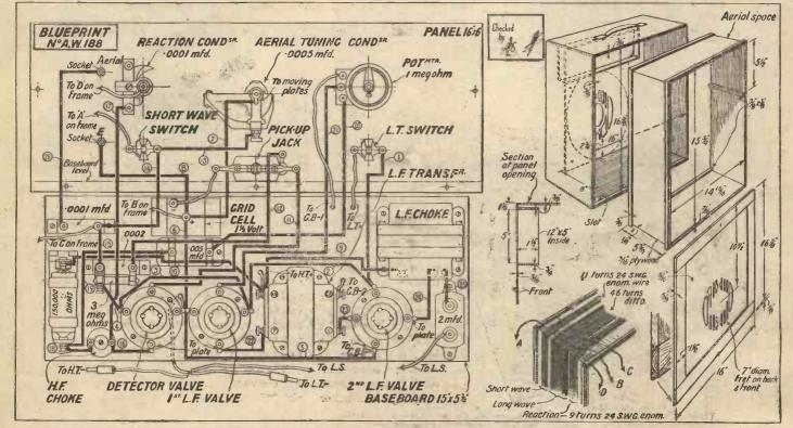
The wiring diagram, with constructional details of case and frame aerial
