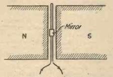
Fig. 1. Principle of the Duddell oscillograph
