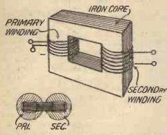
Details of a simple core-type power transformer
