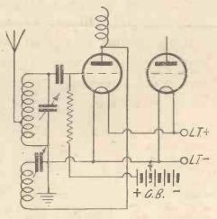
Fig. 1. A Method of Stabilising Reaction
