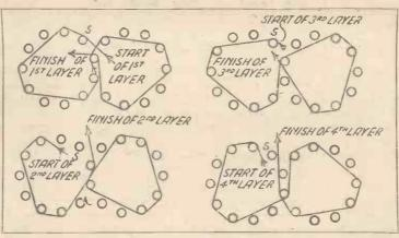
Fig. 4.-System of winding long-wave colls
