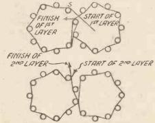
Fig. 3. System of Winding for Broadcast Waveband
