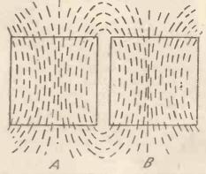
Fig. 1. The Lines of Force of a "Figure 8" Coil
