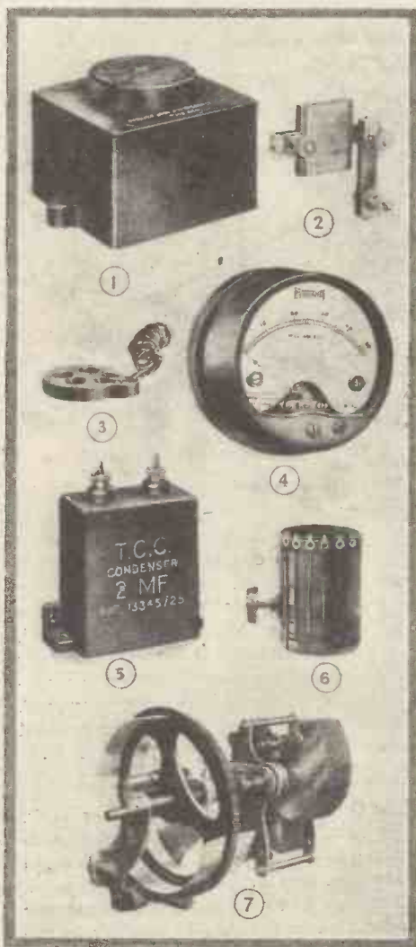
1. Dubilier Anti-interference Unit (Stands 102, 103). 2. Met-Vick Fixed Condenser (Stands 32, 41). 3. Met-Vick A.C. Valve-holder Adaptor (Stands 32, 41). 4. Ferranti Milliammeter (Stands 84, 85). 5. T.C.C. Fixed Condenser (Stand 121). 6. Eagle Engineering Reaction Tuner (Stand 139). 7. Igranic Drum-control Condenser. (Stands 53, 54, 75).
