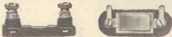
Fig. W 19.—The Fixed Condenser.
