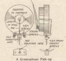
4B.A. round-headed screw, to which it is then soldered. The screw is also soldered into the half of a wire connector. These connectors are sometimes known as "barrel connectors."
