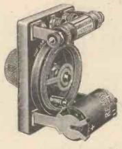
This Unit is an electrically controlled Carborundum Detector and is adaptable to all detector circuits. This is because of the resistance controlling feature whereby the Detector may be made to match the impedance of any circuit. The unit control is exceptionally fine and smooth, accu-rate to about 1/1000th of a volt. The Unit consists of a fixed detector, high-resistance potentiometer, built-in mica con
