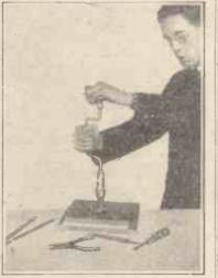
Much time and labour can be saved in cutting large holes in ebonite panels for meters, valve windows, etc., by the use of a disc cutter held in a brace.
