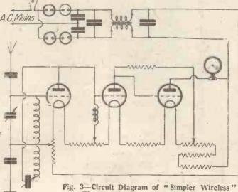
Three-valver for use on A.C. Mains
