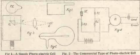
Fig 1-A Simple Photo-electric Cell Fig. 3-Photo-telegraphic Transmitter Fig. 4-A Photo-electric Relay
