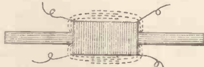
Fig. 3.—Transformer Core Wound
