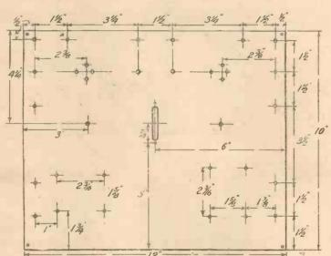
Fig. 1.-Layout of Panel.
