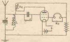
Fig. 7.-Circuit with Magnetic Reaction.
