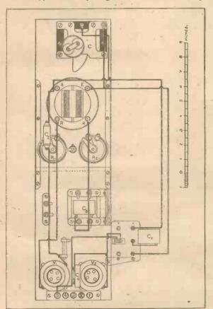
Fig. 5.—Diagram of Second Stage of Wiring.
