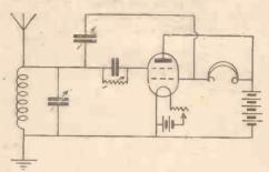
Fig. 8.—Circuit with Capacity Reaction.
