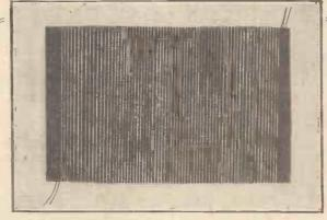
Photograph of Selenium Cell in the Course of Construction.
