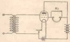
Fig. 11.-L.F. Circuit with Two-grld Valve.
