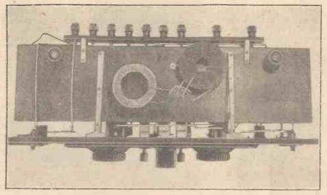
Under-side View showing Tuning Coils.
