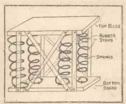
Fig. 2.—Construction of Anti-vibration Base.
