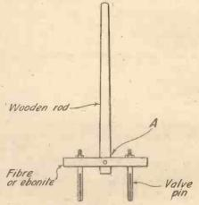
Fig. 3.—Support for Coil.
