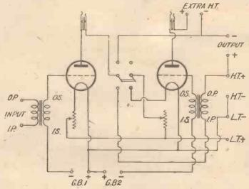
Fig. 2.—Circuit Diagram of Power Amplifier.
