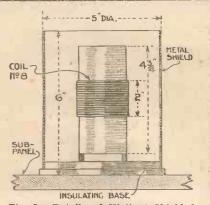
Fig. 9.—Details of Walbert Shielded Coil.
