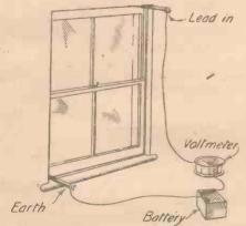
Method of Testing Aerial Insulation.
