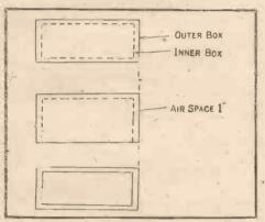
Fig. 1.—Construction of Sound-proof Box.
