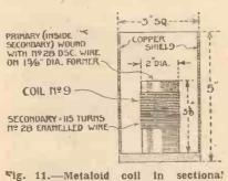
elevation. Inductance of secondary, 320 microhenries. Resistance (average), 9.5 ohms. Figure of merit, 33.7.
