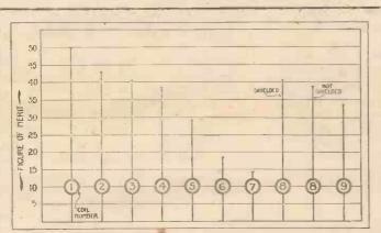
Fig. 10.-Comparison of Low-loss Colls."
