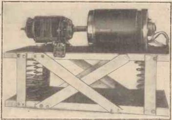
Photograph showing Generator Mounted on Anti-vibration Base.
