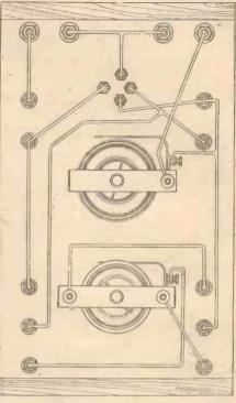
Fig. 3.-Connections on Eack of Panel.
