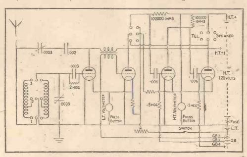
second valve. The other connections to the transformer are by flex, so that they may be readily altered. One length of flex from the opposite end of the secondary coil passes along the back edge of the baseboard so as to cross to the grid bias battery.
