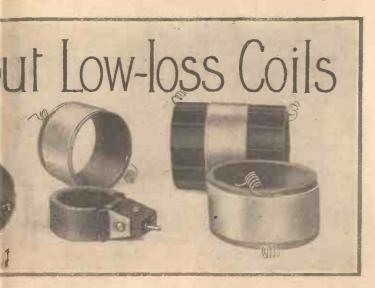
coil, the Walbert coil; which is shown in section by Fig. 8. The former is an lebonite tube of 2½-in. diameter; this is awound with fairly fine wire, namely, 50 turns per inch. When wound, the coil is enclosed in a metal shield (Fig. 9) to prevent interaction with adjacent coils. A remarkable feature of this design is that the shielded coil shows an even higher efficiency than the unshielded coil.
