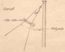
Arrangement of Halyards and Pulleys.
