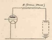
Fig. 3.—Anode Circuit with Resistance.
