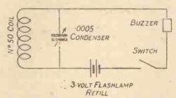
Circuit Diagram of Substitute for Wavemeter.
