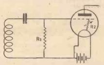
Fig. 1.—Diagram showing how the Grid Leak Functions.
