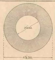
Fig. 6.—Toroid coil, wound with No. 20 d.c.c. wire, supported by Bakelite frame. Inductance, 180 microhenries. H.F. resistance at 400 m. = 9.8 ohms. Figure of merit, 18.4.
