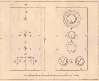
Fig. 2.—Layout and Plan of Panel.
