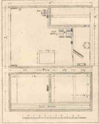
Fig. 10.—Elevation and Cross Section of Cabinet.
