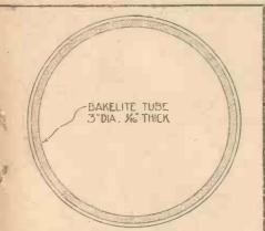
Fig. 5.—Single-layer solenoid, wound with No. 22 d.s.c. wire. Length of winding, 1½ in. Inductance, 153 microhenries. H.F. resistance at 400 m. = 5·2 ohms. Figure of merit, 29·5.
