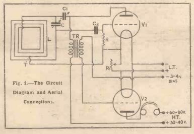
the rectifying valve are used, but as there are variations with valves it is advisable to vary the plate voltage above and below the value given to find the best working conditions
