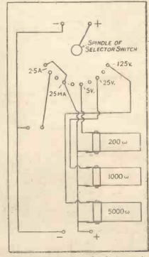
Fig. 10.—Connections for Instrument.
