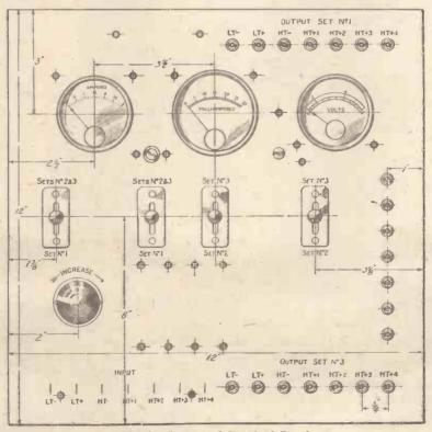
Fig. 1.-Layout of Front of Panel.
