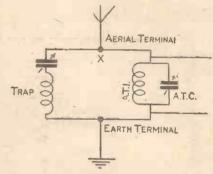
Fig. 2 .- An Effective Wave-trap Arrangement.
