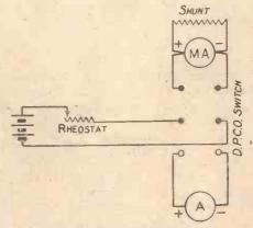
Fig. 6.—Circuit for Testing Shunt.
