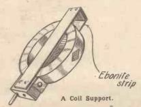
such as that illustrated in the accompanying diagram, which will assist the insertion or removal of the coil. For the sake of neatness of appearance thin strips of ebonite are used for the side supports but there is, of course, no reason why wood should not be used. Countersink-head screws are used to attach the side supports to the coil socket. These holders will protect the windings from a great deal of damage and, if neatly made, add to the appearance of the coil.
