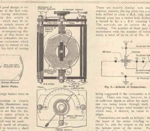
Fig. 1 .- Elevation and Plan of Variometer Tuner.
