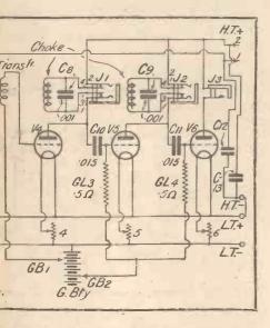
own grid battery tapping the plate current can be kept down to reasonable dimensions when a general-purpose valve is in the holder.
