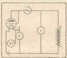
Fig. 2 .- Circuit of Testing Set.
