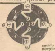
Valve sockets and springs are locked together by a mechanical process, making a definite and permanent connection. Bakelite mouldings, nickel silver springs and phosphor bronze valve sockets. Nickel plated.
