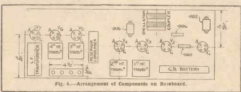
A full-sized reproduction of this sketch should be made and then pasted on the ebonite panel, and the requisite centres punched by means of a suitable tool.
