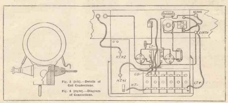
were made of parts out of the "junk" box, and their method of construction is shown in Fig. 3. It is not imperative to make up this special arrangement, as the Igranic firm market a similar coil which they term the Unitune Major.
