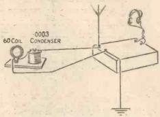
Fig. 3.—A "Hook-up." Wave-trap.
