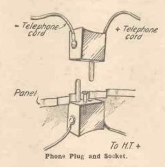
circuit. The type of plug and socket illustrated is absolutely irreversible and is therefore quite suitable.
