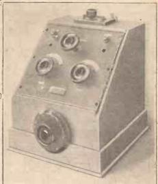
Photograph of Complete Receiver showing Tuning Controls
