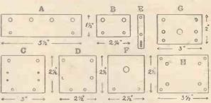
Fig. 5 .- Details of Sub-panels.
