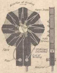
Fig. 2.-Constructional Details of Coil
