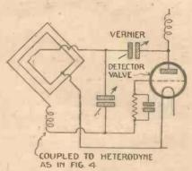
Fig. 10.-Capacity-reaction Coupling.
