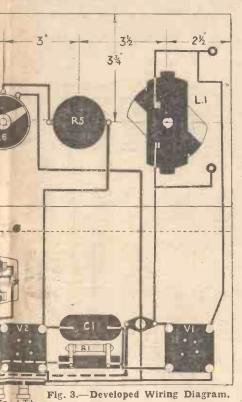
degrees the windings are in parallel and for the second 180 degrees they are in series. This gives a continuously variable tuning control from 250-1,650 metres. The switches S1, 2 and 3 are shown separately for clearness, but are really controlled by one lever.
