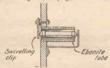
Details of Grid Leak Mounting.
