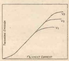
Fig. 3.—Emission and Fliament-current Curves
