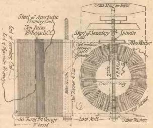
Fig. 2.—Details of Variocoupler.
