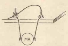
Fig. 8.—Adjusting the Ammeter Shunt.
