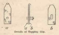
small B.A. screw and nut or terminal A hole is bored through a to receive the screw, while in b a slot is cut so that, when assembled, the piece b is pressed down on the wire to be tapped. This holds the wire firmly in the hook at the end of a when the parts are clamped together by the nut or terminal head.
