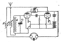
Fig. 2.—Suggested Circuit for Short-wave Receiver.
