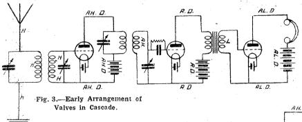
waves and so the current flowing in the plate circuit of the detector valve consists of a direct current modulated at speech frequencies. As before, only the fluctuating component induces a corresponding current in the secondary of the transformer, which causes the potential of the grid of the last valve to fluctuate and vary the direct current through the phones so that the telephone diaphragm produces audible signals.
