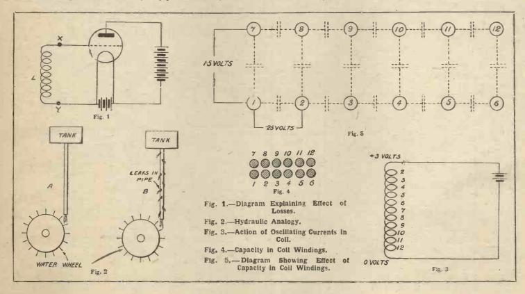
difference of 1.5 volts between the first turn and the seventh, the second and the eighth and so on.
