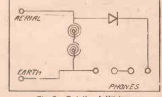
Fig. 3 .- Details of Wiring.
