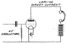
Fig. 2.—The Valve as a Detector.
