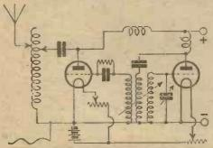
Fig. 40.-A Typical Master-oscillater.
