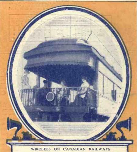
The Library car of a Canadian National Railway trans-continental express, equipped with a wireless receiving set. The aerials can be plainly seen, the wires extending from above the observation platform to the front of the car.
