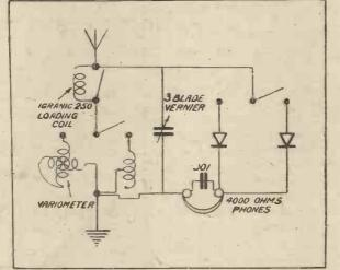
Circuit Diagram of the Crystal Receiver with which the author received K D K A of Pittsburgh, U.S.A.
