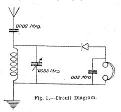
Wiring is carried out with No. 18 tinned-copper wire according to the circuit diagram shown in Fig. 1. A wiring diagram is shown in Fig. 2 for those who
