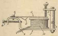
Fig. 5.—Details of Buzzer.
