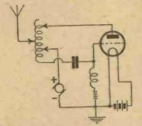
Fig. 34.—Dispensing with the Radio Choke.
