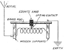
Fig. 2.—Diagram of Slider Inductance Connected to Aerial.
