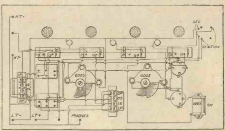
Fig. 3.-Wiring on Under Side of Panel.
