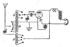
Fig. 1.—Circuit Diagram of Reinartz Receiver.
