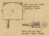
Fig. 36.—Details of Reaction Coil Mount.
