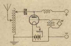
Fig. 37 -The Principle of the Masteroscillater.
