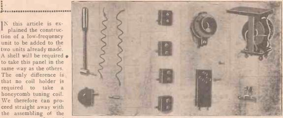
Figs. 28a and 28b .- Component Parts of L.F. Amplifying Panel and Reaction Unit.
