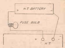
Fig. 3.-Method of Connecting Fuse.
