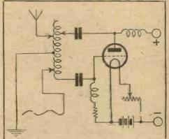
Fig. 33-An Arrangement of Counterpoise
