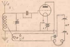
Fig. 1 .- Typical Single-valve Circuit.
