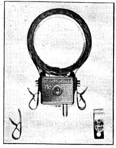
Clips Mounted on Coil Base.
