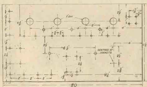
Fig. 2.-Drilling Plan of Panel.
