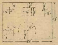
Fig. 5.-Layout of Panel.
