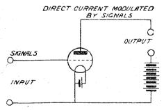
Fig. 1.—The Valve as an Amplifier.
