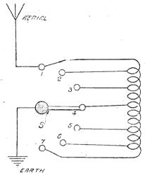
Fig. 1.—Diagram of Variable Industance Connected to Aerial.
