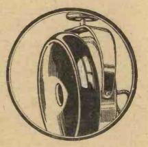
The ebonite cap of the earpiece is screwed on by special apparatus to a marked degree of tightness. It is almost impossible to unscrew it without a wrench. This means more accurate clearance distance between the diaphragm and the faces of the pole pieces and guards against distortion. what is more important, it defeats any casual attempt to unscrew the caps, which, once done, destroys the Matched Tone adjust-
