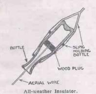
A sling of cord or wire is made with which to fix the bottle to the mast or wall hook. Next a piece of wood is cut which will pass through the bottle neck and as long as the internal diameter of the bottle. This piece of wood is dropped inside the bottle and a loop is made on the end of the aerial wire, and this also is passed inside.
