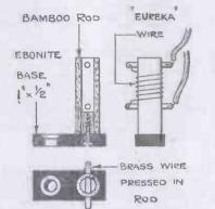
Fig. 6.—Details of Fixed Resistance.
