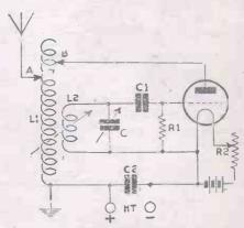
Fig. 21.—Circuit Diagram of Single-valve Transmitter.
