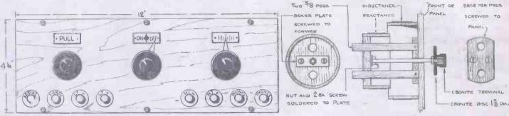
Fig. 3.-Front View of Panel.
