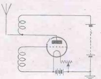
Fig. 20.—Principle of Valve Transmitter.
