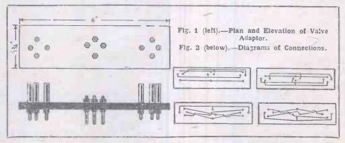
powerfully, he hit upon the idea of working two valves in parallel on the receiver. This arrangement resulted in at least an increase of fifty per cent. in signal strength, while the impedance of the extra valve did not seem to affect the working simple, effective and inexpensive, and can be applied to existing receivers when required without any internal alterations of
