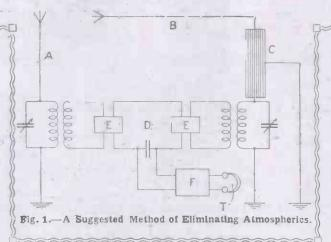
The ordinary electromagnetic wave travelling over a good conducting surface is known to consist of a vertical electric field and a norizontal magnetic field, both field only, with no magnetic component. If, therefore, the receiving system as a to the magnetic component of the field, it will be unaffected by atmospherics.
