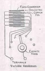
the capacity increased or decreased by means of a switch arm. For fine tuning this can be shunted by a vernier condenser if desired.
