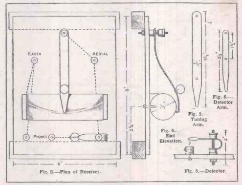
be 234 in. from the front edge (Fig. 2). Terminals for aerial, earth and telephones may now also be screwed into position.
