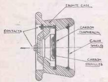
Fig. 1 .- Section of Carbon-type Microphone.
