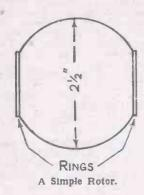
rings should be fitted over the holes to form the flanges on which to commence the windings. The cardboard rings will adhere quite firmly if glued on, but rubber rings can be affixed with rubber solution.
