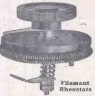
With finished and lacquered brass bush for panel mounting. Resistance wire wound on insulating rod, thereby giving perfectly smooth adjustment. Each supplied with diagram giving drilling dimensions.
