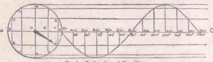
Fig. 4.—Explanation of Sine Wave.
