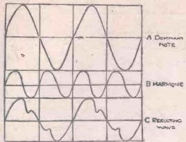
Fig. 3.-Composition of the Compound Wave.
