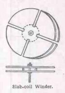
deep in the centre washer; then lock the washer and cheeks together with three nuts. Wind your coil and bind by putting a thread through the slot in the centre washer, over the top and through again. Do this two or three times at each of the four slots and your coil is finished and ready for work.
