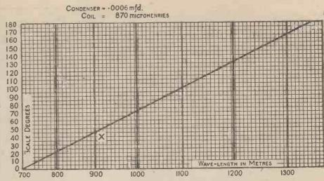
Fig. 2.-Calibration Chart for Inductance Ccil.
