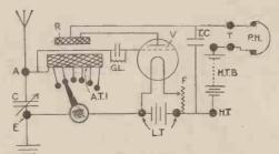
Fig. 4.—Circuit Diagram of Portable Receiver.
