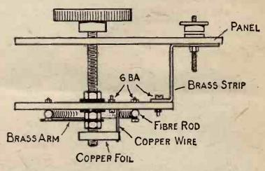
Fig. 3.—Enlarged Detail of Filament Rheostat.
