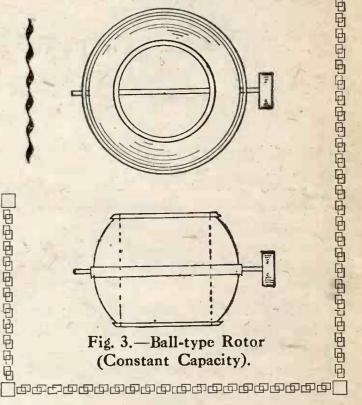
ing must be put on in two parts and joined at the centre, as it is only possible to wind "up the hill." The winding should be started at each end and continued upwards (inwards), and the two ends then soldered together and tucked inside.
