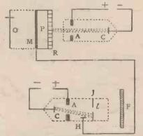
Fig. 4.—Diagrammatic Suggestion of Cathoderay Transmitting and Receiving Apparatus.
