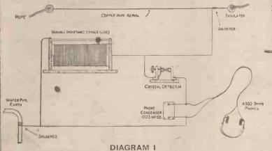
Diagram 1 (above) shows the method of connecting up a singleslide tuning inductance to a crystal detector. This manner of coupting is termed. "direct-coupling."
