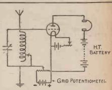
Fig. 2.—Diagram showing Adjustment of Grid Voltage.
