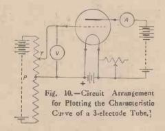
commit it to paper in the form of a curve. The most useful correlation of these variable factors is that which shows the proportion existing between the applied grid voltage and the resultant plate curplate-current characteristic.
