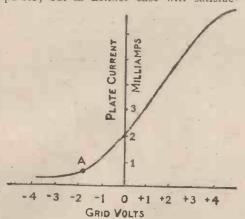
Fig. 1.—Graph showing Characteristic Curve of Valve.
