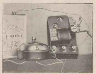
Fig. 1.—Photograph of Transmitter.
