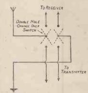
Fig. 3.—Connections of Change-over Switch.
