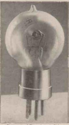
Photograph of Three-electrode Valve.
