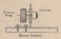
knob the crystal can be moved so that any point on its surface can be touched by the metal contact. This is an improvement on the common ball-and-socket movement, as once the sensitive point is found the crystal is held in position by tightening the knob.
