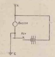
Fig. 2. - Circuit Diagram of Simple Transmitter.
