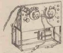
Fig. 1.—The C Mark III Low-frequency Amplifier.
