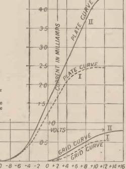
the applied grid potential for each curve is plotted in the same manner as described with reference to Fig. 10, the separate curves representing a different value of steady plate high-tension in each case.
