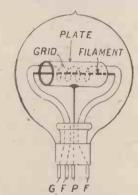
Fig. 9.—Three-electrode Valve shown Diagrammatically.
