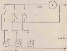
Circuit Diagram showing Arrangement of Switches.
