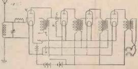
Fig. 3.—Addition of Detector Valve to C Mark III Low-frequency Amplifier.
