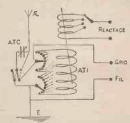
Fig. 6.—The Single-circuit Receiver with "Series-parallel" Condenser and Tapped Reactance Coil.
