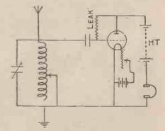
Fig. 10.—Another Grid-leak Connection Diagram.
