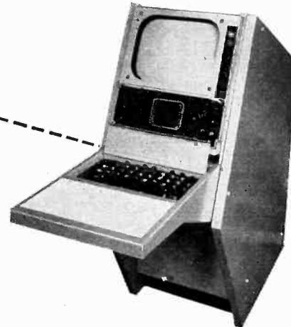
Preset controls on the Camera Control Panel are under a hinged cover — here shown open. A 14" picture and 5" waveform display are provided by the BD 873 Monitor.
