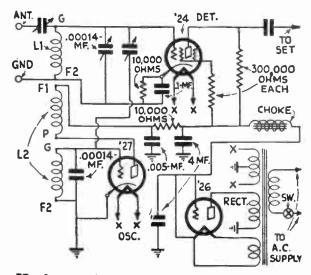
Hook-up of Leutz S.-W. adapter; only two wires connect to B.C. set.
