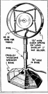
soldered. The rings for the microphone springs are made of No. 16 wire formed around a lead pencil. They should be attached to the large ring through small holes, drilled 5½" apart, soldered firmly on both sides, ar-1 smoothed down with a
