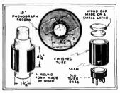
record is heated over a gas flame until it is soft, when you will find it possible to cut out square pieces with a knife. White still warm, wrap the flat piece around a
