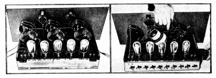
Two interesting photos of Mr. Lenck's short-wave phone and code transmitter constructed from a once-famons nentrodyne receiver, which he hanled down ont of the attic.
