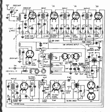
Wiring diagram for the "short-wave" superhet receiver installed on the yacht "Migrant."
