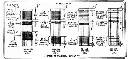
Converter Coil Data-2 coils at left 11/4" O.D.; 2 coils at right %" O.D. (Outside diameter.)
