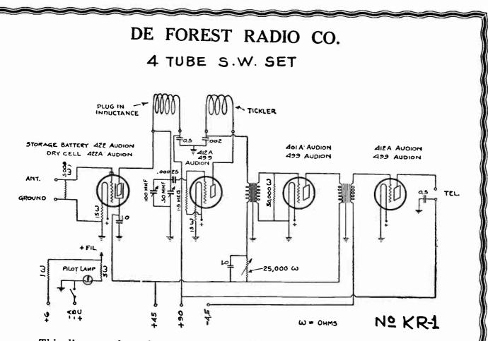
This diagram shows how the various parts of the new DeForest Short-Wave Receiver are connected.
