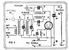
A.C. schematic diagram for the 1-tube supertegenerator.
