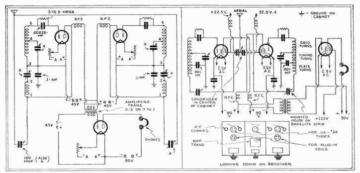
Fig. 1, at left, shows diagram of the Reinartz interference elimination receiving circuit for hattery tubes; Fig. 3, at right, shows the same circuit adapted for use with A.C. tubes.
