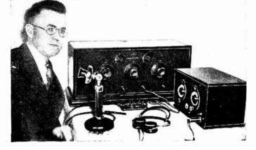
The author with his transmitter constructed from an old neutrodyne receiver.
