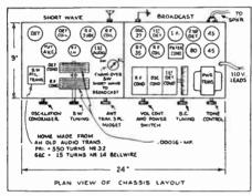
Top view of chassis layout used by Mr. Legate for his combination "short" and "broadcast" wave receiver. The short-wave receiver employs an R.F. stage, a re-generative detector, and also an audio coupling stage.
