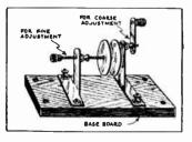
check-nut shown at left of the condenser. The second plate, at the right, may be moved side-wise by means of the lever and insulated button.
