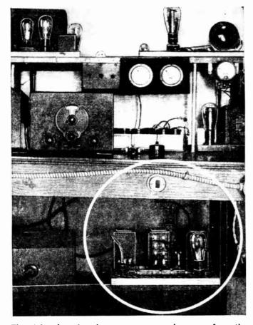
The right place for short-wave power-packs—away from the sets themselves. On the shelf just above the floor are (at the left) the factory-built power unit for the National SW-58, and (at the right) the "home-made" unit for the SW-3. A completely A.C. operated audio power-amplifier for the latter is mounted on a shelf above the tuners.
