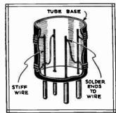
in making short-wave plug-in colls I have found an easier method of fastening the ends of the rolls to the prongs of the coll form or tube base. For IX bases take four pieces of stiff wire (as tall as heressary) just large enough to fit tightly into the prongs of the form and solder the ends of the colls to the wire. For UY use five wires, etc.—Harry' F. Sleber.
