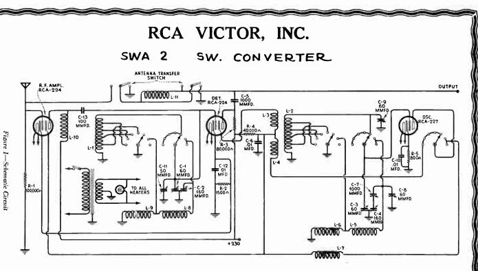
RCA Victor Short Wave Converter SWA-2 is a three tube, single control short wave unit designed to convert all short wave signals from 13.8–200 meters to a single frequency so that they may then be amplified by means of the usual broadcast receiver.
