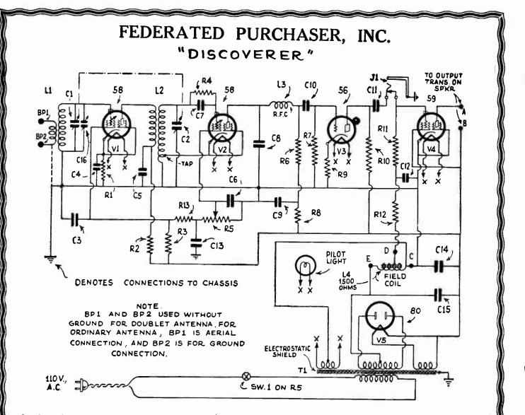
In the ordinary regenerative receiver, the tube is pushed into oscillation by means of energy feed-back from the plate circuit to the grid circuit or by some other means. The fundamental action is that of a stable tube and the tube is actually forced into oscillation by means of any one of the com-monly known methods. In this receiver, we use the opposite method, whereby the tube is constantly oscillating and has to be pulled out of oscillation for voice recep-tion or music. tion or music.
