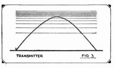
The space radiation is bent downward; more exactly it is refracted and totally reflected (at certain frequencies).
