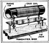
on to it, after fitting nuts into the ma-chine screw. Then, as illustrated, these should fit into tip jacks. For push-pull an additional tip and tip jack is needed at the point marked 'X'.-James L. Paul.
