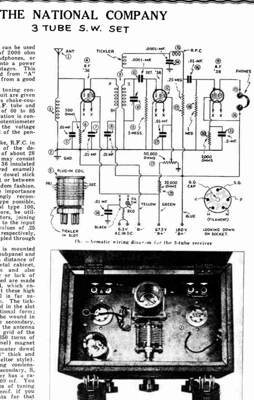
Tickler 3 turns of No. 32 Double Silk. No. 12 coils, covering from 23 to 41 meters Primary 7 5/6 turns of No. 34 Enamel Primary 7 5/6 turns of No. 34 Enamel Tickler 3 turns of No. 32 Double Silk. No. 13 coils, covering from 40 to 70 meters: Secondary 19 5/6 turns of No. 18 Enamel Primary 12 5/6 turns of No. 34 Double Silk
