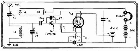
Schematic diagram of short wave megadyne.
