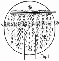
Fig. 1 shows the interior of a vacuum tube where (1) is the filament, E is the stream of electrons going in the direction of the arrows, (2) is the grid, (3) is the plate. The small dots surrounding the grid and plate indicate a layer of gas always adhering to metals, a miniature Heaviside layer, which the electrons must pierce.
