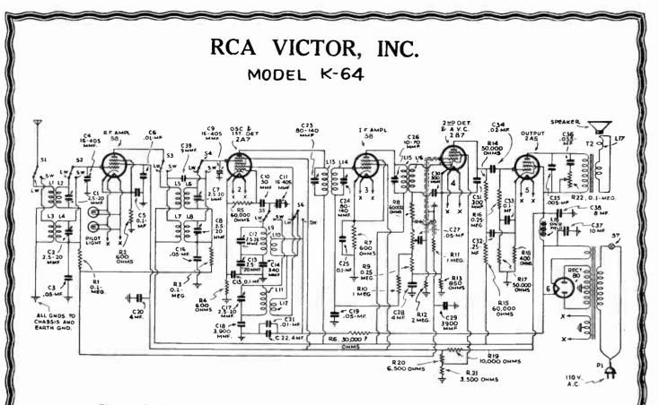
Diagram for the new RCA-Victor 2-band model, "short-wave" and "broadcast" 6-tube receiver.
