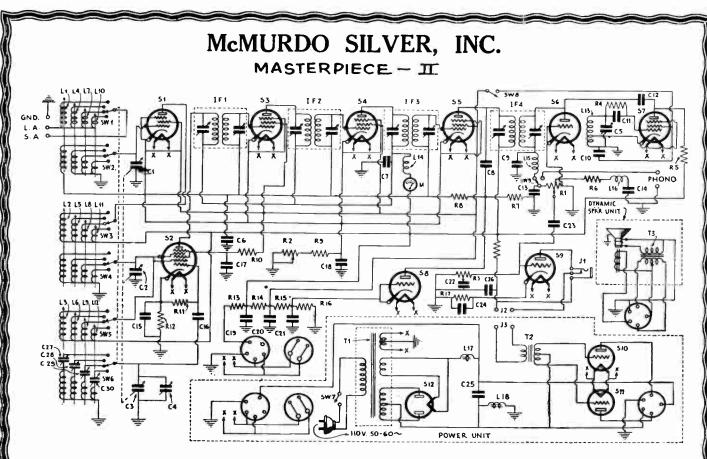
Here we have the schematic circuit diagram for the new McMurdo Silver "Masterpiece II" All-Wave Superheterodyne Receiver.
