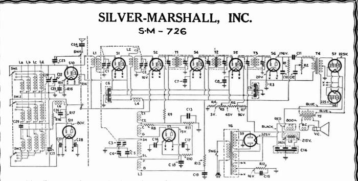
Wiring diagram for the latest "S-M"—726 SW., "All-Wave" Super-het. For short wave reception the aerial feeds into a S-W detector S-10 and oscillator S-11; in all 2 oscillators and 3 detectors are used. Tubes—S2, S-10—'24's; S3, S6, S11—'27's; S7, S8—'47's; S1, S4, S5—'51's (R. C. A. 235); S9—'80 rectifier. This set is a combination of a 9 tube vari-mu pentode broadcast super-het, and an 11 tube short wave super, using switches instead of plug-in coils. Pentodes are used at S7 and S8.
