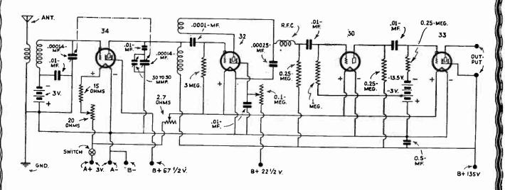
The interesting hook-up devised by the Leotone engineers, whereby maximum strength of signal is obtained, with a minimum of battery consumption. An A. C. model is also available.
