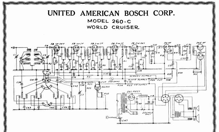
The oscillator and antenna coils are changed for each band, thus providing practically four separate and complete short-wave receivers in one instrument.
