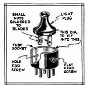
small nut on the inside of each blade and opposite the hole. Then, I drilled the tube-base for the bolks to go through the sides to the blades of the A.C. plug. The A.C. plug is slightly smaller than the tube-base, but if it is filed down close, this makes a very neat "adapter" plug. —Charles Cassell.
