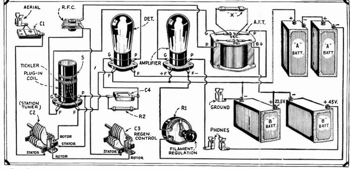
Even though you have never built a radio set, you can't help but go right with this 2-Tube "Globe-Trotter," as the "picture diagram" above shows you just how to wire it.
