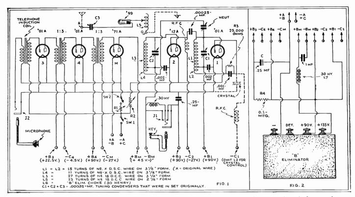
Circuit above shows how Mr. Lenck hooked up the microphone and key connections to his revamped neutrodyne receiver, which then served him as a short-wave phone and code transmitter. Fig. 2, at right, shows connections of "B" eliminator.
