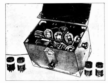
Five tubes, including the rectifier, provide this S.W. converter with a real It enables you to hear S.W. stations on your "broadcast wallop." receiver."
