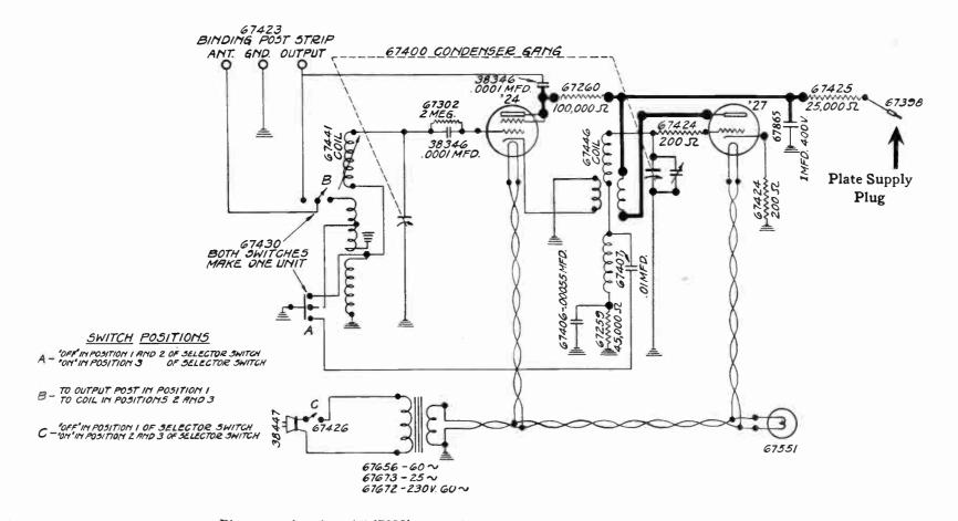
Plate supply plug (#67398) must be connected to some source of filtered D.C. at a potential of 180 to 280 volts. Recommended voltage is 250.
