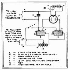
How to use two Ford spark (ignition) coils to obtain high voltage for plate supply of transmitter. The tube "V" rectifies the secondary voltage.
