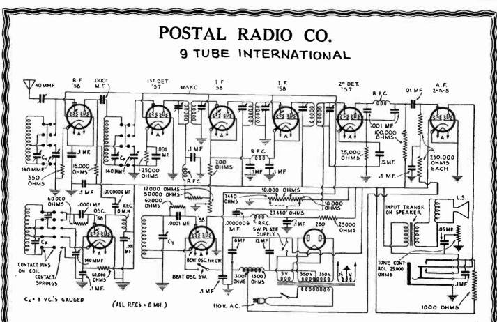
Diagram of connections used in the Postal International 9-Tube Superhet. All three coils, E.F., detector, and oscillator, are simultaneously changed in one single operation from the front panel, by a simple one-half inch movement of the complete coil shield box or "drawer"; the set being converted from ordinary tuning to band-spread tuning in a jiffy. The bands are spread over 65 degrees of the dial.
