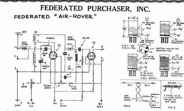
Parts List for "Air-Rover" Acratest Triple Binding Post. Aerial & Ground Connections Acratest Twin Phone Tip Jack, Speaker or Phone Connections 1¼" Piece of Bare No. 14 Wire wound over with appx. 14 turns of No. 18 insulated push-back hook-up wire. Set of Four Plug-in Short Wave Coils. These are accessories. Not furnished with kit. Coil A-200 to 80 meters Coil B-80 to 40 meters Coil C-10 to 20 meters Coil C-20 to 10 meters Acratest Triple Binding Post. Aerial & Ground
