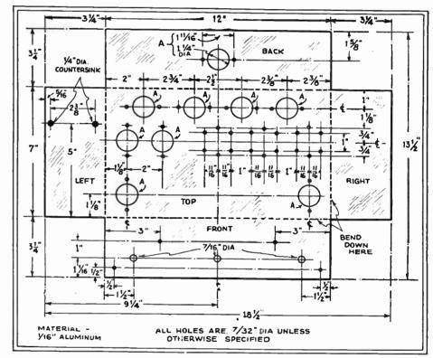
Subpanel layout for the S-tube super.
