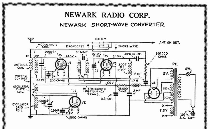
Diagram of the connections used in the Newark Short Wave Converter which includes an I.F. stage.
