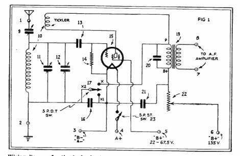
Wiring diagram for the dual-role short-wave receiver here described by Mr. Denton, its constructor.
