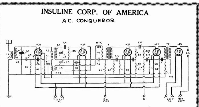
Diagram of connections for the A.C. "Conqueror" short wave receiver.
