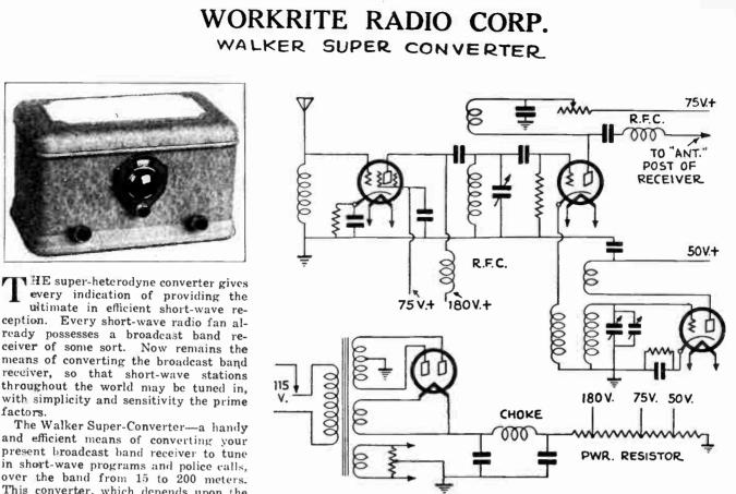
ready possesses a broadcast band receiver of some sort. Now remains the means of converting the broadcast band receiver, so that short-wave stations throughout the world may be tuned in, with simplicity and sensitivity the prime factors. The Walker Super-Converter-a handy and efficient means of converting your present broadcast band receiver to tune
