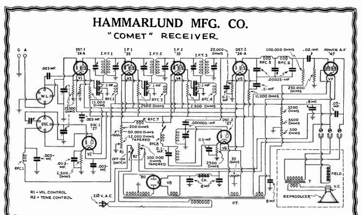
The interesting all-wave superheterodyne circuit developed by Hammarlund engineers. The wave bands from 14 to 550 meters are provided for by changing two plug-in coils at sockets "WL" and "OSC," insuring maximum freedom from dead-end losses. All circuits are fully by-passed and with the carefully designed I.F. stages, and A.F. amplifier, a signal of great volume and high quality is assured on all wave lengths.
