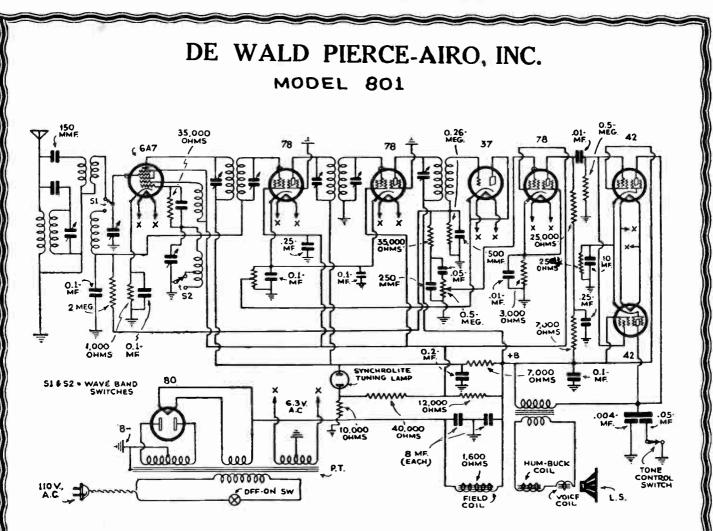
Wiring diagram of model 801 "BC" and "SW" receiver-an 8-tube superhet.
