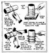
copper strlp is wound around a form and the operation aided by means of a fibre nullet. Tubing may also be wound hy walking around a stationary form with it. Copper strlp may he "cige-wise" wound between nails driven into a wooden form as shown, (or pins or screws in a metal drum or piece of pipe).
