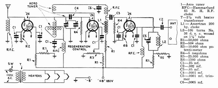
been many devices for converting the broadcast receiver into a short-wave job. The device which the writer considers to fill the gap is a combination of two recent developments in the radio field. The Aero tuner which covers the short-wave spectrum up to 100 meters, and has a single additional coil to fill the gap between that point and the broadcast band, is employed in combination with the dynatron oscillator.
