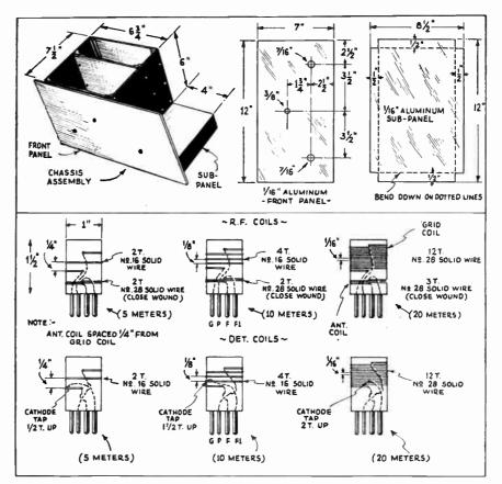
Coil Data and Receiver Chassis Dimensions.
