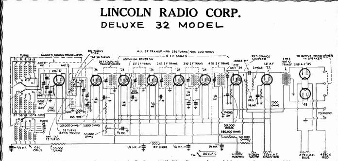
Complete wiring diagram of the new Lincoln De-Luxe "All- Wave" super-het, which tunes from 15 to 550 meters at a single "twist of the wrist". The various coils used for tuning in the different wavelengths and their connections to the "ganged" control switch, are shown at the extreme left of the diagram.
