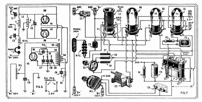
Schematic and picture diagrams are presented above, so that the uninitiated as well as the experienced short-wave fan can bulld this latest creation of Mr. Denton's-a super-regenerator receiver with balanced detector.
