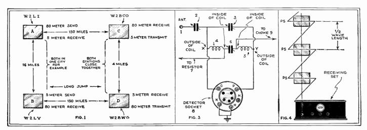
Fig. 1, at left, shows how 5-meter transmitters and receivers may be used in amatenr stations to supplement 80-meter communication; Fig. 3 shows special part of the circuit in the super-regenerative receiver which requires accurate connections; Fig. 4, at right, shows positions for resonance wave coils along the receiving antenna.
