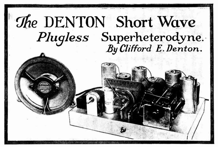
Here is the complete super-heterodyne, with band-changing switch at right, together with midget dynamic speaker—all ready for a cabinct.
