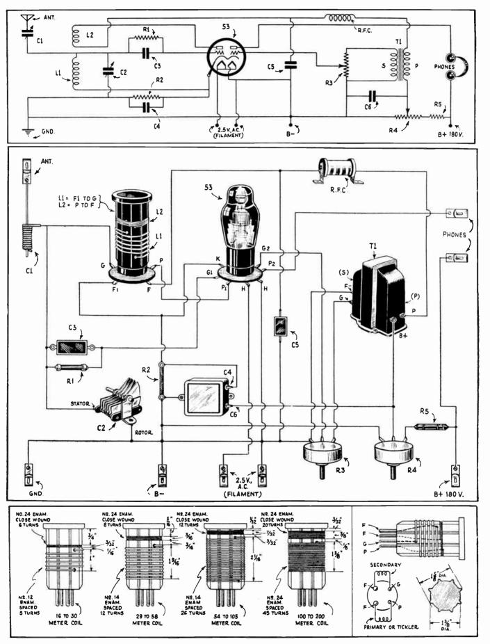
The drawings above show both the schematic and physical diagrams for the one-tube "Twinplex" receiver—in which a single 53 tube does double duty; that is, it performs both as a detector and as an A. F. amplifier—true economy! Data for winding your own coils is given in the diagram above.
