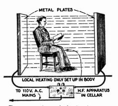
Tomorrow—instead of using furnaces we may heat "our body only" by sitting in a high frequency field. The opposite end of the "artificial fever" apparatus the engineer is holding one of the 30 meter oscillator tubes. It is a 4elementscreen-grid tube, with an output of 500 watts.
