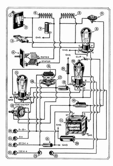
Left - Picture wiring diagram showing how ensy it is to build the 5-meter "Bearcat-3" re-ceiver. This receiver possesses high amplifying powers and good selectivity and uses but three tubes, it being possible to receive strong signals on a speaker.
