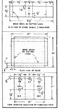
Details of aluminum chassis used by Mr. Shuart in building his 3-Tube Bandin building his 3-Spread Receiver.
