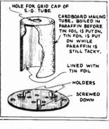
proscopie and after that a layer of tin-foil is placed around the tube while the par-affin is still tacky. A tin-foil disc is cut out for the cap and this is lapped over the tin-foil on the cylinder.—Norman Harris.
