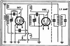
Circuit of detector and oscillator for et showing coupling coil. Denton super-het
