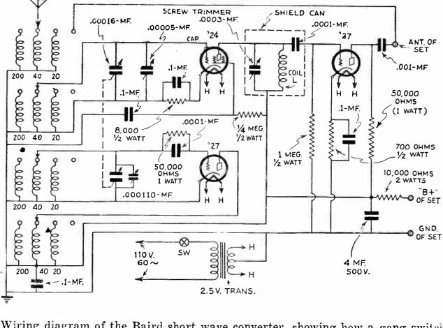
Wiring diagram of the Baird short wave converter, showing how a gang switch changes the various inductances for each change in wavelength, the range being from 19 to 200 meters.
