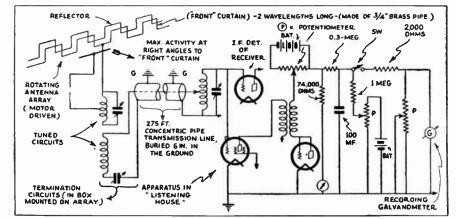
How the rotating antenna array is connected through tuned termination circuits, the short-wave signal currents then being led through a shielded cable buried in the ground to the recording amplifiers and the ink recorder itself.
