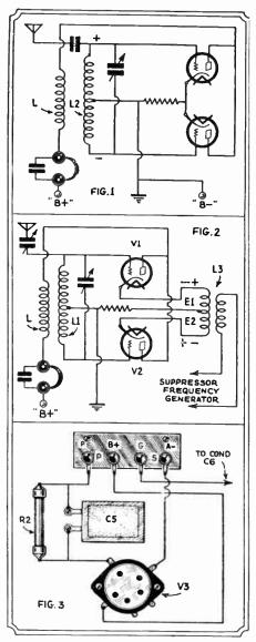
Diagrams, above, show a novel connection of balamced-detector tubes; Fig. 3 shows hook-up of apparatus to Acme 30 K.C. transformer.
