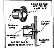
Grind or file the top of the knob fiat. Drill a hole in the center and tap it for a 6/32 or 8/33 marbine screw. Procure a disc about design drillameter (I cut mine in the center and tap it also. This disc is then fastened to the top of the knob with a machine screw just long enough to go through the end of the brass bushing and still clear the end of the shaft. This arrangement makes a ship-shape pleasure.—R. E. Lauth.
