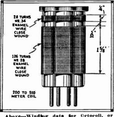
Above—Winding data for Octocoil, or similar shaped form, having sufficient inductance to cover the brondcast band with .00015-mf. condenser.
