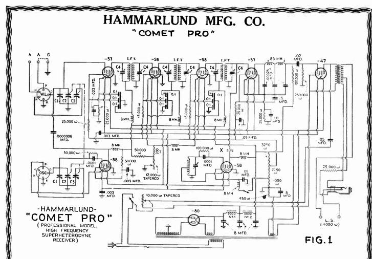
An intermediate frequency of 465 kc was chosen as a compromise. It is below the broadcast band, and at the same time is high enough to provide a large spread between a desired signal and its "image" interference. By using Litz wound intermediate coils the selectivity and sensitivity are kept high.
