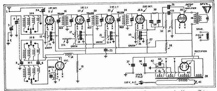
Here is the schematic diagram of the plugless S.W. super-het, in which two J.F. stages are used, with an oscillator, first and second detectors, and pentode power output stage.
