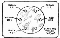
Diagram above shows the connections of detector and oscillator coils to 6-pin forms, and lower diagram shows the line-up of battery cable plug terminals. 120 TO 300 METERS-Detector
