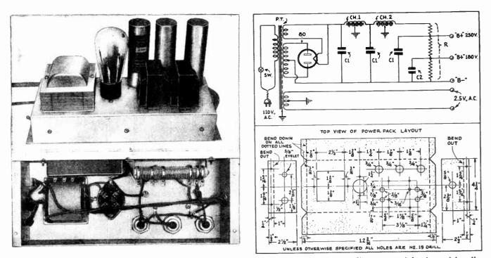
The two photos at left show the plate supply unit from the side and from the bottom. The diagrams at right show wiring dia-gram for the plate supply unit and lay-out of the metal subpanel.
