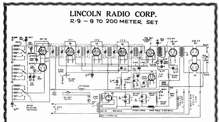
Diagram of the new Lincoln R-9 Superheterodyne, especially designed for reception in the short-wave spectrum from 9 to 200 meters. Switches select the proper coils for each band.
