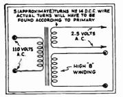
I was recently building a 4-tube A.C. receiver, but I lacked a filament transformer. I solved ny problem by removing the power transformer from my power supply and winding five turns of No. 12 D.C.C. cooper wire over the high voltage "B" winding. This gave me enough amperage to supply four 2½ yolt tubes. This method can be utilized for different voltages by yarying the number of turns-Renaldo Karas.
