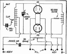
The diagram above shows the hook-up of the exceptionally few parts required in constructing the "RT" Beginner's Trans-mitter, which was especially designed by Mr. Shuart so as to embody the simplest possible construction at the lowest cost, without sacrificing quality and efficiency.
