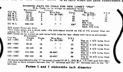
adjusted the entire spread band will be above that frequency. Conversely, setting the band with the main dial at 100 will throw the spread band on the lower frequency side. The dials on the two tank condensers are finely and accurately calibrated to facilitate precise logging. While calibration curves are furnishel with each receiver, the operator should make an accurate calibration of his own receiver by means of standard frequency signals, certain stations known to be well controlled, etc.
