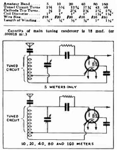
Note the difference in the funed circuits for 5 meters and above.
