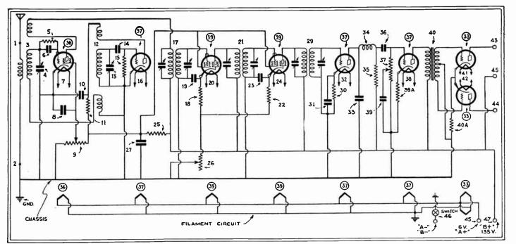
Six-volt automobile tube wiring diagram for Mr. Denton's S-Tube Portable "All-Wave" Superheterodyne receiver.
