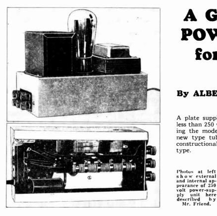
EVERY short wave experimenter needs a good cheap power supply of small size. I have designed one which can be easily constructed for less than five dollars. It will give 250 volts of pure D.C. at a current drain of 50 milliamperes (more current at a lower voltage) as well as 2.5 volts A.C. at 5.0 amperes. The overall dimensions are only 81/2 x 51/4 x 51/4 inches (with-
