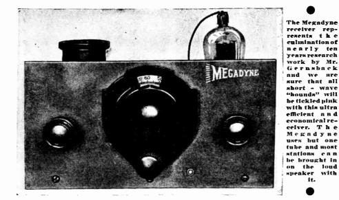
RECENTLY, after quite a good deal of experimenting, which covered a term of several months, I devised a new circuit which is termed the "Megadyne" circuit. (Megas, the Greek for "great"; dyne, Greek for "power.") The circuit originally was devised by the author for the broadcast band, and is unique in that it is actually possible to operate a loud
