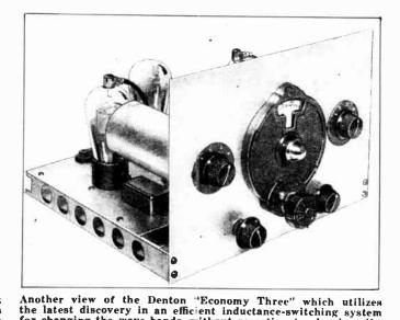
Here's a 3-tube short-wave receiver that you will derive a lot of pleasure from—it is up to the minute, with all controls mounted on the front panel, while switches change the wave bands.
