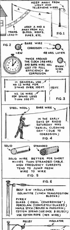
resistance to these minute R.F. currents and within 48 hours the corrosion will be so far advanced as to lower the efficiency of the antenna.
