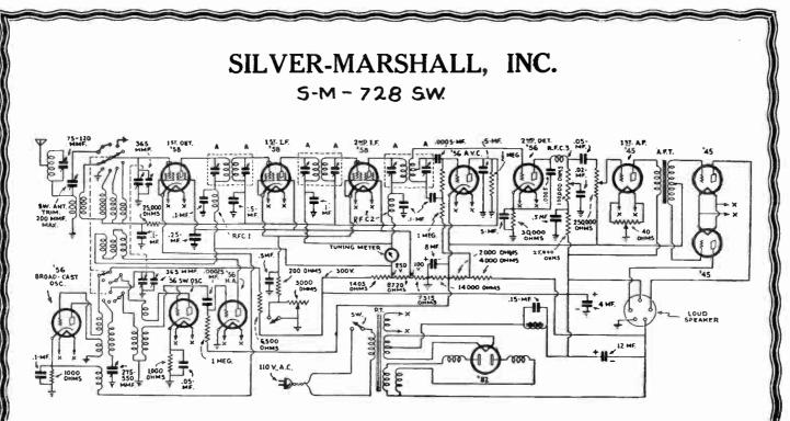
Wiring diagram of the new 728 S-W Silver-Marshall, 13 to 550 meter, 12-tube superheterodyne. Capacity A-75-120 mmf., R.F. chokes have a value of 7 millikenries.
