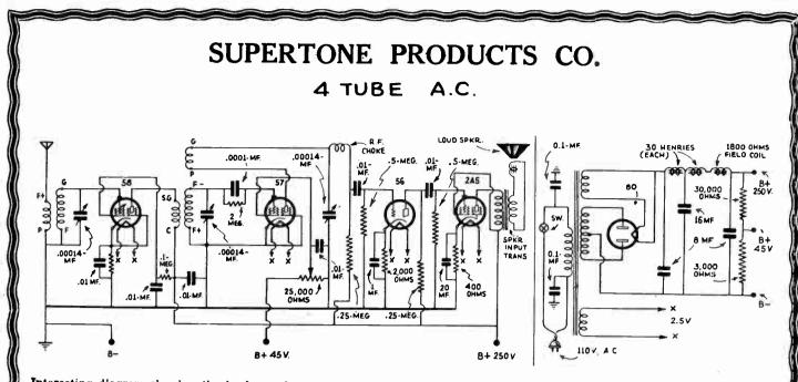
Interesting diagram showing the hook-up of the Supertone 4-Tube A.C. operated short-wave receiver, utilizing the new 2A5 output tube; also connections of power supply unit.
