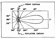
Chart above shows direction of maximum reception with respect to plane of antenna array used by Dr. Jansky.
