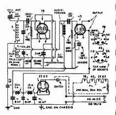
Wiring diagram of the new "Alan" Short-Wave Feceiver—it employs plug-in coils to change the wave bands. The tubes are operated in series with a small resistance across the line.
