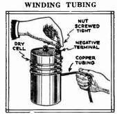
Wind your copper tubing coils on an old dry-cell. First flatten the end of copper tubing, drill a hole through it and allp over binding post. Wind the required turns while the other end is pulled tight in a vise or held by someone.—Floyd Gribben.
