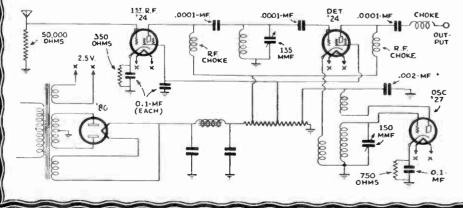
The Model 4X super-converter here illustrated was designed by Mr. George W. Walker, who has carried on a tremendous amount of experimenting and research on converters of every description; if anyone knows how to design and build a converter it is Mr. Walker. The converter here shown employs four tubes -2-'24 screen grid, 1-'27, and 1-'80 tubes. The wavelength range covered is 14 to 200 meters; the popular band from 23 to 50 meters is tuned without changing the coils.
