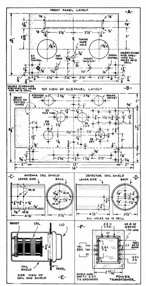
Details of chassis and other parts used in building the "Master Composite" Receiver.
