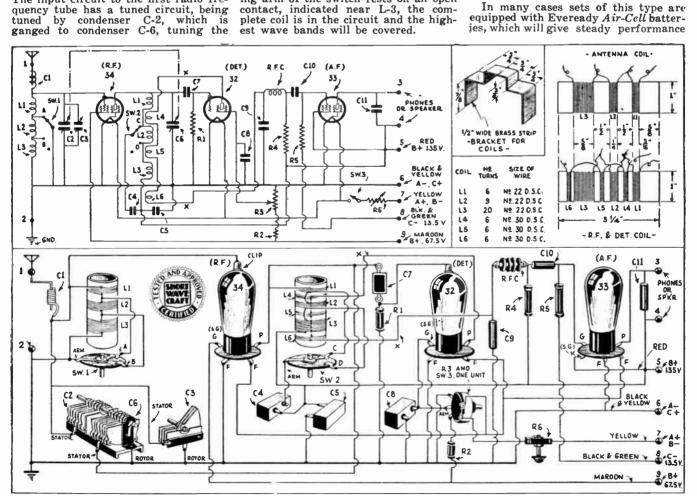
Both schematic and picturized wiring diagrams are shown above for those interested in building the Denton "Economy Three" This set employs three battery tubes and switch-type inductances instead of plug-in coils, to cover the most used bands, the 20, 40, and 80 meter bands.
