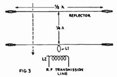
Fig. 3-The Directive Antenna System.
