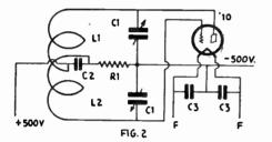
Fig. 2-The Colpitts Transmitter. C1—Two section transmitting condenser, 25-m.m.f., each section.
