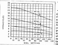
Tuning curves showing the bands covered by each of the plug-in coils.
