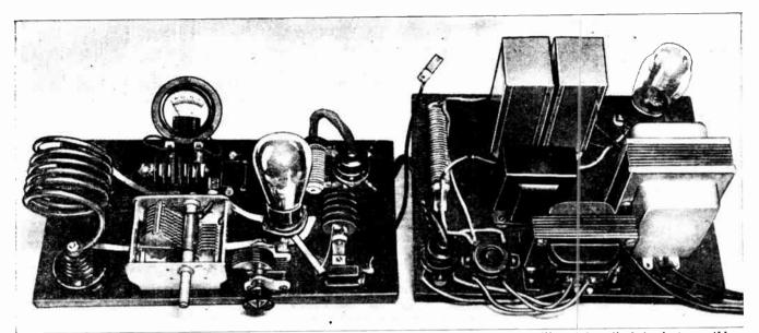
The neutralized amplifier and power-pack for use in conjunction with the Master Oscillator described in last month's article by Mr. Victor. This power amplifier uses a 46 tubr and requires no external biasing battery.
