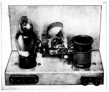
Yep! Only one tube to buy, a 6A7 or a 2A7 pentagrid-converter, plus a little simple wiring, and you have a sensitive receiver which has an output equivalent to "two" tubes---thanks to the reflexing. tubes-
