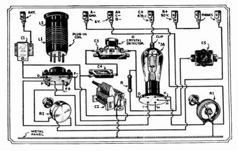
any changes in the wiring, if necessary, for experimental work. A metal panel  $8 \times 4\frac{1}{4}$  inches, mounted on a half-inch baseboard  $8 \times 6$  inches, forms the framework of the chassis. The use of a metal panel is recommended, as it eliminates hand capacity.
