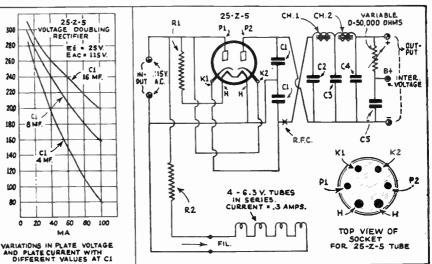
The graphs shown above, at left, tell the story of the variation in size of condensers used in conjunction with the 25-Z-5 rectifier. Wiring diagram for the complete rectifier is shown at the right. O-50,000 ohm resistor is R3.
