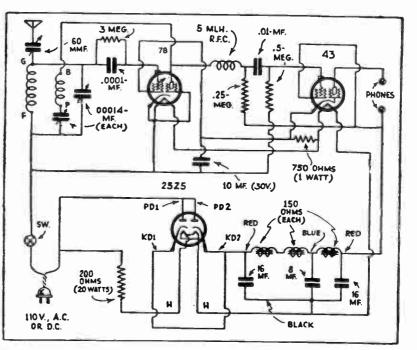
Simple wiring diagram used in the 110-volt A.C.-D.C. portable The plate current is rectified by a 25Z5 tube. illustrated above. The whole outfit is very light.
