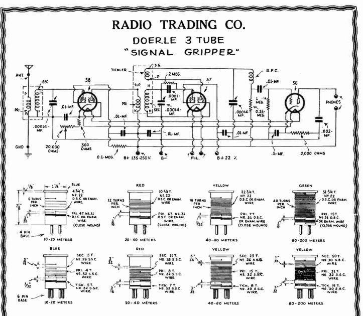
The old system of coupling between the R.F. stage and the detector, which is tuned impedance, is done away with and inductive coupling is used. The coils for this arrangement were obtained from the Radio Trading Co., and have three windings, one for the grid, one for the tickler, and a winding in-ter-woven with the grid coil for the plate circuit of the R.F. tube. Four of these coils will be needed and it is cheaper to buy them than to wind them by hand, because this is quite a difficult task.
