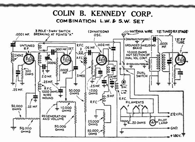
The receiver is not of the superheterodyne type, but uses a dynatron oscillator, the output being taken from the screen of this tube through a con-denser as shown. The frequency of the oscillator is fixed at approximately 1530 K.C., but can be varied.
