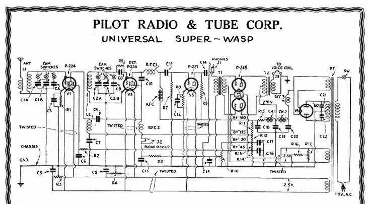
Schematic diagram of new "Universal Super-Wasp", the four only to tune the highest waveband, above 470 meters.
