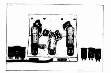
A glance at the diagram herewith shows that a tuned stage of radio frequency amplification, employing a 58 tube, is used to build up the signal strength before it is detected. Next we come to the tuned three coil coupler which links the R.F. stage with the regenerative detector, employing a 57 tube. Dual regeneration control is provided through the medium of the
