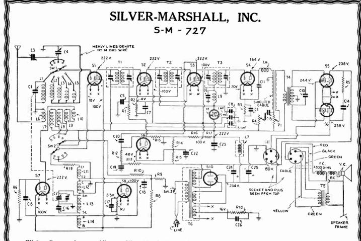
Wiring diagram for new All-wave Silver-Marshall Super-heterodyne designed for operation on 110 volt, 60 cycle A.C. circuit.
