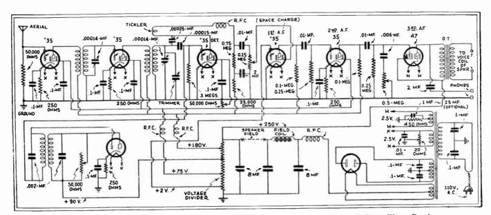
Schematic diagram showing how to wire Mr. Grater's Improved Super-Regenerative Short-Wave Receiver
