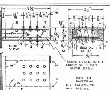
sketch of a *band switch* I have designed and which has worked in a very satisfactory manner.
