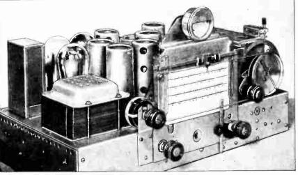
"Close-up" of the 10-tube multi-wave superhet chassis.
