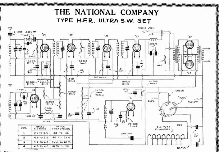
Diagram of connections used in the National 9-tube superheterodyne for ultra-short-wave reception, covering 4 to 7½ meters or 75 to 40 megacycles.
