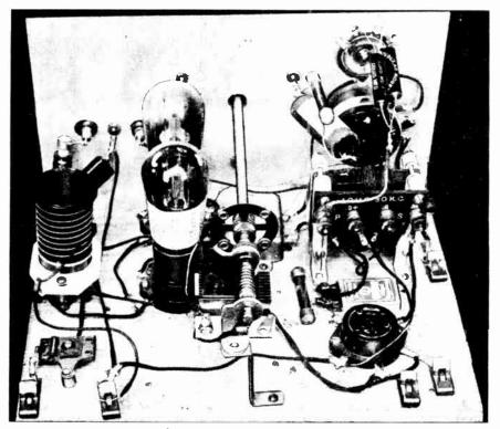
Rear view of Mr. Denton's latest short-wave receiver—the balanced-detector saperregenerator; the third tube has been left out of the socket at the right for clarity.
