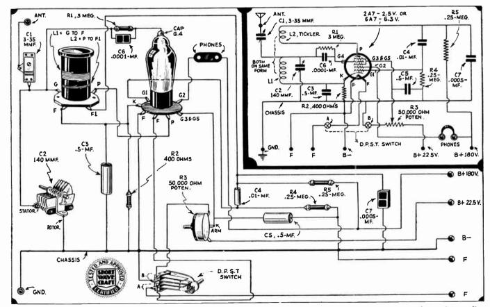
be does all the work—either a 6A7 or a 2A7, plus the really few and inexpensive parts shown in the above picture dia-Anyone can build this "one-tuber," which really gives the same output as a "2-tube receiver," due to the reflex circuit used, as verified by Mr. Shuart, well known to our readers. One tube does all the work
