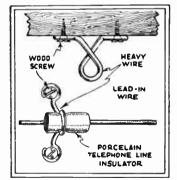
A good aerial system must have a good insulation system. The lead-in must be kept away from the sides of buildings at all times. A good "stand-off" insulator multar made prorelation insulator knobs, Take some heavy wire and make one turn around the grooved part of the insulator; then spread the legs apart and fasten to the sides of the building with wood screws, 'The lead-in may be then run through the hole. This provides a sturdy and interpensive insulator for the short-ware set.—Y. H. Mort.
