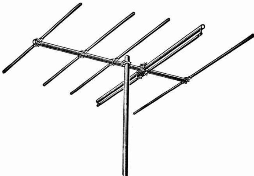
Fig. 9-15.—A five-element Yagi antenna.
