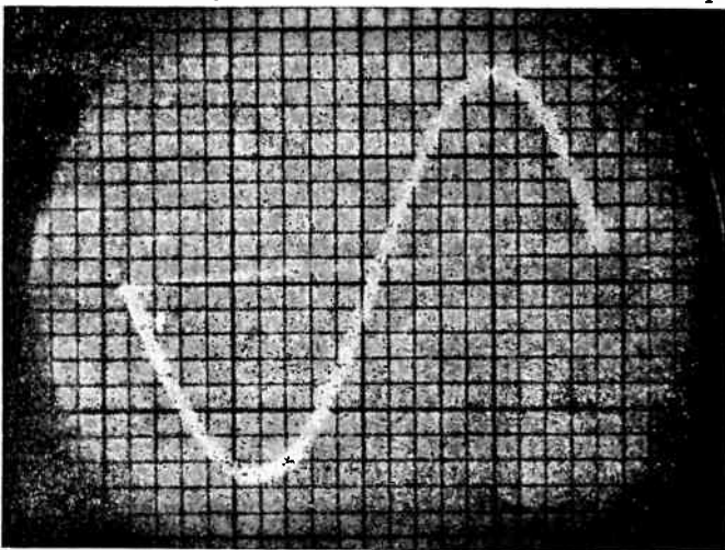
Fig. 99-12.—This graph sheet allows convenient measurement of trace heights.
