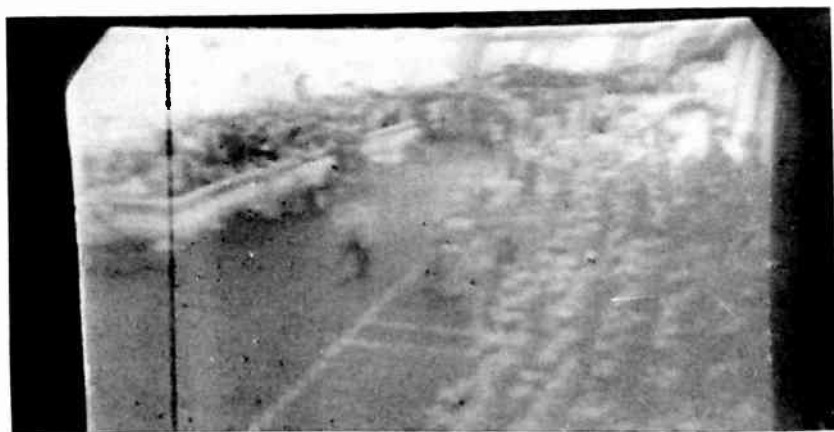
Fig. 88-2.—Barkhausen oscillation causes a dark vertical line at the left on the picture tube screen.
