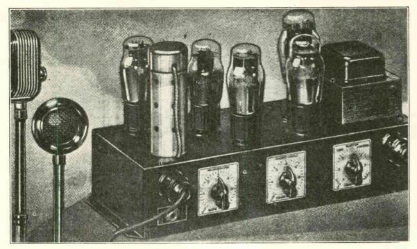
Fig. 227. Photograph of a compact public address amplifier unit. Note the separate controls for microphone, phonograph and radio signal input and also the master tone control. Thousands of P.A. units of this type are now being used in sound trucks, schools, churches, offices, auditoriums, and factories throughout the country. Courtesy Montgomery-Ward Company.
