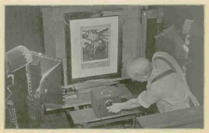
A Totalux being used to intigrate light intensity with time, in reference to exposure in photography.
