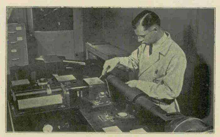
A recording spectrophotometer, a high precision instrument widely used in the paper, textile, chemical and paint industries for analyzing quality and color of product.
