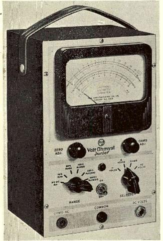
Fig. 150. This instrument checks resistor values with high frequency.
