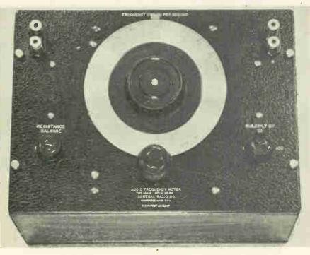
Portable laboratory frequency meter-20 to 20,000 cycles.
