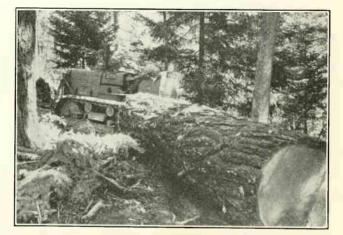
z. 25. This photo shows a Diesel-tractor used for dragging out logs in the lumber woods. (Courtesy of the International Harvester Company.)
