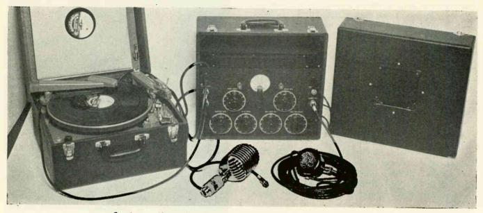
Complete portable recording system-designed to make transcriptions at any location.
