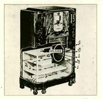
Fig. 135. Console Radio Cabinet equipped with extra built-in baffle boards to increase the distance between the back and the front of the speaker. Courtesy Stromberg Carlson Co.)
