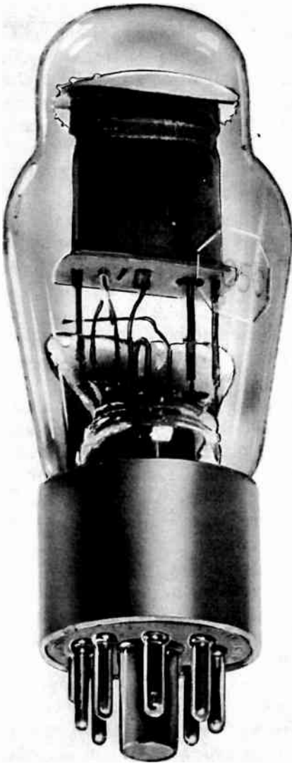
Fig. 1.—A gas-filled tetrode tube used for control purposes.
