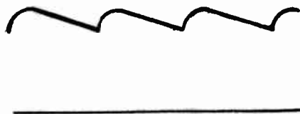
(C) Wave Form of Filter Output
