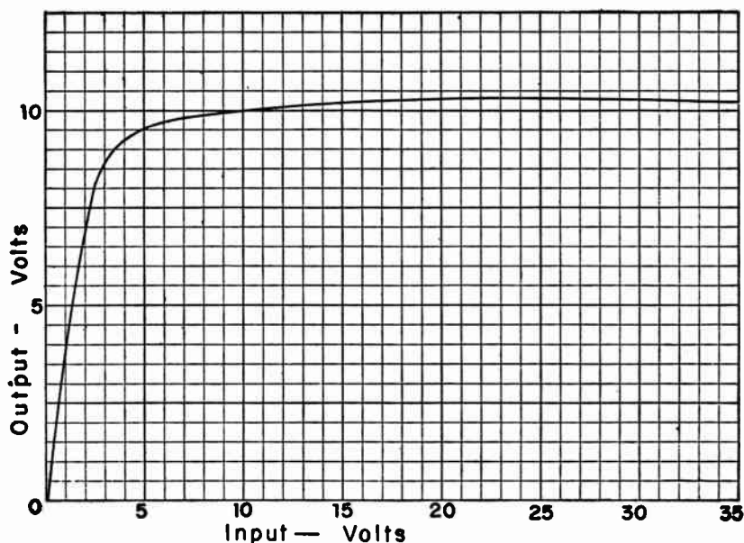
Fig. 4.—Input and output voltage relations for a typical limiter stage.
