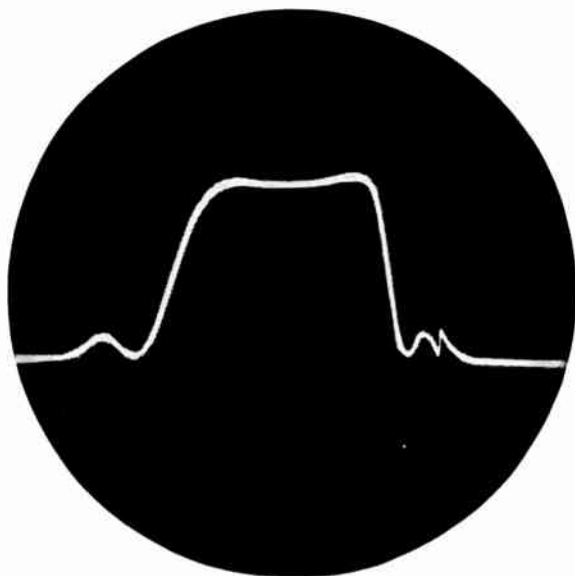
Fig. 1-8.—This response would be normal for a certain type of video i-f amplifier, from mixer to video detector.
