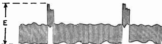
Fig. 8-15.—Height of the picture and sync signal will vary during oscillator adjustment.
