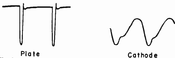
Fig. 14-20.—Oscilloscope traces taken from a diode damper tube.
