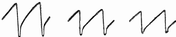
Fig. 14-16.—Oscilloscope traces showing the effect of adjusting a drive capacitor when there is feedback for production of negative pulses.
