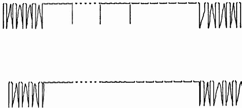
Fig. 1-12.—This is the portion of the television signal which produces pictures.
