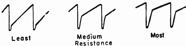
Fig. 14-11.—Oscilloscope traces showing the effects of varying the resistance in a drive control.
