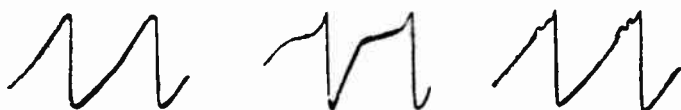
Fig. 14-14.—Oscilloscope traces from the grid of an output amplifier with which is used a capacitor drive control.
