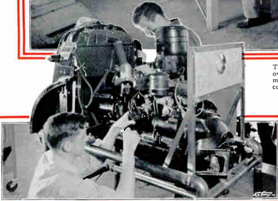
Students, adjusting and checking ignition on late model Plymouth engine. This sort of practical training helps to prepare Coyne Students to understand coils, distributors, wiring or timing on many types of engines.
