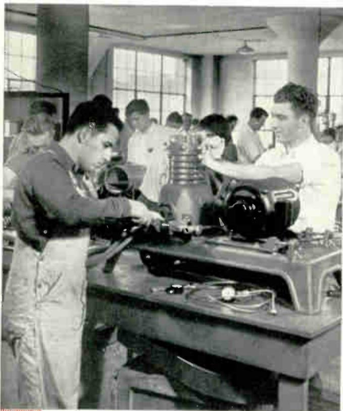
Coyne students assembling and checking a modern commercial refrigeration compressor for an ice cream machine.
