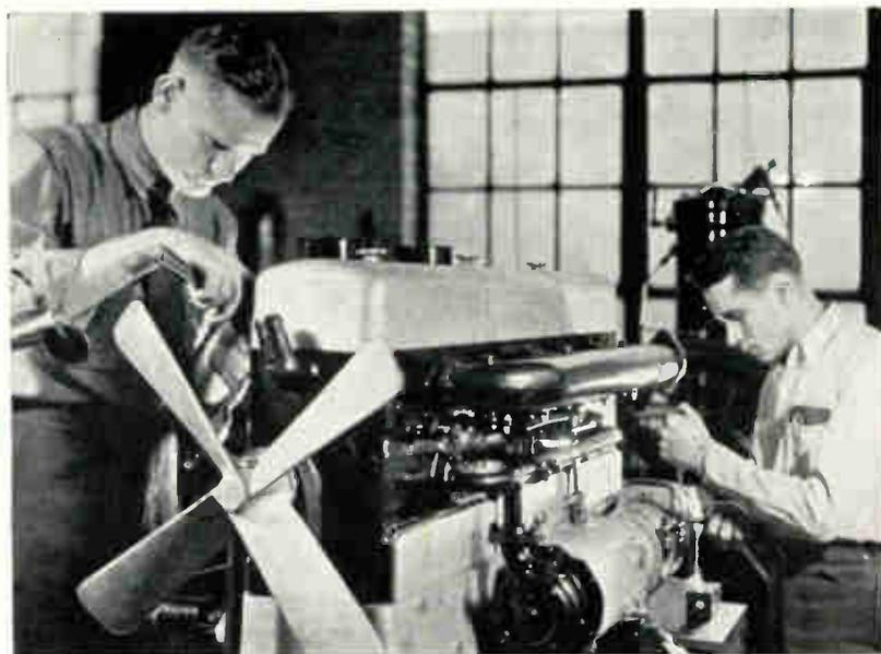
Electric starters and electric "hot plugs" form an important part of Coyne instruction in Diesel Engines. This view shows two students working on a Deutz Engine.
