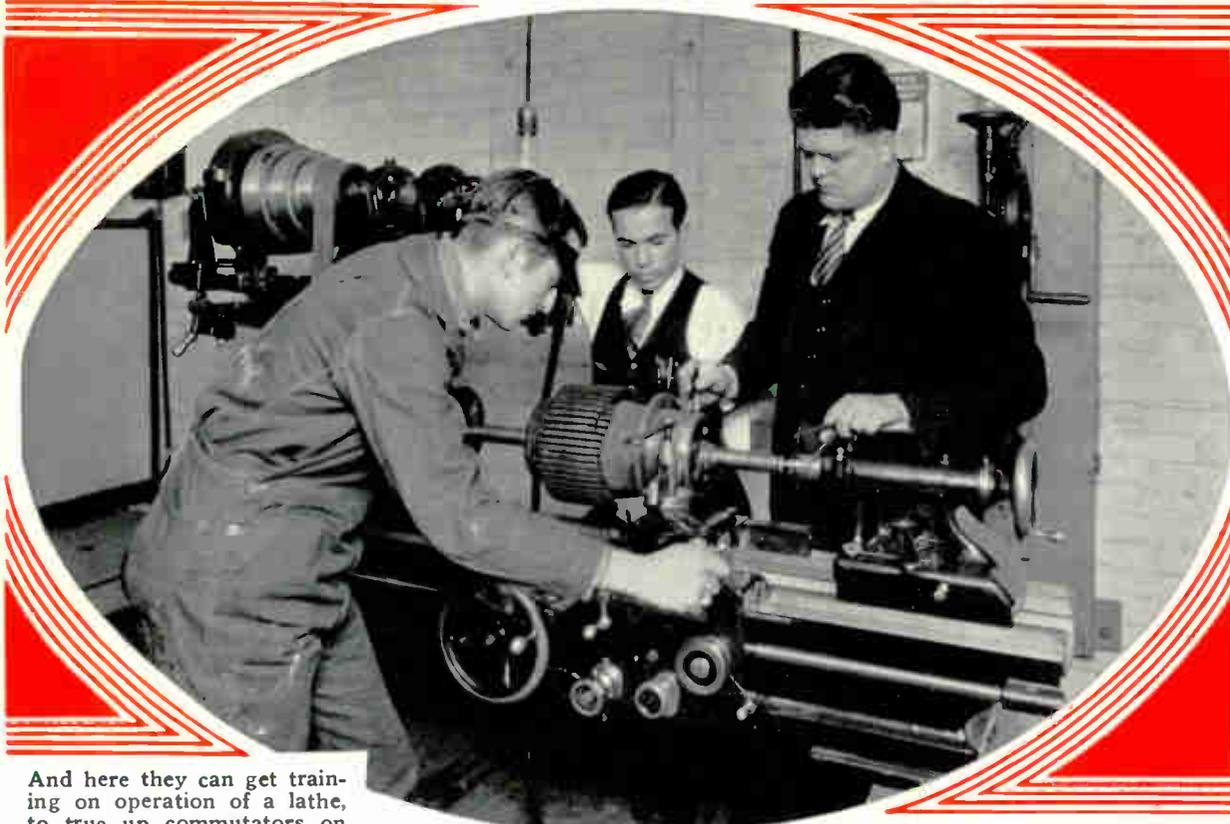
And here they can get training on operation of a lathe, to true up commutators on armatures. The instructor shows them how to grind and set the cutting tool, and how to make a nice smooth cut on the copper.
