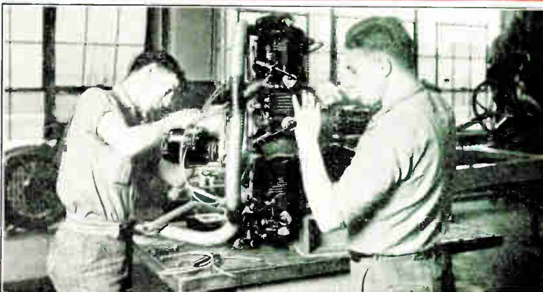
Students in our Aircraft Ignition section assembling and wiring ignition equipment and adjusting magnetos on a radial aircraft engine.
