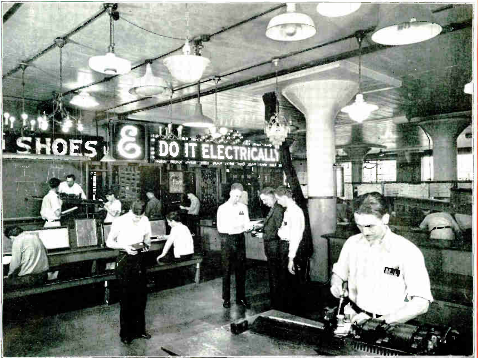
Here you see part of the illumination section, and some of the different kinds of light fixtures you work with. The instructor is showing students how to test the amount of light from each fixture with a "foot-candle meter." You are taught which type of fixture is best for home, office, or factory use.
