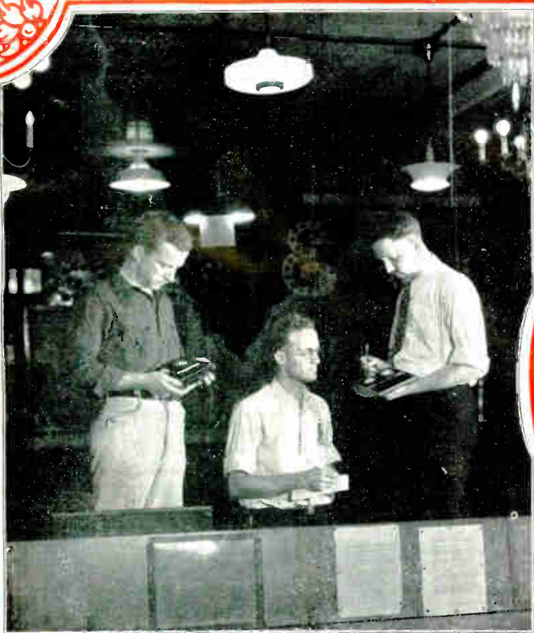
These students are making practical tests on various lighting fixtures with foot-candle meters and light meters. Their instructor is giving them a personal explanation of one of the modern type photocell foot-candle meters. This is the kind of training that makes our graduates real practical men.
