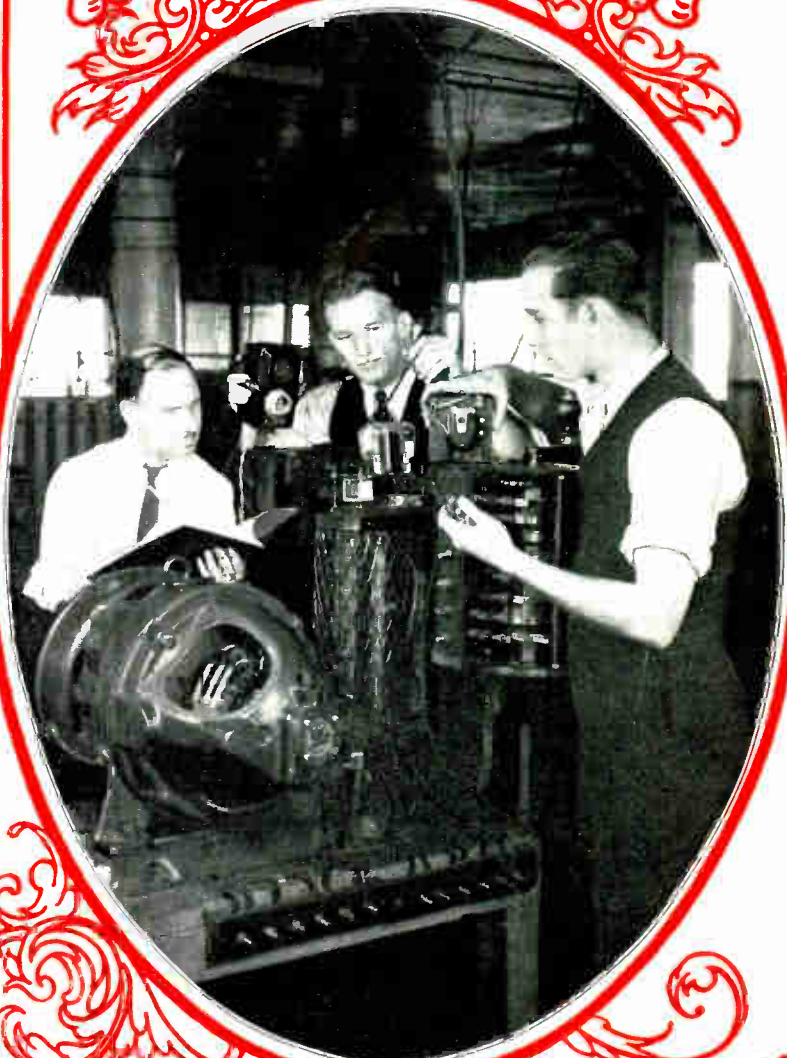
Here you see some students working on a synchronous converter, and making some very interesting connections and tests, under the supervision of the instructor on the right. These machines are used to change Alternating Current to Direct Current. It's the actual work on such equipment that gives Coyne graduates ability and confidence, in their work.
