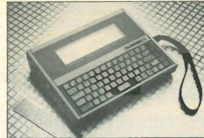
Display is through an eight line, 40-character liquid crystal which can be used for graphics. The screen memory allows for an 80-character by 24-line screen and the l.c.d. acts as a window on this larger virtual screen.
