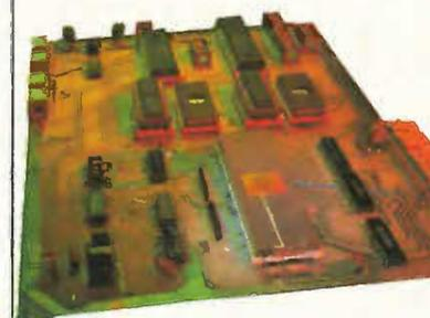
Kaycomp is a low cost computer board using a Motorola 68000 microprocessor with 16-bit data bus. It is designed for use either as an evaluation/educational tool or as the processor board of a larger system, connecting to a wide range of readily available peripheral cards through its G64 bus. This second article describes the circuit.
