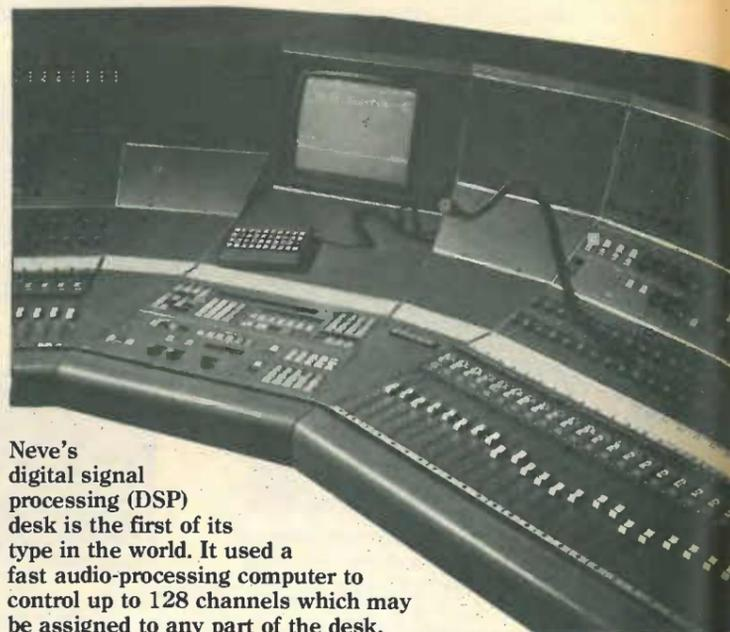
Neve's digital signal processing (DSP) desk is the first of its type in the world. It used a fast audio-processing computer to control up to 128 channels which may be assigned to any part of the desk.
