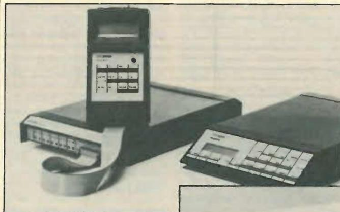
Built-in test facilities and software control are becoming increasingly common. The Hyacinth modem from Telindus has a front-panel l.c.d. screen and a membrane keyboard for entering set-up commands; a password is needed to alter them.
