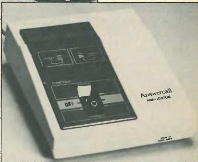
A simple 300 bit/s V.21 modem is still sufficient for many purposes: this direct-connect model is by Answercall.
