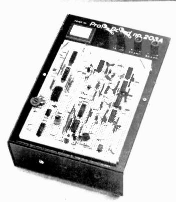
PROTO BOARDS Models PB 205, PB 203A and PB 203AK offer a large breadboarding area and a built in regulated power supply housed in a rugged metal cabinet. Models PB6 to PB105 offer various breadboarding areas screw mounted onto sturdy back plates with non-slip, non-scratch vinyl feet. Red and black binding posts are included, the red being electrically insulated from the back plate, the black being electrically connected for ground.
