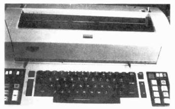
**1.** Originally from a Wang word processor system and ending up as a surplus bargain, this IBM Selectric I/O printer can be used as a letter quality printer in a computer system. Though it can be used as a keyboard as well as a standard typewriter, in this application it is strictly an output device.
