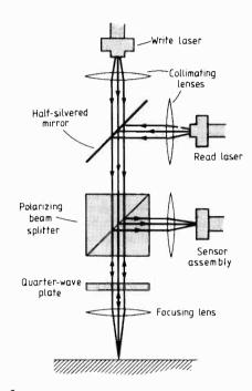
Fig. 4. Components of an optical read/write head, see text for details.
