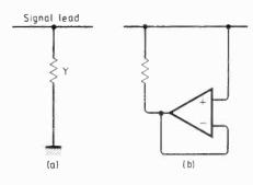
Fig. 3. The bootstrap. (a) An unwanted admittance Y shunts the signal lead. (b) The earthy end of Y is driven by the signal at unity gain. Y is still physically present, but no signal current flows through it.
