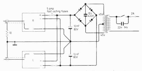
The grounding scheme is flexible in that output ground and input ground are not connected together on the board. This makes it very simple to adopt a number of wiring schemes: a proposed wiring diagram for a stereo amplifier using a common power supply is shown. Using the boards with separate supplies, output and input ground can be connected together, which gives the best signal/hum ratio in a system.
