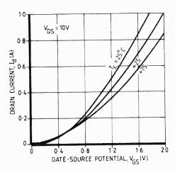
Fig. 1. Negative temperature coefficient of the drain current above 100mA prevents thermal runaway with Hitachi 2SK134/2SJ48 type mosfets and avoids use of temperature-tracking circuits.
