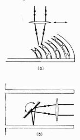
Fig. 7. Where space is no problem, fine track-following can be done by lateral lens shift (a). More compact arrangement uses a rocking mirror as shown at (b).
