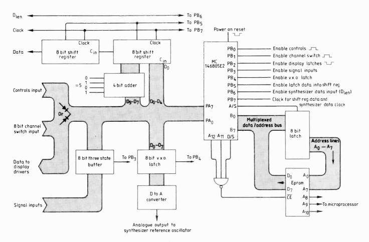
Module 8 block diagram showing the microprocessor and its interfaces. The 6805 has multiplexed address/data buses and two 8-bit peripheral-interface adapter ports. Port A is used as a bidirectional bus while port B is used to select individual peripheral input/output elements. NiCd batteries hold the processor's ram contents when the transceiver is switched off.
