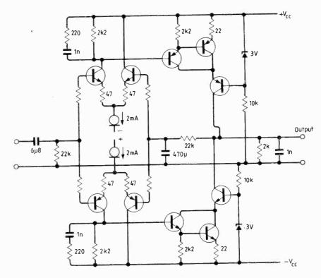
**Fig. 10.** Driver circuit chosen is as it was for open-loop measurements: gain without the load was too high: the  $2k\Omega$  load reduced it to about 66dB. In parallel with 1nF the distortion was 0.1%, both at 1 and 10kHz. Response was down 1dB at 20kHz, 2dB at 30kHz.
