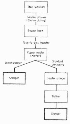
In contrast to lacquer masters, numerous matrices can be produced from a direct metal master, permitting easy correction of defects which may appear in the plating steps en route to the stamper. Process gives a significant time economy in the plating process, especially when making a stamper directly.
