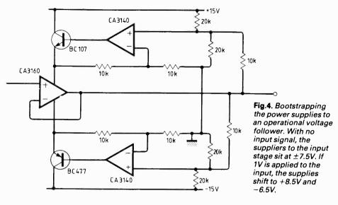
amplifier (surely one only bootstraps passive components?), but the circuit does work as advertised. Indeed, some operational amplifiers have *internal* bootstrapping of the input stage. If the signal gain from input to supply leads in Fig. 4 is adjusted to be very close to unity, improvements of several orders of magnitude in the input impedance can be obtained. Even ordinary bipolar amplifiers such as the 741 can be given an effective input resistance of many  $G\Omega$ .
