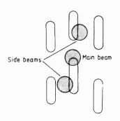
Fig. 8. Simple tracking system uses two auxiliary beams each side of the reading beam. Track misalignment causes the two side beam signals to change in amplitude differentially.
