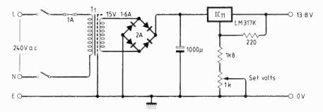
Fig. 4. Power supply, which also charges external battery.
