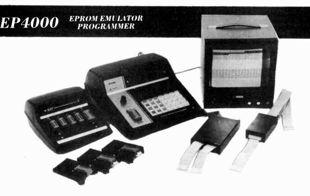
The microprocessor controlled EP4000 will emulate and program all the popular EPROMs including the 2704, 2708, 2716(3), 2508, 2758, 2516, 2716, 2532 and 2732 devices. Personality cards and hardware changes are not required as the machine configures itself for the different devices. Other devices such as bipolar PROMs and 2764 and 2564 EPROMs are programmed with external modules.
