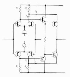
**Fig. 6.** This offers very good linearity and easy control of the second stage current,  $I_2$ .
