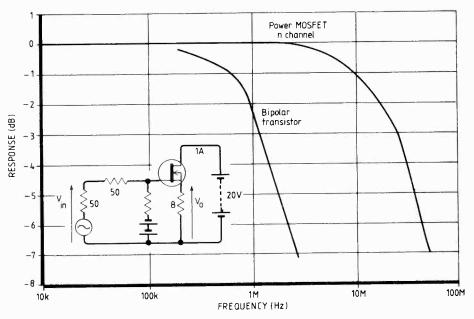
Fig. 2. This n-channel mos source follower has ten times the bandwidth of an emitter
