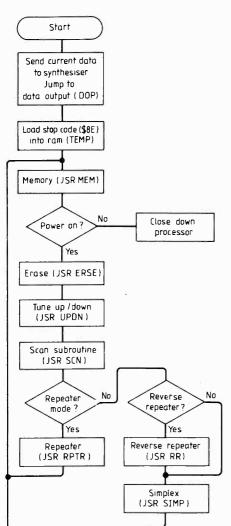
Transceiver software breaks down into these main routines. Mnenonics shown are used in the assembly-language program.
