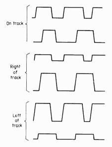
Fig. 9. A possible embedded servo technique for optical discs uses one beam for track following. Two beams spaced at 1/2 track apart could generate twophase signal to count track crossings. In the three examples shown, notice the effect of position error on the second part of the pulse waveform. (Compare with article on servo surface drives, August 1982 issue.)
