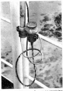
Fig. 13. Matching transformer on receiving whip greatly improves 500 khz reception.
