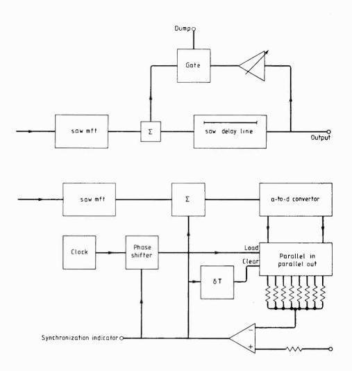
Fig. 6. Recirculation loop enhances otherwise noisy output. As data rate is fixed, section of the sequence appears after a fixed time T. The first output is delayed by T so that it reaches the input of the summer at the same time as the next output of the filter arrives. The output of the summer would go on increasing until a threshold is reached, when the gate would open and sync achieved. A t.t.l. version of the recirculation loop is shown at bottom.
