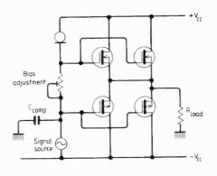
Fig. 9. Paralleling mosfets is easy, thanks to the high-input impedance and the uniform current distribution across the die.
