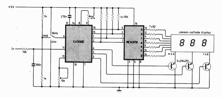
MC14511B is not able to display the "-" (minus) and the "E" (overload) characters. With negative input signals the most significant digit will be blanked, and with overrange input signals all digits will be blanked.
