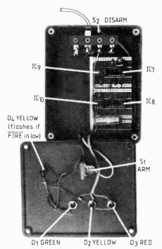
Fig. 6. Remote unit in its metal box.
