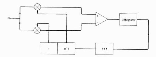
Fig. 4. A d.p.s.k. demodulator that can operate under low s/n ratio is the Costas loop, which requires accurate balancing of the two arms. Loop filter is similar to that used in phase-locked loops.
