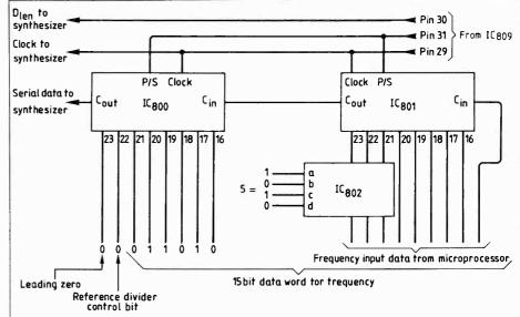
Bits for the synthesizer-control word are set on  $IC_{800,801}$  as shown. Nine least-significant bits are required for the range 135-137MHz, the remaining six are hard wired. Full adder  $IC_{802}$  produces offset required to provide nine control bits from an eight-bit processor port.
