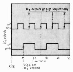
Fig. 2. Counter IC<sub>4</sub> timing diagram, showing 20s delay after FIRE input.
