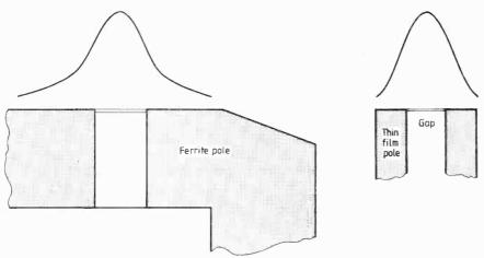
Fig. 2.Comparison of fields of ferrite (left) and thin-film heads (right). Curves show longitudinal field strength at typical working distance from poles. Sharper curve of thin-film head allows shorter wavelength recording.
