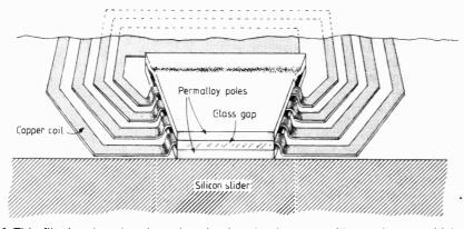
Fig. 1. Thin-film head made using microcircuit technology on a silicon substrate which becomes the slider.
