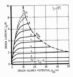
**Fig. 3.** Typical  $I_0$ - $V_{Ds}$  curves for 2SK134 show that maximum drain current is limited to seven amps.
