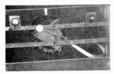
Fig. 5. Arcing from frame to switch interconnecting wire, top centre. The round objects, left and right hand sides, are neon bulbs.
