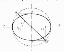
perpendiculars are erected from A and B to meet z-z, these points will meet it at  $F_1$  and  $F_2$ , their accurate distance apart=major axis  $\times$  cos "a". To find the area of the ellipse I multiply the area of the auxiliary circle by sin a.
