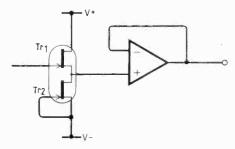
**Fig. 2**. Voltage follower using matched junction fets as input stage.
