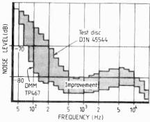
Teldec curves show that new direct metal mastering audibly reduces background noise (measured by third-octave filter). Reference level measurement corresponded to a recorded velocity of 10cm/s for one groove wall. Curve A shows the background noise of rumble test record DIN 45544, and B shows the same measurement with the DMM record TP467.
