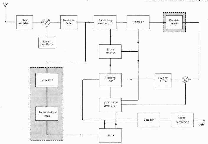
achieve code synchronization so that the local code generator can be synchronized with the received code. As soon as code synchronization is obtained, the tracking loop is switched on and decoding by correlation begins. Further description of acoustic surface-wave matched filters is given later.
