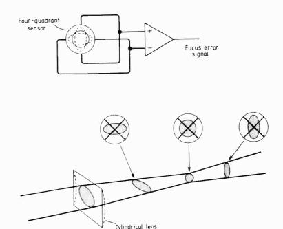
Fig. 6. Use of a cylindrical lens prevents a point focus and results in an elliptical image, circular at one point only. Horizontal ellipse causes more light to fall on left and right sensor quadrants, vertical ellipse favours upper and lower quadrants, and a differential amplifier provides focus error signal. Four quadrants are summed for read signal output.
