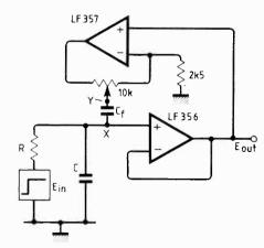
Fig. 5. Capacitance-neutralised voltage follower. R and C are the series resistance and shunt capacitance of the signal source. Signal gain at point Y is adjustable from 1 to 5. The follower stage, here shown as a 356 operational amplifier, is often constructed with bootstrapped supplies as in Fig. 4.
