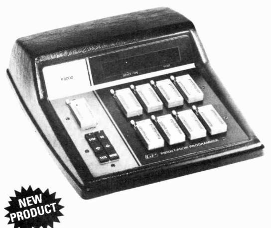
Checks, Programs, Compares up to 8 devices simultaneously
