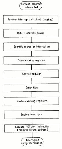
Fig. 10. Step-by-step operation of interrupt-driven systems.
