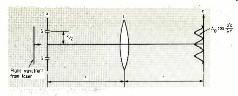
Fig. 4. Amplitude distribution in the front and back focal plane constitute a Fourier transform pair; the slits approximate impulse functions.
