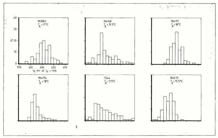
Fig. 2. Distribution of  $V_f$  (amb) for six types of silicon diode.
