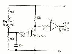
Fig. 2. Optional buffer circuit for 20mA loop input. This circuit replaces  $R_2$ ,  $R_3$ ,  $D_1$  and  $TR_1$  of Fig. 1.
