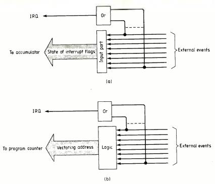
Fig. 8. (a) Non-vectored interrupts; (b) vectored interrupts.
