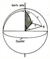
Fig. 7. For plotting range rings on the polar projection map, to aid evaluation of the antenna elevation required, angle x must be found for various latitude values using constant values of angle a. In Fig. 3, range rings are plotted for  $a=30^\circ$ ,  $a=50^\circ$ , and  $a=70^\circ$
