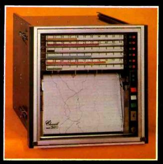
This Chessell multi-pen chart recorder uses six low-inertia DC motors for pen drive and a stepper as paper drive.
