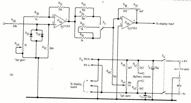
Fig. 5. Signal amplifier. Resistors  $R_{30}$  to  $R_{40}$  are of high-stability, and  $R_{41}$  is a linear, wirewound, 1W component.
