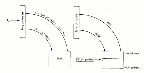
Fig. 5. How the program counter is saved and restored before and after interruptions.
