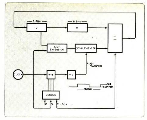
Fig. 2. Block diagram of sine-wave oscillator. Set carry for subtract mode; reset carry for add mode.
