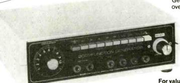
Get all the waveforms you need - 1 Hz to · 1 MHz in five overlapping ranges: stable, low-distortion sine waves, fast rise/fall-time square waves, high linearity triangle waves - even a separate TTL square wave output. Plus high- and low-level main outputs. An applied DC Voltage at the Sweep input
