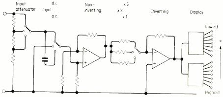
Fig. 2. Block diagram of millivoltmeter.
