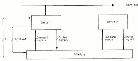
Fig. 3. Basic interrupt configuration.
