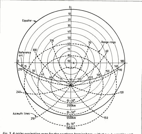
Fig. 3. A polar projection map for the northern hemisphere, with the sub-satellite path reference arc drawn in, and the azimuth lines and range rings plotted at 0° longitude, 52° latitude, i.e. London.
