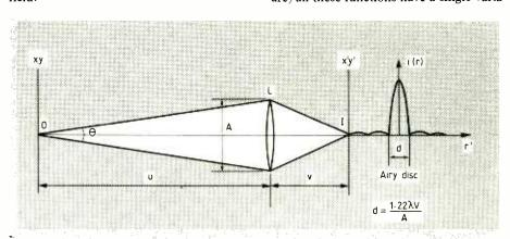
Fig. 1. Image of a point object is a circularly symmetric distribution of intensity called an Airy disc.
