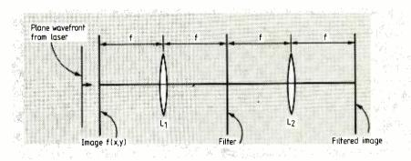
Fig. 5. Optical image processing system operates on the Fourier transform of an image by spatial filtering.
