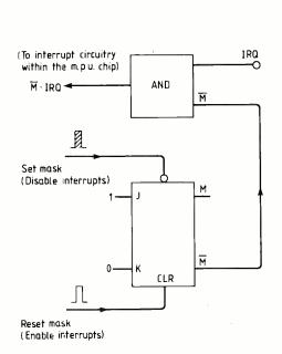
Fig. 9. Flip-flop for masking interrupts.
