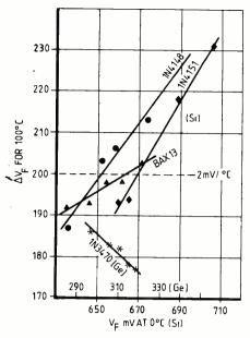
Fig. 3. Correlation between  $V_f$  (0°C) and  $\Delta V_f$ (100°C).
