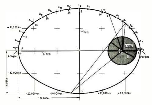
Fig. 1. The orbit ellipse. Once the ellipse has been plotted, it can be used to estimate the height of the satellite above tne earth at any point on the orbit, along with the time elapsed from either apogee or perigee to the point concerned.
