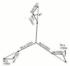
8. Vector addition of the inverter windings.
