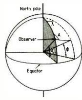
Fig. 5. Angles used in the formula for calculating azimuth lines.  $\phi_0$  is the observer's latitude and  $\lambda$  is the meridian used to calculate  $\phi$ , the latitude cut by the azimuth line.
