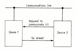
Fig. 2. Block diagram showing how communication between two devices is established using flags.
