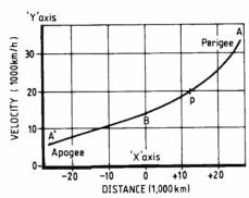
Fig. 2. This graph shows the velocity of the satellite at any point between apogee and perigee, or vice-versa, for the hypothetical orbit shown in Fig. 1. Distances shown on the graph relate to the axes of the ellipse.
