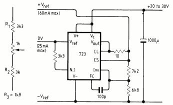
Fig. 6. Stabilized power supply. The resistor network allows adjustment of the positive rail to exactly twice V<sub>ref</sub>.
