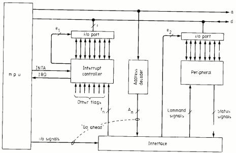
Fig. 7. Basic configuration of an interrupt system.
