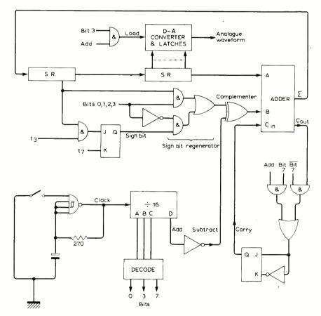
Fig. 3. Logic diagram of oscillator
