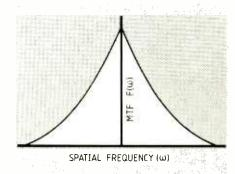
Fig. 3. High quality lenses have an m.t.f. close to that of an ideal or diffractionlimited lens.
