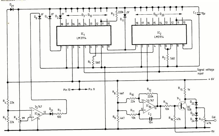
Fig. 3. Display circuit and calibration oscillator ( $IC_{3b}$  and  $Tr_1$ ).
