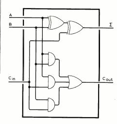
Fig. 4. Logic details of adder in Fig. 3.
