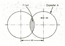
Fig. 2. Modulation transfer function of a lens may be viewed as an auto-convolution of the aperture function. Area of overlap represents magnitude of the m.t.f. at spatial frequency  $\omega$ .
