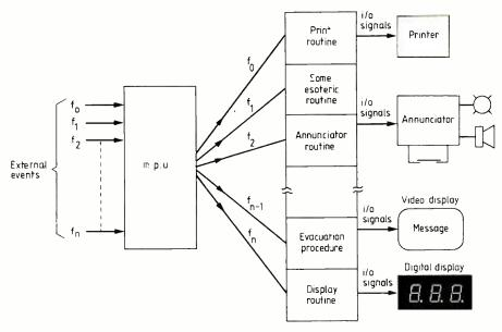
Fig. 1. Block diagram showing software response to external events — note the i/o signals.
