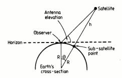
Fig. 6. The angle  $\theta$ , needed to calculate the antenna elevation angle, can be found either by plotting distances on a globe, or by plotting range rings around the observer on the polar projection map.
