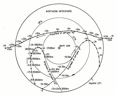
Fig. 4. Representation of the top side of a transparent overlay. These three sub-satellite paths have been plotted from the example data given in the text at three different arguments of perigee to demonstrate the method. Once a path has been plotted, it should be usable for about three months, depending on the orbit inclination and the accuracy required.
