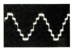
9. The combined output of six inverters.
