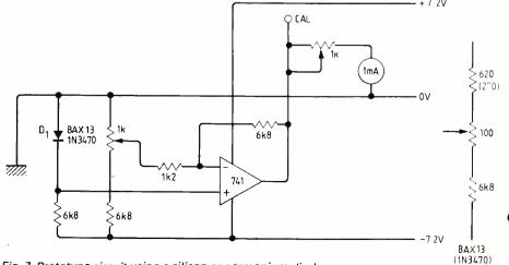
Fig. 7. Prototype circuit using a silicon or germanium diode.
