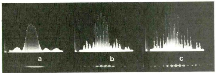
Fig 2. n-slit diffraction (a) n = 1, (b) n = 2, and (c) n = 4. The direct image is seen in the lower portion, and the intensity distribution in the upper portion of each frame.
