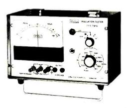
A logarithmic scale covering 6 decades is used to display either insulation resistance or leakage current at a fixed stabilised test voltage. The current available is limited to a maximum value of 3mA for safety and capacitors are automatically discharged when the instrument is switched off or to the CAL condition. The instrument operates from a 9V internal battery.
