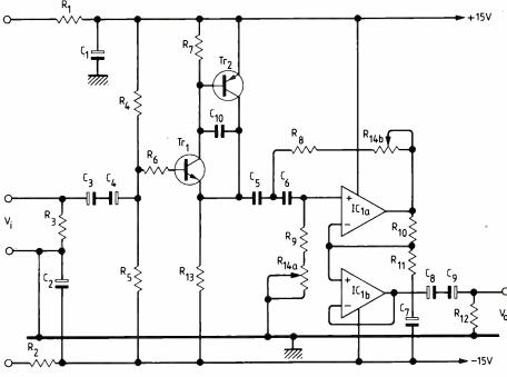
Fig. 5. Practical rumble filter, tunable from 20Hz to more than 160Hz.
