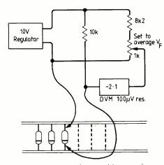
Fig. 11. Test circuit for matching sensing diodes.
