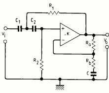
Fig. 2. Second-order, high-pass filter formed from v.c.v.s. of Fig. 1.
