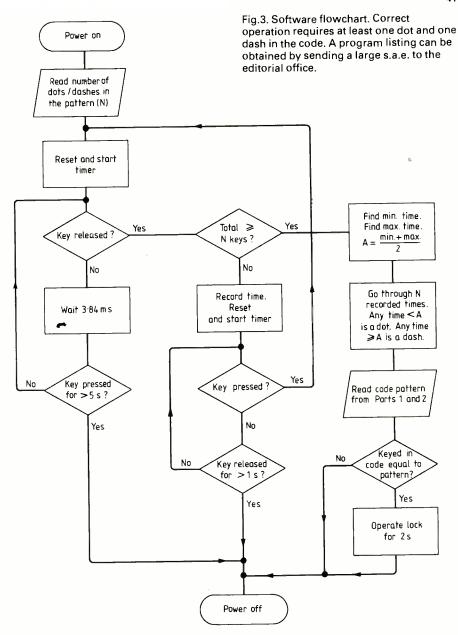
sary if a wrong code is entered because the 8478 will switch itself off after one second and the code can then be re-entered. These periods were found to be the most suitable after simulations of the Morse code input algorithm were carried out.
