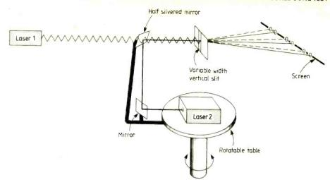
Fig 5. Schematic view of the assembly for varying the angular separation of two laser sources.
