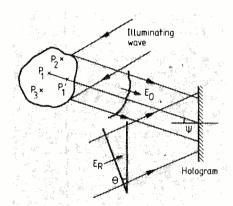
Fig. 6. Two-dimensional intensity distribution at the hologram is a combination of angle and amplitude modulation.
