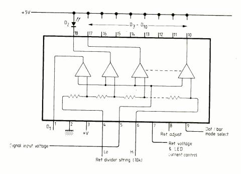
Fig. 1. Working of LM3914 dot/bar driver i.c.
