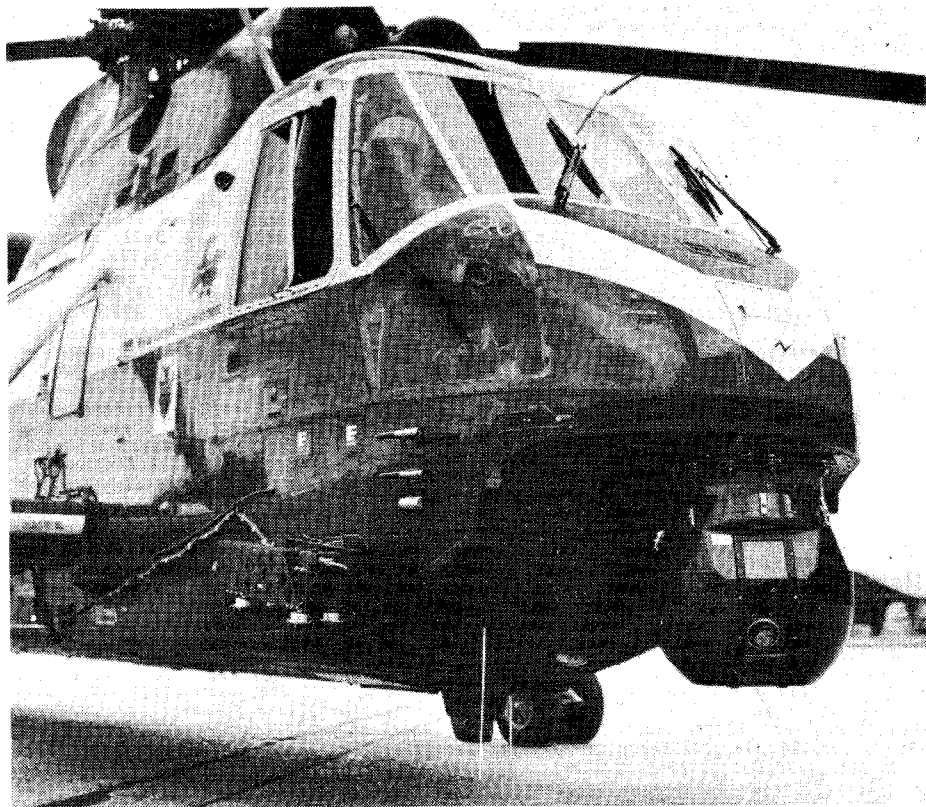
Marconi infrared camera for night vision, mounted under the nose of a Sea King helicopter. Camera aligns itself with pilot's line of sight, and display is mounted on his helmet.
