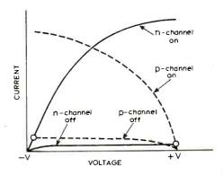
Fig. 3. Load lines of c.m.o.s. device show power dissipation to be low—says 10nW per gate—in both on and off states.
