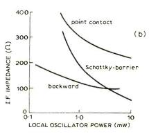
Fig. 3. Increasing oscillator power increases conversion efficiency but also the noise temperature ratio. There is an optimum power level for minimum noise figure.
