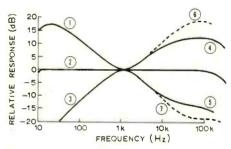
Fig. 2. Amplitude/frequency response curves of tone control circuit. 1. Bass boost max. 2. Flat response 3. Bass cut max. 4. Treble boost max. 5. Treble cut max. 6, 7. Treble boost and cut with  $R_{\gamma}$   $R_{\kappa}=1k\Omega$ .
