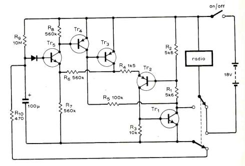
2N3706 for  $Tr_1$ ,  $Tr_5$  and 2N3702 for  $Tr_2$ ,  $Tr_3$ ,  $Tr_4$ .) The capacitor must also have low leakage and some experimentation may be necessary. Resistor  $R_{10}$  discharges the capacitor rapidly to permit another operation immediately. The switch requires a good insulation resistance.
