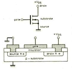
Fig. A. Insulated-gate (m.o.s.) f.e.ts that work by modulation of a conducting channel can be either a depletion type—conducting with zero bias—or an enhancement type—cut off with zero bias. Illustration shows an n-channel enhancement device.
