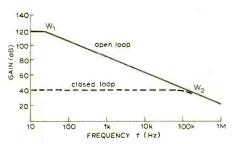
Fig. 8. Bandwidth increase with addition of feedback.
