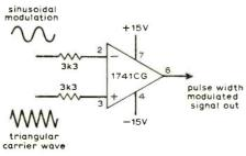
Fig. 12.1 Op-amp used for pulse width modulation.
