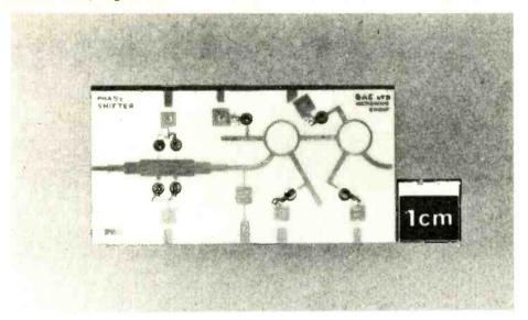
Fig. 8. Four-element phase shifter on 0.025-in alumina consisting of 22.5, 45, 90 and 180° sections which can be switched in any combination. (Thanks to my colleague J. E. Evans for this.)
