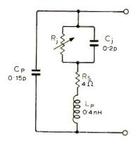
Fig. 2. Most microwave semiconductors are encapsulated and the package reactances must be taken into account when calculating the terminal impedance. Shown is a typical equivalent circuit for an X-band diode.
