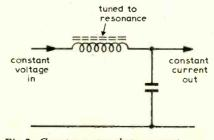
Fig.2. Gyrator network to convert constant-voltage square wave to constant-current tube drive.
