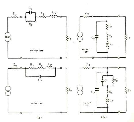
insertion loss is  $10 \log_{10} [2^2 + 2.5^2/4.5^2 + (2150) + 1] = 0.2 \text{dB}$ . With the switch off under zero bias and again neglecting  $C_p$ ,  $R_F = 10 \text{k}\Omega$  and some algebra indicates that the isolation provided is about 24dB.
