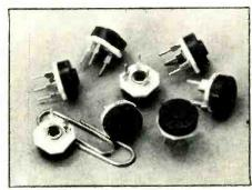
The RGP 10 is rated at 0.5W at 40°C, resolution is infinite, and the temperature coefficient is  $\pm$  250p.p.m./°C. Resistance range is  $100~\Omega$  to  $1M~\Omega$ . Featuring an integral dust cover, the device also offers standard 0.1in grid pin spacing which, with its low price and technical specification, makes the RGP 10 a practical alternative to carbon devices. Industrial Electronic Components Division, Guest International Ltd., Redlands, Coulsdon, Surrey, CR3 2HT.
