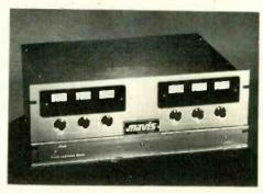
speech amplifying systems. It enables the bass range, mid-range and trable range to be separately controlled. The cross-over frequency for each range can be specified if required but will be, in the standard unit, as follows:
