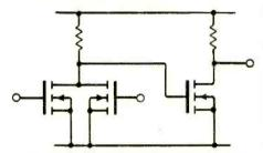
Fig. B. Linear or logical functions can be performed by this simple p-channel i.g.f.e.t. circuit, which can be directly-coupled provided the supply is greater than the threshold voltage.
