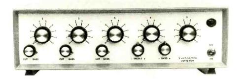
This is a high fidelity amplifier with bass cut controls on each of the three low impedance balanced line microphone stages and a high impedance (1.5 meg.) gram stage with bass and treble controls, plus the usual line or tape input. All the input stages are protected against overload by back to back low self capacity diodes and all use F.E.Ts for low noise, low intermodulation distortion and freedom from radio breakthrough.
