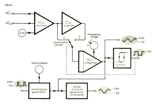
Fig. 3. Oscillator VCO, in block diagram form.
