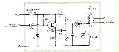
an air-cored transformer which provides ample power-frequency isolation. At the hi-fi system, the resulting f.m. signal can be capacitatively coupled into the aerial circuit of an f.m. radio. By suitable
