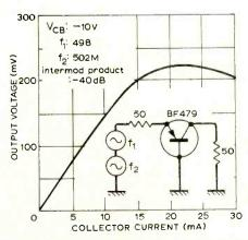
Fig. 2. Linearity of gain up to 15mA or so of BF479 improves cross-modulation performance, the gain control function being taken over by p-i-n diodes.
