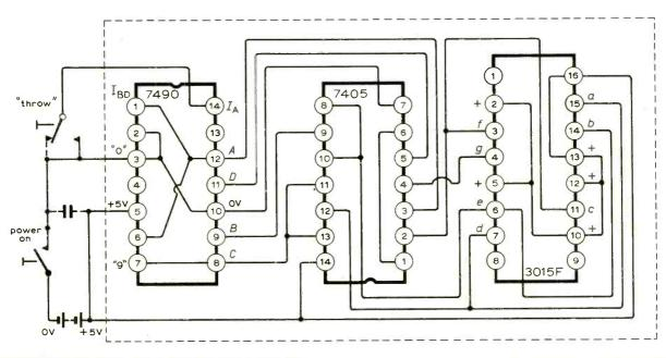
Fig.2. The layout of the circuit, seen from the component side.
