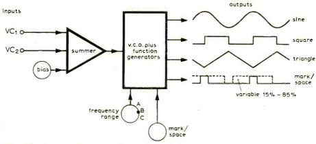
Fig. 2. Functions of voltage controlled oscillator, VCO,
