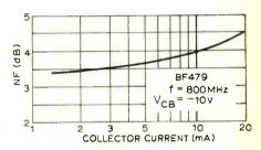
Fig. 3. Lower and more constant noise figure versus temperature and current are features of the BF479 transistor.
