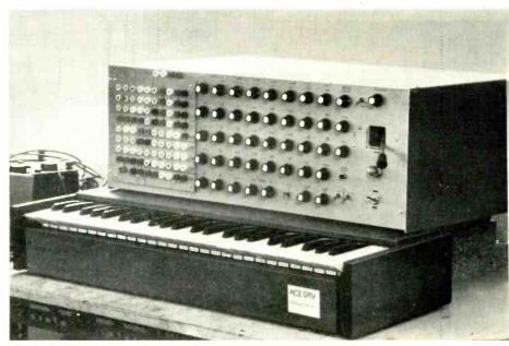
Manual control of the synthesizer's functions is provided by a control panel, joy-stick and keyboards. The patch panel provides a means, together with voltage summing networks, of linking the internal functions.
