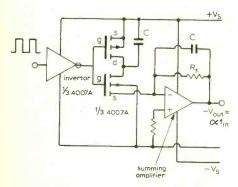
Fig. 15. This precision frequency-to-voltage converter is cheaper using c.m.o.s. package than with discrete i.g.f.e.ts.
