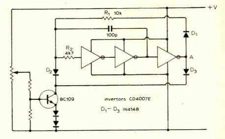
approach an equilibrium under the influence of the d.c. feedback the system switches to hard off when the loop gain round the first two invertors reaches unity. The feedback resistor then causes a current from point A to point D into the capacitor to move back toward the equilibrium. This results in a further regenerative switching edge in the reverse direction.
