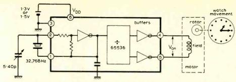
Fig. 9. Electronic watch system features both linear and switching operation of c.m.o.s. This circuit will operate from a 1.3V cell at  $6\mu W$ .
