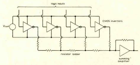
Fig. 10. Technique of digital-to-analogue conversion in which a resistive ladder is switched to generate a linear signal from a digital code.
