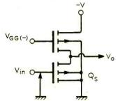
Fig. C. Many m.o.s. circuits have the resistive loads replaced by transistors, as in this p-m.o.s. inverter.
