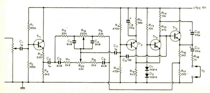
Fig. 1. Circuit diagram of tone control. Transistors  $Tr_1$ ,  $Tr_3$ ,  $Tr_4 = BC109$ , BC114, BC184.  $Tr_2 = BC15$ , BC214, BC309 etc.
