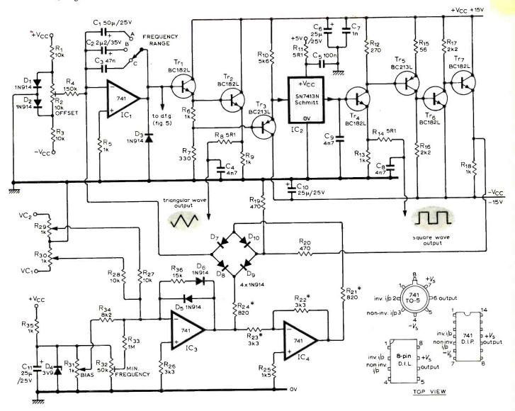
Fig. 4. Circuit of VCO<sub>1</sub>. All resistors are 5%, & W unless asterisked — these are 2%.
