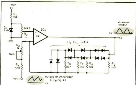
Fig. 5. Diode function generator which produces a sinewave output when fed with the triangular wave output from the integrator  $IC_1$  in Fig. 4. All resistors are  $\frac{1}{4}W$ , 5%.
