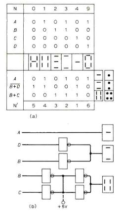
Fig.4. (a) Logic states and patterns of the pure binary die. (b) Decoding and drive circuit.
