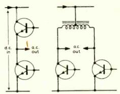
Fig.1. Using the push-pull circuit (b), right, leads to a lower Q requirement for the subsequent gyrator than with the transformerless circuit (a).
