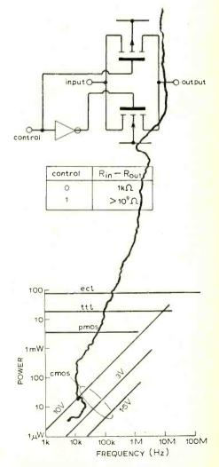
Fig. 8. For c.m.o.s. high speed means high power and low power means low speed.
