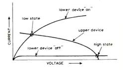
Fig. 1. Load lines of a p-m.o.s. inverter (Fig. C) intersect at a high-current point leading to significant power dissipation, around 10mW, with the lower device on. Complementary m.o.s. devices avoid this.
