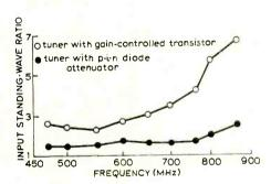
Fig. 1. Better aerial input matching is achieved in tuners using p-i-n diodes instead of gain-controlled transistors for a.g.c.
