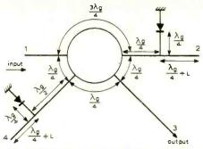
Fig. 7. Hybrid ring phase shifter makes use of directional properties of the coupler and uses p-i-n diodes to switch reactive lengths of line in and out of circuit.
