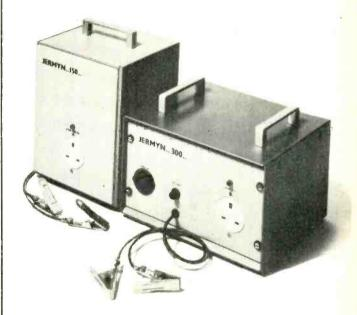
The Jermyn Invertor provides a completely portable source of 240v 50Hz power, working from an ordinary car battery.
