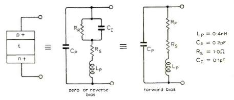
Fig. 4. Equivalent circuits for reverse and forward bias conditions of a silicon p-i-n diode.  $R_S$  is the series resistance associated with the contacts to the i-region of the diode and  $C_i$  is the intrinsic-region capacitance. Values of L and  $C_p$  are typical of devices used up to the end of X-band (8200 to 12,400MHz).
