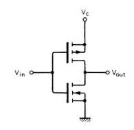
Fig. 2. By using both p- and n-channel devices in a complementary way the high power consumption of the p-m.o.s. inverter is arrived.
