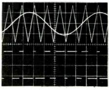
Fig. 12.2 The upper traces show the two input signals to the circuit (2V/div.) and the lower trace the output of width-modulated pulses (10V/div.). Horizontal scale, 10ms/div.
