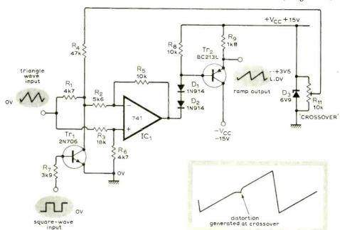
Fig. 13. Circuit of the ramp function generator.
