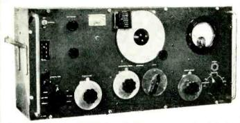
MARCONI SIGNAL GENERATOR TYPE TF-144G: Freq. 85 Kc/s-25 Mc/s in 8 ranges. Incremental: ±1% at 1 Mc/s. Output: continuously variable 1 microvolt to 1 volt. Output Impedance: 1 microvolt to 100 millivolts, 10 ohms 100mV - 1 volt - 52-5 ohms. Internal Modulation: 400 c/s sinewave 75% depth. External Modulation: Direct or via internal amplifier. A.C. mains 200/250V, 40-100 c/s. Consumption approx. 40 watts. Measurements 29 × 12½ × 10 in. Secondhand condition. £27-50 each, Carr. £1-50.
