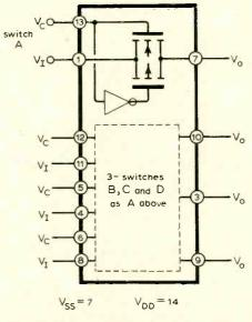
Fig. 11. This quad bilateral switch enables switches to be fully floating.
