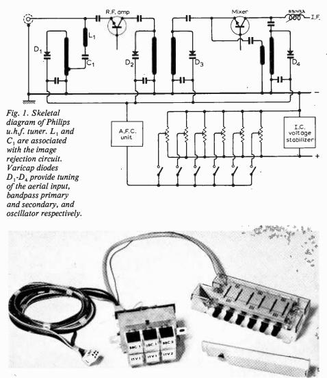
Push-button channel selector (left) and pre-set potentiometers (right) of the Philips varicapdiode tuner (Fig. 1), as used in the Philips G8 colour television receiver.
