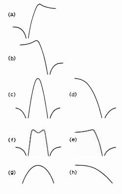
Fig. 11. Building up a 3rd-order b-p response. On the right, corresponding l-p responses.
