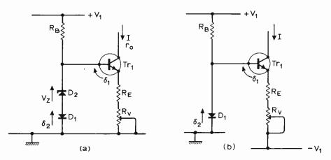
Fig. 2 (a) Popular current source circuit. (b) Current source using two rail supplies.
