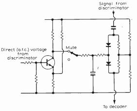
Fig. 4 (left). Interstation muting circuit in Dynatron tuneramplifier. Tuner uses diode tuning, five integrated circuits and dual-gate f.e.ts.
