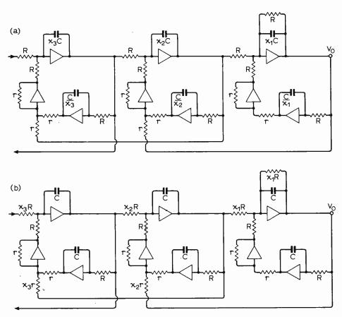
Fig. 13. As first derived the integrators of the elementary tuned circuits have different Ts (CR products). This can be corrected by making the changes shown in (b).
