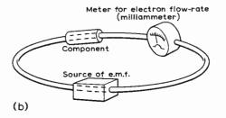
Fig.2. The Fig.1 loop with (a) a source of electro-motive force and an electronic component inserted; and with (b) a meter included to measure current.
