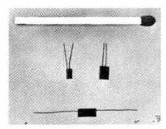
tolerances are  $\pm 20\%$ ,  $\pm 10\%$  and  $\pm 5\%$ and the operating temperature range is -55 to  $+125^{\circ}$ C. The capacitors consist of very small tantalum anode assemblies with attached leads enclosed in insulated cases filled with epoxy resin. Union Carbide U.K. Ltd, 8 Grafton Street, London W1A 2LR.
