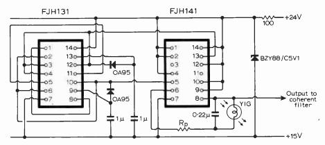
Fig. 3. Drive circuit for the YIG.
