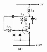
ed for conventional analysis, and Fig. B shows it with the collector of the transistor at an a.c. earth. In both circuits the tuning capacitor has been transferred to be in parallel with only the larger part-winding, simply to make the circuit look conventional.
