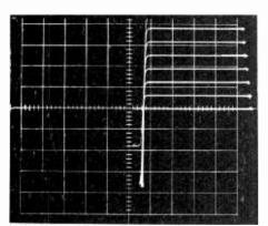
Fig. 7. Characteristics of Fig. 6(a) using sample X (Plessey). Scales: vertical 0.05 mA/div; horizontal 1 V/div. Steps: 0.1 A.
