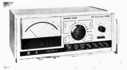
Wayne Kerr stand during the I.E.A. exhibition earlier this year, also measures direct voltage and resistance. Amplifier uses photochopper stabilization with 40-Hz switching to avoid beats with the 50-Hz supply. Instrument also features a small reverse scale for null detection, overload protection, one set-zero control for all ranges, a recorder output of 0-1mA at 1k $\Omega$ , and a hum rejection filter which rejects hum equivalent to 50 × f.s.d.
