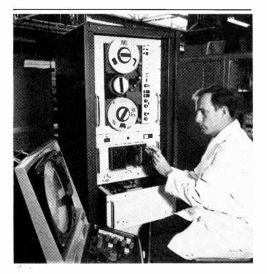
Designed primarily for air traffic control use by Solartron the interface equipment shown allows a standard television tape recorder to be used to record radar data for subsequent analysis on a radar display.
