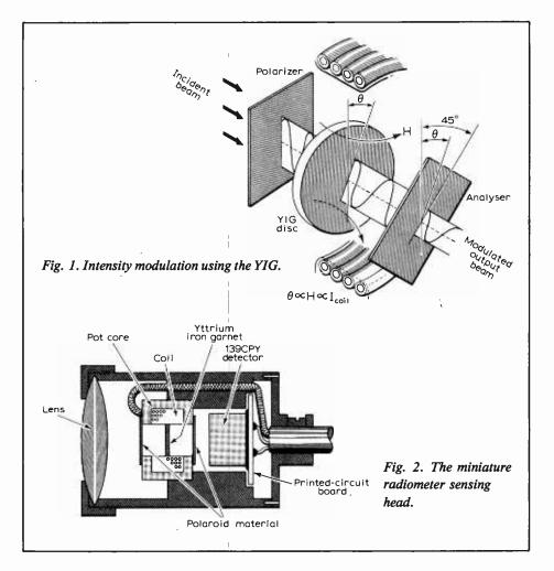
with a rotating segmented chopper-disc. The size of such a disc with its associated driving motor has necessarily led to rather bulky sensing heads in previous equipments, however the YIG solid-state optical modulator removes such size restrictions. The total absence of all moving parts has also eliminated the need for servicing.
