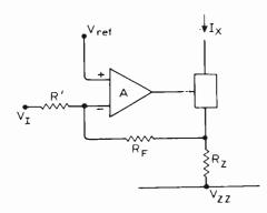
Fig. 9. Variation of Fig. 8(a) for reduced current from  $V_I$ .
