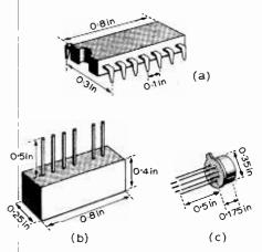
Fig. 4. Typical common low-power linear microcircuit packages for attachment to non-copperside of printed circuit board: (a) Dual-in-line; (b) single-in-line; (c) multilead TO-5.
