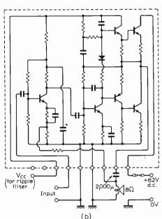
Fig. 7. Typical commercial example of high-power linear microcircuit (Sanken Electric SI-1050A, 50Watt Hi-fi power amplifier). (a) Package; (b) hybrid circuit.
