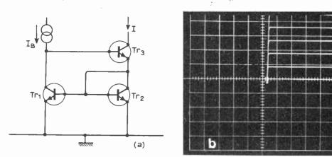
Fig. 6. (a) "Enhanced" current mirror circuit. (b) Characteristics of Fig. 5(a) using SL303A. Scales as in Fig. 5(b).
