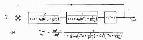
Fig. 5. A two-lag loop and its band-pass counterpart.
