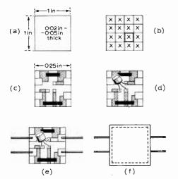
Fig. 3. Construction of thick-film hybrid microcircuits: (a) Starting ceramic substrate; (b) number of identical R, C and conductor networks printed and fired on substrate; (c) single circuit substrate scribed and cracked from complete multiple-unit substrate; (d) discrete components such as transistors attached to substrate. (e) Leadout wires attached; (f) circuit encapsulated in protective package.
