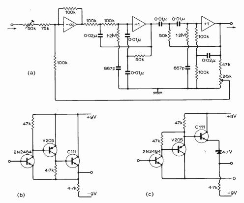
Fig. 10. (a) Schematic for  $\frac{1}{3}$ rd-octave 2nd-order band-pass filter, centre frequency 159 Hz, peak gain 18 approx. (b) Enhanced emitter follower using three transistors. (c) Simple high-gain amplifier.
