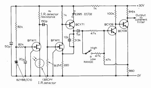
Fig. 4. Low-noise preamplifier circuit with compensatory detector bias.
