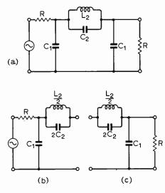
Fig. 12. Bisection of a symmetrical filter.
