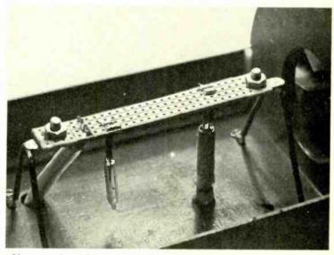
Close-up of the dry (left) and wet (right) thermistors and their mount.
