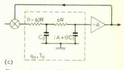
Fig. 15. (a) loop with lag and integrator not isolated by a buffer; (b) equivalent circuit when  $A = \infty$ ; (c) equivalent circuit when  $A < \infty$
