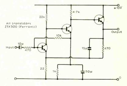
Wide-range Wien Bridge Oscillator. The oscillator has five ranges as follows: 15-200Hz, 150Hz-2kHz, 1.5-20kHz, 15-200kHz and 150kHz-2MHz. The output is IV r.m.s. with less than 0.2% harmonic distortion at 1kHz. Frequency of oscillation is given by  $1/2\pi RC$ . Extracted from the publication "E-Line Transistor Applications" produced by Ferranti Ltd.
