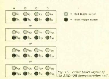
Basic facts like  $A\overline{A} = 0$  and  $A + \overline{A} = 1$  can be instantly demonstrated using the demonstration unit. It can also be used to demonstrate minimization (ABCD + ABCD = ABC.etc.)
