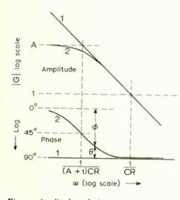
Fig. 5. Amplitude and phase curves for an ideal integrator (1), and a finite-gain integrator (2)
