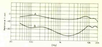
Fig 7. Curves A and B show, respectively, the wanted signal and the crosstalk into the second channel, from a ceramic cartridge loaded by  $2M \Omega$  and of 5g playing weight. The temperature is  $21^{\circ}C$  and the test record TC5702.
