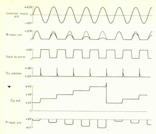
Fig. 3. Waveforms of potential with respect to staircase generator negative rail, when the test transistor is an n-p-n type with an external load.
