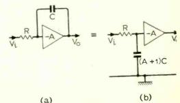
Fig. 4. The equivalence shown in Fig. 2 applied to a Blumlein feedback integrator
