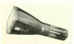
tube has a writing speed in the storage mode of  $0.5 \text{ cm}/\mu$ s, a deflection sensitivity of approximately 12V/cm in both axes, at a writing beam voltage of 1.5kV, a typical line width of 0.4mm in the c.r.t. mode. The English Electric Valve Co. Ltd, Chelmsford, Essex.
