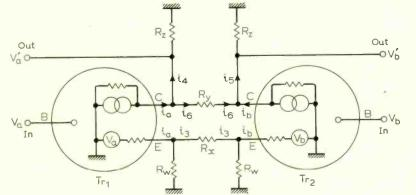
Fig. 3. Equivalent circuit of Fig. 1.
