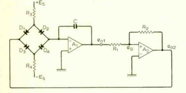
Fig. 8. Schematic for generator of triangular and square waves.
