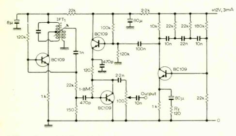
470kHz oscillator with 220Hz modulation, submitted by K. E. Potter. Modulation is at about 90%.
