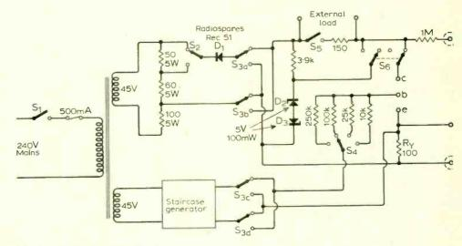
Fig. 1. Main circuit of curve tracer.
