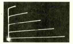
Fig. 4. Characteristic curves for (above) 2N1304—  $\Delta I_{b}=10\mu A$ ,  $I_{c}=0.4mA/cm=1.5V/cm$ ,  $load=5k \Omega$  (below) 2N3819—  $\Delta V_{gs}=1V$ ,  $I_{d}=3.2mA/cm$ ,  $V_{ds}=1.5V/cm$ ,  $load=560 \Omega$
