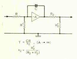
Fig. 6. Showing loss of effective gain by passive attenuation
