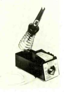
which gives a 24-volt feed into the iron from a 230-volt mains input. Price, including the continuously-variable temperature-controlled soldering pencil, the control unit and one tip is  $\pounds 23$ . Extra tips are 8s each. Weller Electric Ltd, Redkiln Way, Horsham, Sussex. WW306 for further details
