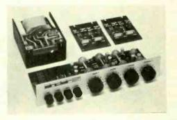
is comprehensive and seems to leave nothing to chance. It should be noted that though the Z30 amplifiers are advertised as being capable of delivering 24W continuous sine-wave this power level can only be delivered into 3 $\Omega$  with a rail just above 30V. With a 12-volt rail and a 16 $\Omega$  load the maximum continuous output power is reduced to 0.75W. Sinclair Radionics Ltd, 22 Newmarket Road, Cambridge CB5 8DU.
