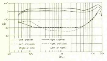
Fig. 11. Frequency response curves for photo-electric cartridge.
