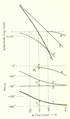
Fig. 10. Amplitude and phase curves, open loop
