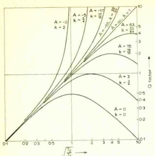
to changes in A. Indeed "designable" circuits, which can accommodate large uncertainties in the value of A, should use values of A which give q close to  $q_i$ .
