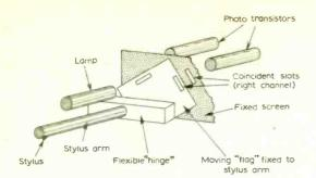
Fig. 10. Diagrammatic representation of Toshiba C100P pickup cartridge.
