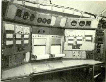
One of the two flight checking positions in the new aircraft. The one shown here handles i.l.s. and the other up to four v.o.r. or two TACAN checks simultaneously.
