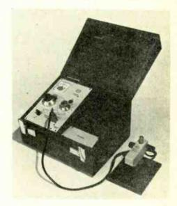
driven by the phase discriminator operating in a digital mode so that directional proximity of the null is also indicated. Bridge accuracy of  $\pm 1\%$  is claimed. A simple four-in-line configuration is used in the probe system for which low cost replaceable contacts are available. Soil resistivity may also be measured by changing the probe head for an array of earth spikes. The bridge costs £245. J. A. Radley (Laboratories) Ltd, 220 Elgar Road, Reading, Berks. WW331 for further details
