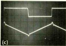
Fig. 12. Waveforms from the triangularand square-wave generator for different values of C,  $R_3$  and  $R_4$ . In (a)  $C = I \mu F$ ,  $R_3 = 56 \ k\Omega, R_4 = 680 \ k\Omega;$  horizontal scale 50 ms/div. In (b)  $C = 0.01 \ \mu F$ ,  $R_3 = 56 k\Omega, R_4 = 18 k\Omega;$  horizontal scale 0.1 ms/div. In (c) C = 220 pF,  $R_3 = 27 \ k\Omega, R_4 = 27 \ k\Omega;$  horizontal scale I µs/div. All waveforms, vertical scale 2 V/div.
