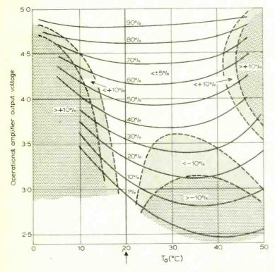
Fig. 6. Thermistor hygrometer error distribution for calibration at 20°C.
