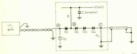
Fig. 1. Diode pulse shaper.  $D_1$ ,  $D_2 = HP_{5082-2301}$  (Hewlett-Packard);  $D_3$ ,  $D_4 = TMD_{7000}$ (Transitron);  $T^{2}L$  gate = SN7400 (Texas);  $R = I k\Omega$  (Metal Film);  $R_{T} = 50 \Omega B.N.C.$ termination.
