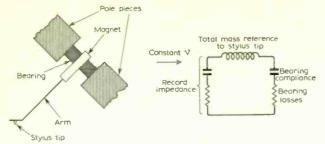
Fig. 5. Analogue of a simple armature system.
