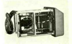
programmed by pre-punching with up to 100 holes, corresponding to the switchpositions, and stored ready for use. When a particular programme is chosen, the appropriate card is inserted in a slot in the switching device which then automatically senses the card and closes the switche corresponding to the punched holes Interlocks prevent operation from atincorrectly punched or misorientated carc
