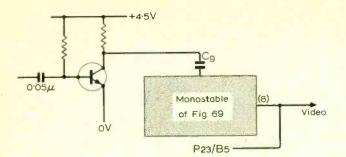
Fig. 98. Altering the blanking arrangements to give better performance and about 4V output for LAN Electronics' 19-in oscilloscope.
