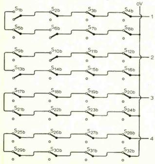
(Below) Fig. 97. Demonstrating sequential circuits. A two bit counter which may be extended to four or six bits, depending upon instrument type.
