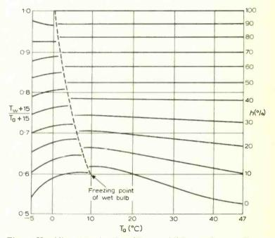
Fig. 1. Humidity curves based on  $(T_w + 15)/(T_a + 15)$  versus  $T_a$ .
