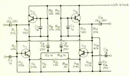
Fig. 2. Practical circuit for construction.  $R_7$  and  $R_{13}$  are ganged.
