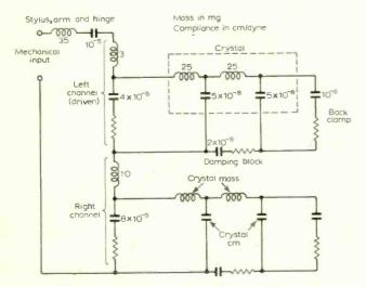
Fig. 6. Analogue of a crystal stereo pickup.
