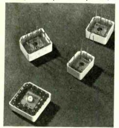
encapsulated in a resin block which is finally enclosed in a plastic box. As the electrical contacts to the component are made via either terminal spills or printed-circuit termination pins, all of which are on one face of the box, mounting in either the upright or inverted positions is easy. They are available in ten sizes. Plessey Co. Ltd, Swindon, Wilts.
