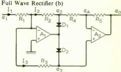
For positive inputs  $D_2$  is reverse biased and the two inverting amplifiers are in cascade
