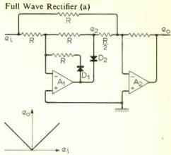
The circuit shows an arrangement commonly used to obtain full-wave rectification. The first amplifier acts as a half-wave rectifier and the second amplifier as an adder. For negative input signals  $D_2$  is reverse biased and  $e_2 = 0$ ; the output from the second amplifier is thus  $e_0 = -e_i$ . For positive input signals  $D_2$  is forward biased and  $e_2 = -e_i$ . The output from the second amplifier (the adder) is thus  $e_0 = -(e_i + 2(-e_i)) = e_i.$
