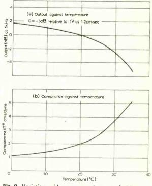
Fig. 9. Variations with temperature in a crystal pick-up cartridge.
