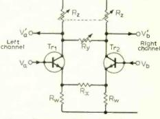
Fig. 1. Basic a.c. circuit of the design.
