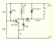
Fig. 1 Circuit of a transistor oscillator
