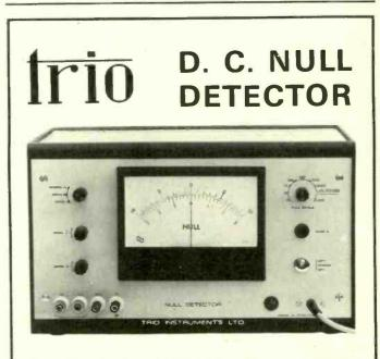
TRIO INSTRUMENTS Null Detector is a mains operated instrument intended for use with D.C. potentiometers and bridges. It features extremely high sensitivity combined with low noise and drift. Maximum sensitivity is 1 uV., F.S.D. which combined with a noise level of less than 0.05 uV peak to peak permits the use of this instrument at voltage levels of 0.1 uV.
