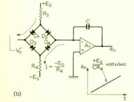
negative levels of comparator output voltage in the Fig. 8
