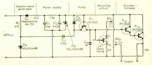
Fig. 2. Circuit of staircase generator.
