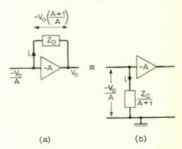
Fig. 2. Mathematical equivalent of an amplifier with a shunt feedback impedance
