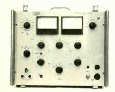
the instrument has the following specification. Transistor measurements: leakage current, 1 nA and above; collector current, 1 nA to 2A f.s.d.; collector voltage, 0-12V; base current, 0-150mA; and  $h_{fe}$ (1kHz); 0-1500. Diode measurements: forward voltage drop (at 2A) 0-12V d.c.; reverse voltage, 0-1kV d.c. f.s.d.; and reverse current, 10 nA and above. K.S.M. Electronics Ltd, Bradmore Works, Bradmore Green, Brookmans Park, Herts. **WW332 for further details**
