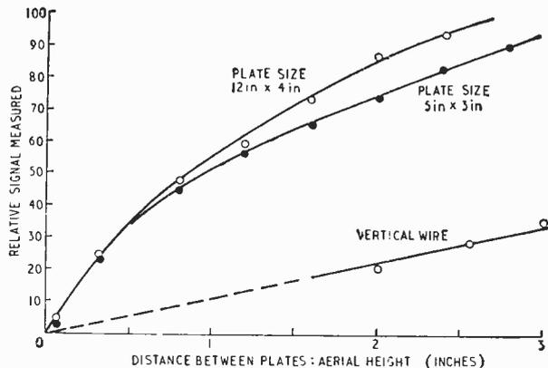
Fig. 3.  $v_a$  into the receiver using the aerial amplifier.
