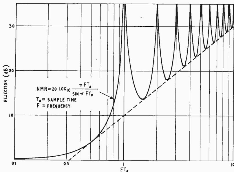
Fig. 8. Normal mode rejections for normalized frequency for an integrating d.v.m.
