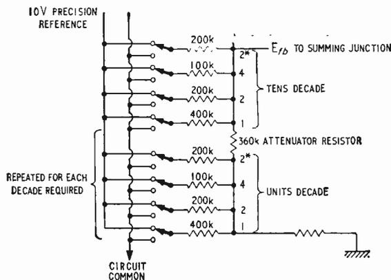
Fig. 2. Simplified bridge diagram.
