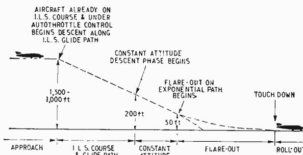
Fig. 1. Vertical plane diagram of the automatic landing sequence (not to scale). I.L.S. azimuth guidance is provided throughout.
