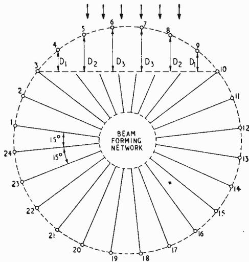
Fig. 4. A plan view of the 24 aerials used in the multiple beam receiving array.
