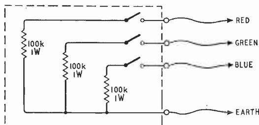
Fig. 1. "Gun-killer" switch box circuit: insulating flexible crocodile-clipped leads arranged so that, by clipping to the three grids of the colour picture tube and to chassis, signals on any grid can be shorted out via a 100kΩ resistor to earth.
