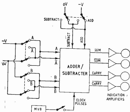
change-over switches and a multivibrator, the output states being displayed by the standard indication circuit. A single-pole switch determines whether clock pulses from the multivibrator are fed to the adder/subtractor or not. The outputs should conform to the addition and subtraction tables given earlier. An example of a test would be as follows:—
