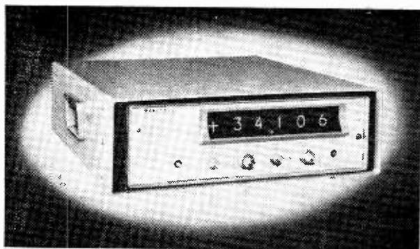
The Honeywell Model 85 successive approximation digital voltmeter.
