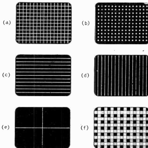
Fig. 4. Patterns commonly used in commercial crosshatch/dot generators: (a) crosshatch; (b) dot, (c) horizontal lines; (d) vertical lines; (e) crossed lines; (f) grey scale checkerboard.
