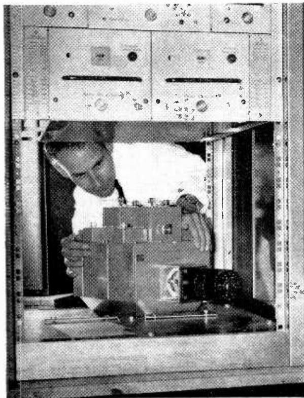
Fig. 2. Mechanical modulator for the "quadrature clearance" system used in I.L.S. ground equipment recently introduced by S.T.C.
