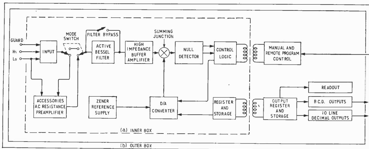
Fig. 4. Block diagram of the Honeywell Model 85 successive approximation d.v.m.
