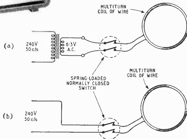
Fig. 8. (below) Two basic types of degaussing coil arrangements: (a) low-voltage transformer driven; (b) high-voltage mains-driven.
