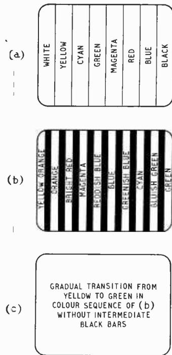
Fig. 5. (left) Commoner patterns in commercial colour bar generators: (a) PAL (test card); (b) keyed-rainbow; (c) simple rainbow.
