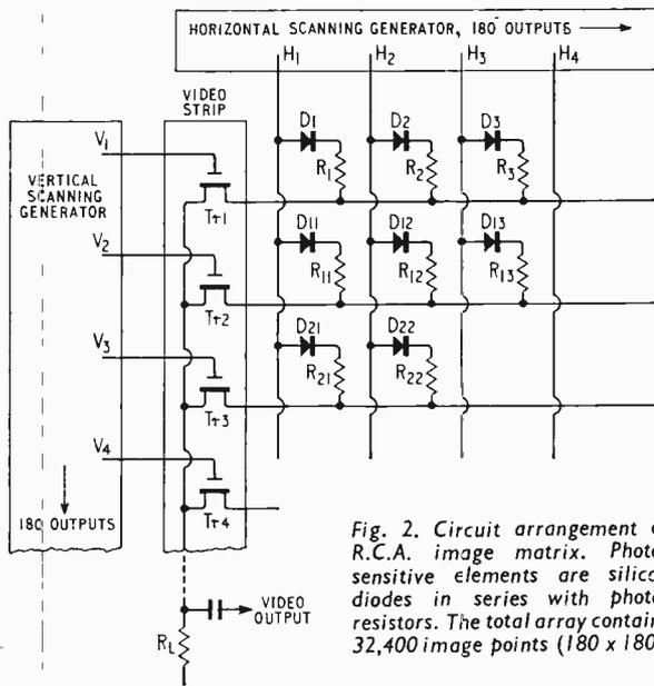
Fig. 2. Circuit arrangement of R.C.A. image matrix. Photosensitive elements are silicon diodes in series with photoresistors. The total array contains 32,400 image points (180 x 180).
