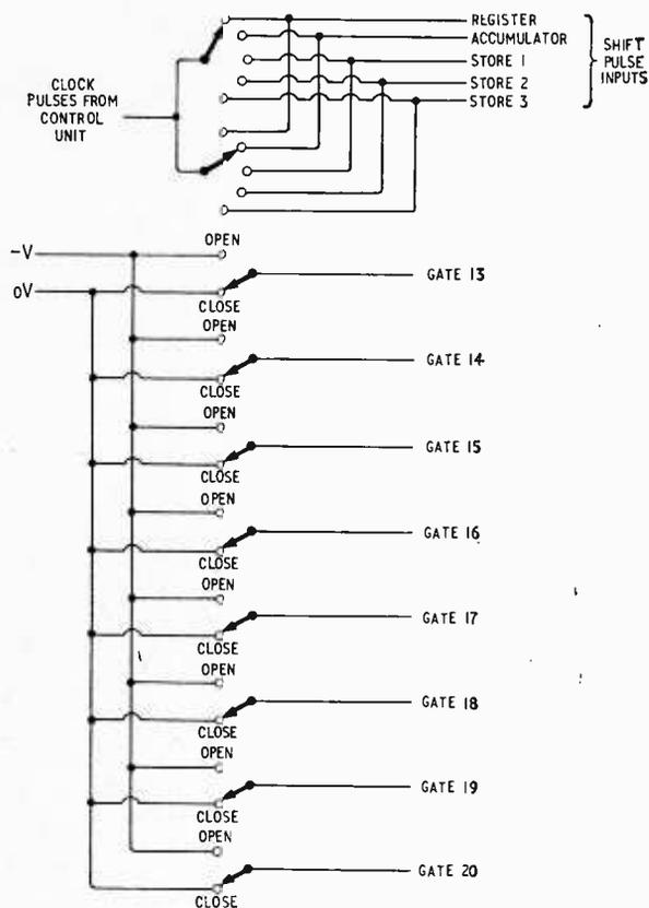
Fig. 39. Arithmetic and data transfer test switching.
