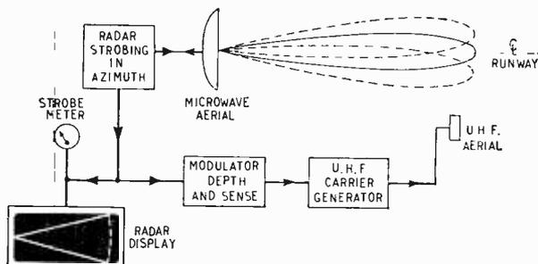
Fig. 8. Radar strobing system for azimuth guidance.
