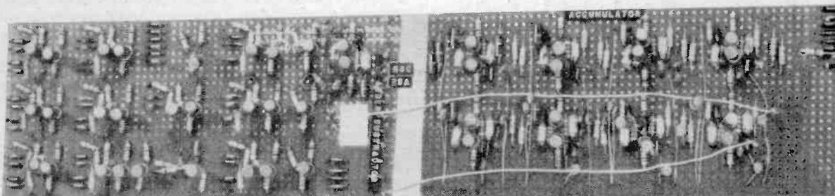
Circuit boards carrying the adder/subtractor (left) and accumulator (right).
