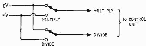
Fig. 38. Test input switches for checking control unit.
