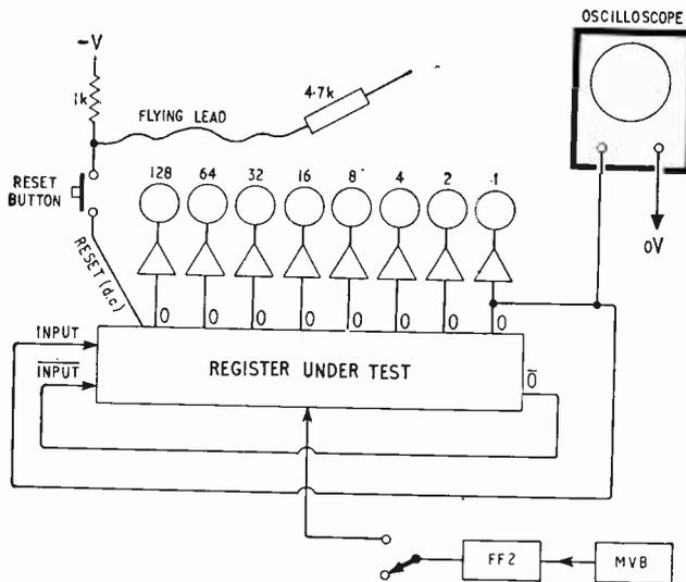
Fig. 37. Shift register test circuit.
