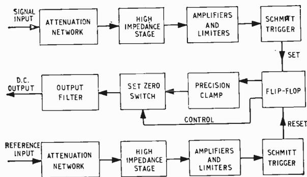
Fig. 13. Block diagram of a phase converter.
