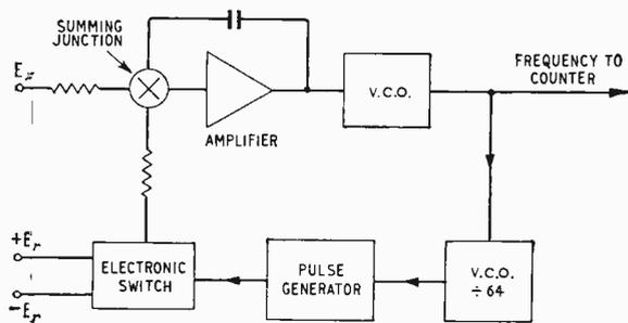
Fig. 10. Schematic of a d.c. to frequency converter.
