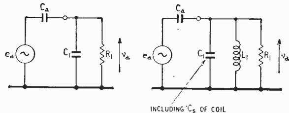
Fig. 1. Aerial equivalent circuits. In the l.h. drawing  $v_a = [C_u / (C_u + C_1)] e_a$ , and  $R_1 > 1/\omega C_1$ . In the r.h. drawing  $v_a = [C_u / (C_u + C_1)] Q e_a$ .
