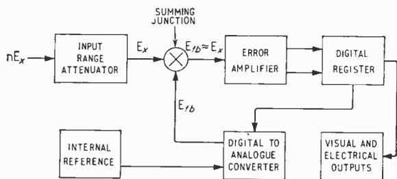
Fig. 1. Block diagram of a continuous balance d.v.m.
