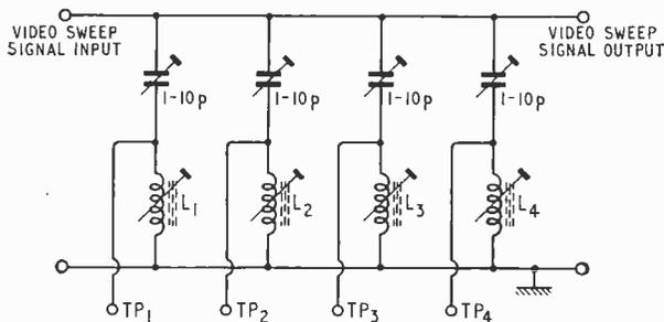
Fig. 3. Video sweep absorption marker-box circuit.
