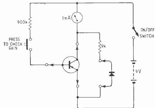
Fig. 32. Circuit for testing transistors and diodes.
