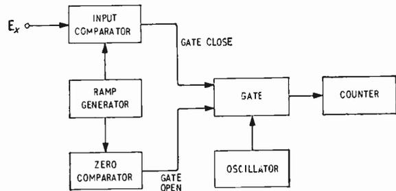
Fig. 5. A typical ramp d.v.m. layout.
