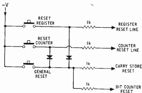
Fig. 35. Auxiliary reset press-button circuits.
