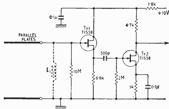
Fig. 2. The broadband amplifier circuit.
