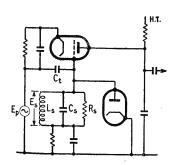
Left: Fig. 11. Circuit of synchrotector with sampling pulses derived from input signal.
