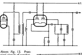
Above: Fig. 13. Practical circuit of synchrotector preceded by locked-oscillator limiter.
