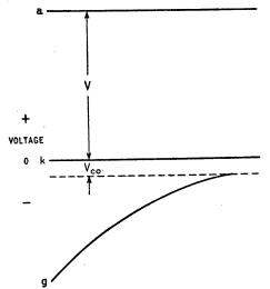
Fig. 3. Electrode potentials of valve in Fig. 1 during discharge phase of blocking oscillator cycle. The dotted line marks the minimum cut-off grid bias, Veo, when the anode is at +V volts.
