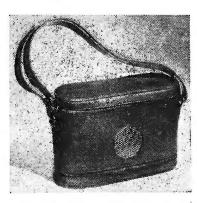
PRINTED CIRCUITRY is used in this four-valve Roberts' battery portable housed in a leather case. Access to the control panel and the batteries is gained by two zip-fastened covers. The current consumption is h.t. 10.4 mA, l.t. 125 mA.
