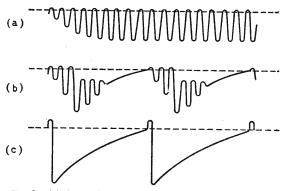
Fig. 2. (a) Start of oscillations in sine-wave oscillator in circuit very similar to Fig. I except for closeness of coupling. (b) Squegging condition obtained by increasing the coupling slightly. coupling to the limit. (c) Alleged result of tightening
