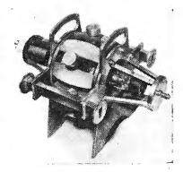
Mullard five-cavity klystron
