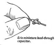
BS415-1957 and is made in five sizes with capacitances of from 470 pF to 20 kpF. The latter is for earth leads Another "aerial isolator". but of tubular ceramic form with side-entry wires, was shown by Stability Capacitors. It measures 0.7 in long, 0.2 in in diameter and conforms also with BS415. Normal values are 470 pF, 1 kpF and 1.8 kpF.
