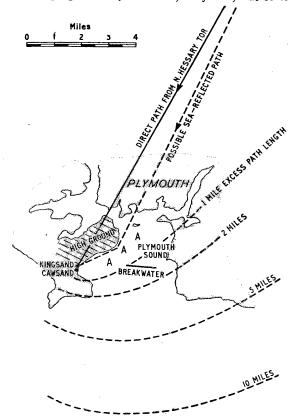
Fig. 1. Plan of the affected area and its environs, showing ellipses through reflection points giving various path differences.
