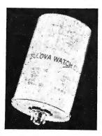
simplified, made more dependable and can have a far wider operating range. The oven is normally mounted on a standard octal base, weighs less than 7½oz, dissipates an average of 5 watts after warm-up and has the high stability of ±0.1°C.
