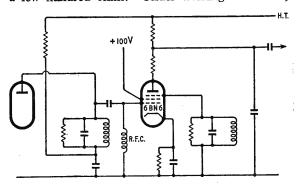
Fig. 8. Circuit used with 6BN6 gated-beam discriminator.
