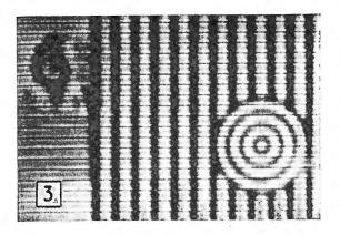
other things a stepped effect when diagonal or curved lines are scanned, as shown in Figs. 2 and 4, with consequent deterioration of picture quality.
