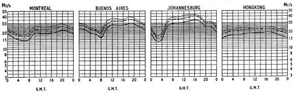
THE full curves given here indicate the highest frequencies likely to be usable at any time of the day or night for reliable communications over four long-distance paths from this country during June.
