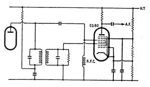
Fig. 3. Circuit for use with nonode discriminator.
