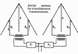
central mast A in each pair Br, Bz and B3, B4 of the outer aerials will be in phase, and will therefore cancel at the terminals of the second transmitter. The symmetry of the arrangement preserves the normal radiation pattern of both the aerials.
