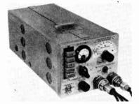
Plessey 5-channel V.H.F. radio telephone for light aircraft.
