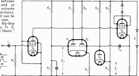
Fig. 3. Improved flip-flop circuit. Typical values :—  $R_1 = 100$ k $\Omega$ ,  $R_2 = 100$ k $\Omega - 3M\Omega$ ,  $R_6 = 6.8$ k $\Omega$ ,  $R_L = 8.2$ k $\Omega$ ,  $R_z = 4$ k $\Omega$ ,  $C_1 = 100$ pF,  $C_2$  according to required  $t_0$ ,  $E_1 = 40$ V,  $E_2 = 55$ V, E = 250V volts,  $V_1 V_2 = ECC_3 z$  or 6N7,  $V_4 = V_3 = EF_50$ ,  $V_5 = EA_50$ . N.B. For  $t_0 < 10 \mu$ sec miniature values would be desirable.
