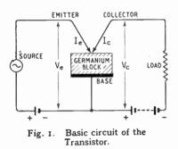
by placing point contacts of tungsten or phosphor bronze in close proximity (0.05 to 0.25 mm) on the specially prepared surface of a germanium block, interdependence of currents in the vicinity of the contacts can be utilized to obtain power amplification of the order of zodb.
