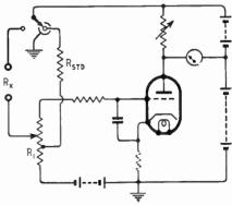
Fig. 4. The addition of a backing-off circuit to Fig. 3 is shown here.
