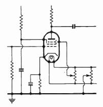
Method of balancing out hum voltage.
