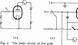
rig. 2. The basic circuit of the gridcurrent megohimmeter is shown at (a) and its practical form at (b).
