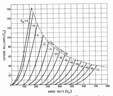
Fig. 3. Characteristic curves for triode-connected EL37 valve for VI duty.
