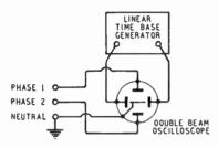
Fig. 2. A practical method of distinguishing negative from positive frequency.
