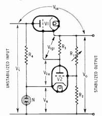
Fig. 1. Basic circuit of series-valve stabilizer, in which the output voltage  $V_0$  is adjusted by varying  $R_1$ . N is the voltage reference standard, and V2 the negative feedback amplifier.
