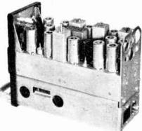
are used in a dual capacity, the crystal oscillator and frequency multipliers being one example. These serve either as a crystal drive for the transmitter, or, with an appropriate crystal switched in, become the local oscillator for the receiver. Then, the two audio stages function either as modulator or as A.F. amplifier for the receiver.
