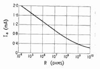
[Courtesy Journal I.E.E. Fig. 1. This curve shows the relation between anode current and resistance for a grid-current type of megohmmeter.
