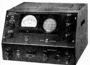
THE VOLTASCOPE—A combined valve-voltmeter and oscilloscope. VALVE-VOLTMETER—Infinite Input Resistance for D.C. ranges 0 to 300 volts. A.C. ranges 0 to 150 volts in 5 ranges.  $3\frac{1}{2}$  inch scale meter. OSCILLOSCOPE—3 inch screen tube provided with balanced amplifiers for Y and X plates giving a 5 times trace expansion. Maximum sensitivity 150mV/cm. Response from D.C. to 100 kcs.
