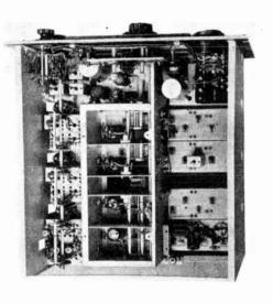
contained and very compact, weighing but  $15\frac{1}{2}$ b and measuring  $2 \times 15\frac{1}{2} \times 7\frac{1}{4}$ in, and it can be either battery or mains operated. It is thus suitable for use in vehicles on the airfield. There was also a "Walkie-Talkie" set described as the type H19.
