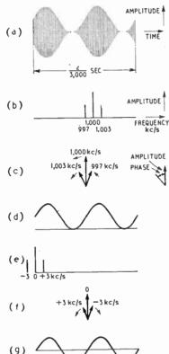
Fig. 3. A high frequency (Ioookc/s) carrier wave modulated at 3 kc/s, represented in three ways a, b, and c. A zero-frequency "carrier wave" modulated at the same frequency is shown in the same ways at d, e and f. g is an alternative to d, representing a different "phase" of the "carrier wave."
