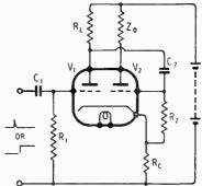
Fig. 2. Simple time delay flipflop. Typical values :-- $R_1 =$ 100k $\Omega$ ,  $R_2 = 1M\Omega$ ,  $R_L =$  100k $\Omega$ ,  $R_c = 1000\Omega$ ,  $Z_c$  = required load,  $C_1 = 100$  pF,  $C_2$  according to required  $t_0$ , E = 200 volts,  $V_1 V_2 =$ ECC32 or 6N7.
