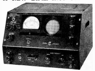
THE VOLTASCOPE—A combined valve-voltmeter and oscilloscope. VALVE-VOLTMETER—Infinite Input Resistance for D.C. ranges 0 to 300 volts. A.C. ranges 0 to 150 volts in 5 ranges. 3½ inch scale meter. OSCILLOSCOPE—3 inch screen tube provided with balanced amplifiers for Y and X plates giving a 5 times trace expansion. Maximum sensitivity 150mV/cm. Response from D.C. to 100 kcs.
