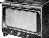
Built with a push-pull output stage giving 8 watts undistorted output. Incorporates a 10 loudspeaker. Covers long, medium and two short wave ranges. Voltages as for 516 T.G.
