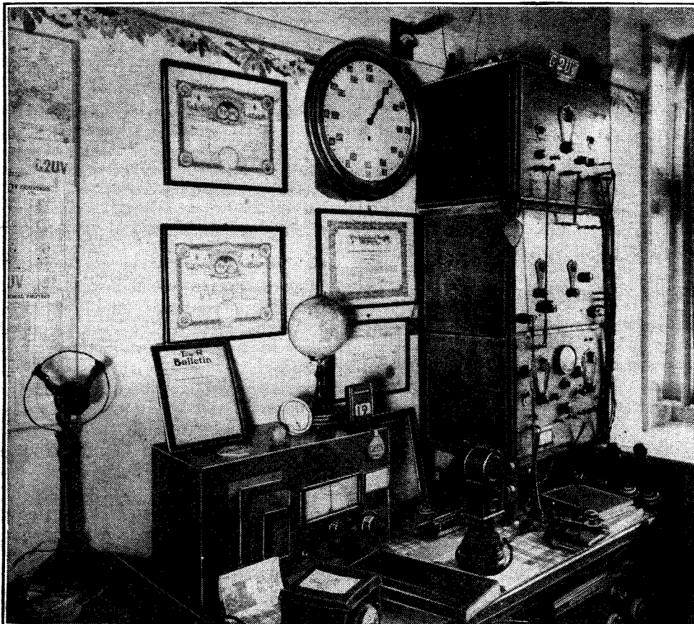
AMATEUR TRANSMITTING STATION G2UV. This station owned and operated by Mr. W. E. Corsham, at Wembley, Middlesex, normally works on the 14-Mc/s band (21.42-20.83 metres) using both telephony and CW system of transmission. The station can often be heard working in the evenings and most mornings at 9 a.m., at which hour Mr. Corsham usually carries out tests with amateur transmitters in New Zealand.
