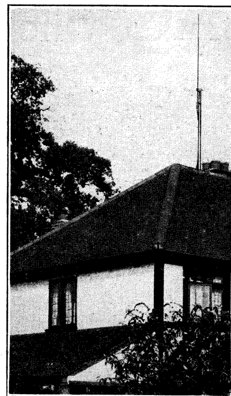
Courtesy Belling and Lee A modern aerial, if necessary of the anti-interference type, improves signal/noise ratio and appearance.
