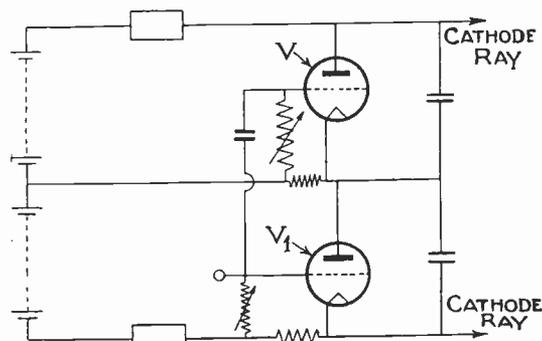
Fig. 1.—Circuit for producing interleaved scanning. Patent No. 423,101.
