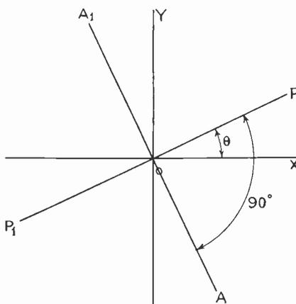
Fig. 1.—Linear polariscope with crossed nicols.— $PP_1$  is the vibration direction of polariser;  $AA_1$  is the vibration direction of analyser;  $OX, OY$  are the vibration directions of birefringent section in the polariscope.
