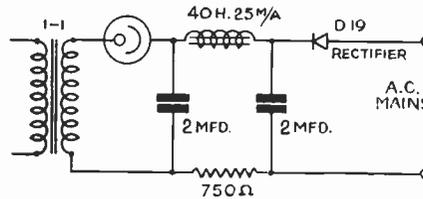
It is an expensive hobby running a neon lamp from dry batteries, so if you have mains laid on use a metal rectifier of the half-type wave. Don't forget the small resistance in series with one side of the supply.
