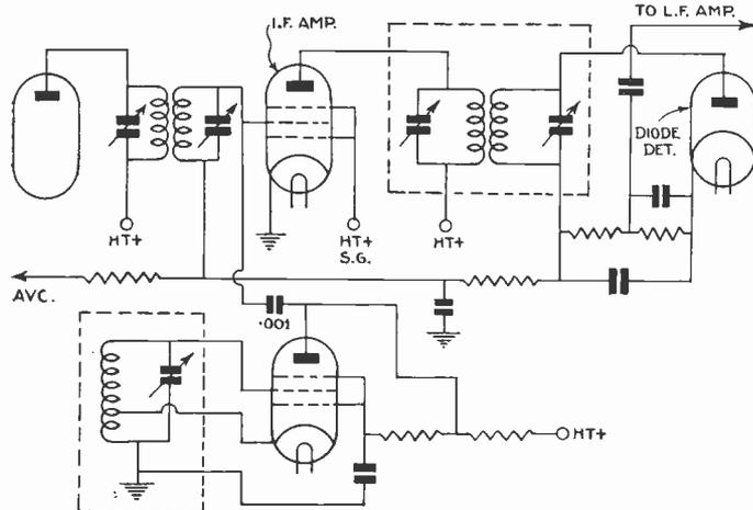
Fig. 1.—By feeding the output from a beat note oscillator into the grid of an I.F. amplifier, C.W. reception is considerably simplified. No super-het without an oscillator of this kind is suitable for C.W. reception.
