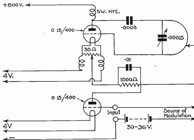
capacity may constitute quite an appreciable portion of the total capacity of the circuit. In these circumstances if the oscillating current is heavy, the glass in the pinch of the valve begins to heat up and the valve may deteriorate. In the present instance the circuit oscillates over a range of 5-11 metres and, since it will normally be wanted for wavelengths around 7-10 metres, where there is quite an appreciable capacity in parallel with the coil, this difficulty does not arise.
