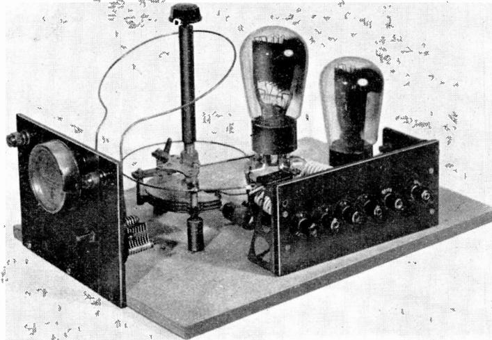
The 7-metre test transmitter.
