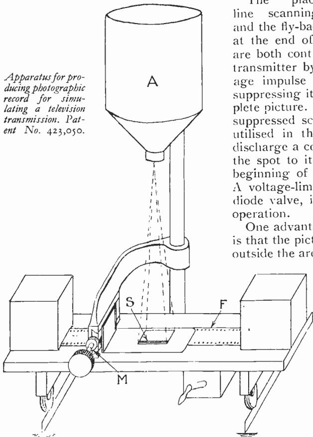
Apparatus for producing photographic record for simulating a television transmission. Patent No. 423,050.
