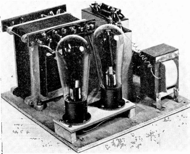
Photograph of the power unit for 7-metre transmitter.
