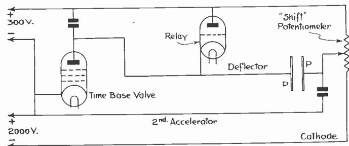
necessary to remember that the focusing of the beam depends on the potential of the final field through which it passes on its way to the screen. With the deflector plates connected to the second accelerator, this potential is that of the second accelerator itself, and the spot can be focused in the usual way. When, however, a deflecting voltage is applied to the plates these will fluctuate in potential above and below that of the second accelerator, and thus tend to alter the focus of the beam.
