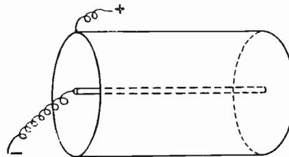
Fig. 4.—Form of cell electrodes.
