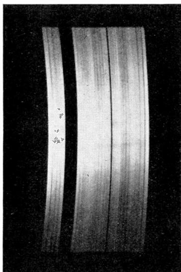
Fig. 1.—Illustrating the effect of an exposure of one-fifteenth sec. Note the vertical bands due to mains modulation on the lamp and indicating asynchronousism. The thin vertical black line is a faulty hole in the disc.
