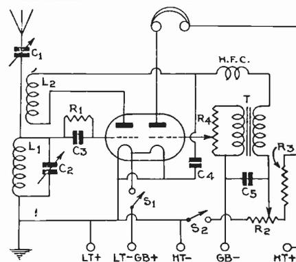
while the values should be .00025-mfd. for C<sub>2</sub>, .0001-mfd. for C<sub>1</sub>, .0003-mfd. for C<sub>3</sub>; R<sub>2</sub> is 25,000 ohms, with a class B valve, such as the Cossor B240. The remaining components are of standard values and are not critical.
