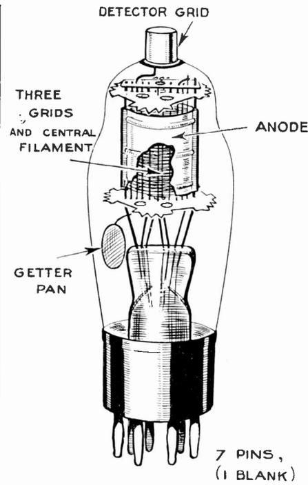
Fig. 5.—All the electrodes in this Osram heptode can be quite clearly seen. A point to remember is that the control grid is taken to the top cap.
