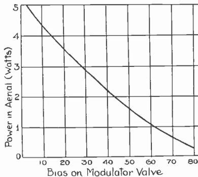
Fig. 6 (left).—Modulation characteristic.
