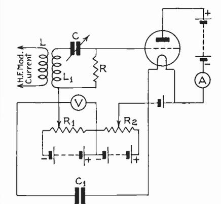
*This is the circuit for the suggested meter. It is better to use this than to rely on the fact that 23 per cent. rise should mean 100 per cent. modulation.*
