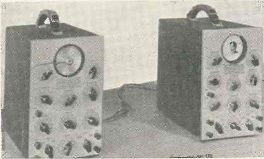
Two oscilloscopes being used as transmitter and receiver and providing a very simple arrangement for test purposes.
