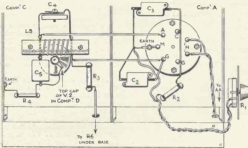
The drawings above give the wiring details of compartments C and A of the vision unit.
