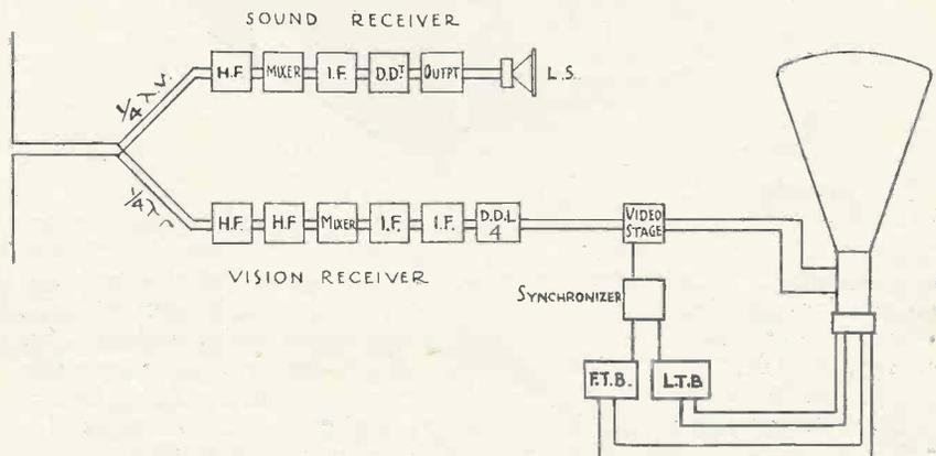
This schematic diagram gives a very good idea of the valve layout in the small Cossor receiver.
