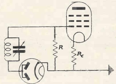
Fig. 3. How the polarity of voltage across R can be altered.
