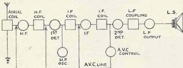
Although there are many less valves in this sound receiver the system is the same as for the vision receiver.
