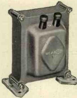
The H.T.35, like all the chokes in this series are specially layer wound—the inductance being adjusted by the air gap. Tested to 1,000 volts. Characteristics:—30 henries 50 ma., 1,600 ohms.
