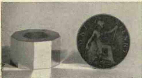
*Above: High Speed line polygon in the Mihaly-Traub receiver compared in size with a penny.*
