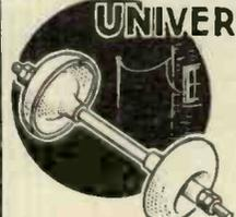
This new device fits to walls or window frames of from 1 in. to 5 in. thick and is self-adjusting. When fitted by boring a 7/16 in. or 1/2 in. hole, it gives "air-insulation" with low losses, and prevents ingress of moisture and dirt. With long-path glazed-porcelain insulators, nickel-plated metal rod, nuts and washers. Suitable for all wave-lengths. 5,000-volt insulation. List No. L.11. Price 1/6 each.
