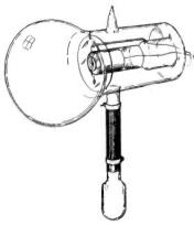
Above: The newest Bell Telephone Lab's., neon tube, having a concentrated or "crater" target, which provides a better image than before.
