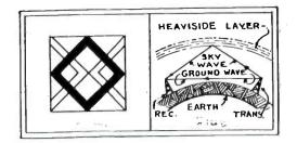
Fig. 1 Fig. 2 The double television image at the left is caused by the two paths of the signal, at the left.
