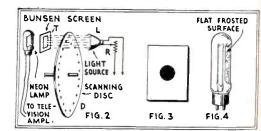
In Fig. 2, the arrangement of Mr. Fitch's proposed televisor in which stronger light may be used than at present; the expected effect is shown at Fig. 3. A tube like that in Fig. 4 will simplify matters.
