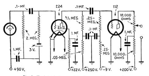
Fig. 5. Typical television amplifier for use with photo-cell.
