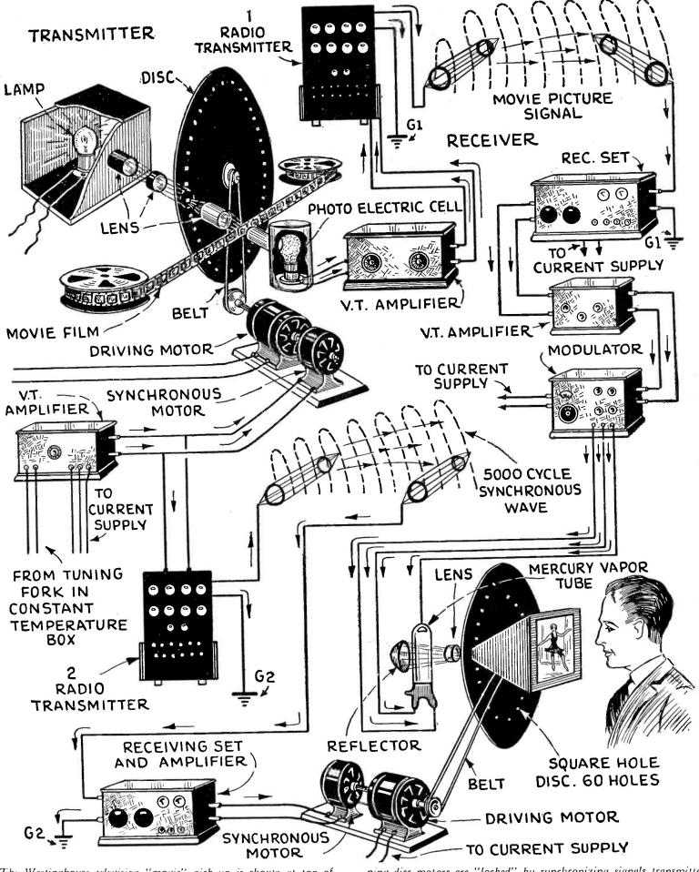
The Westinghouse television "movie" pick-up is shown at top of Diagram, while method of reproducing the movies is shown in lower right-hand corner of diagram. The transmitting and receiving scan-
