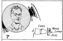
7. DIM IMAGE—Cause: (a) Insufficient signal strength. (b) Too much current through television lamp. (c) Too much outside light. Remedy: (a) Television signals should be uncomfortably loud on loudspeaker to properly operate television lamp. Use more powerful amplifier. (b) if television lamp is in series with output tube cut down current by increasing grid blas or reducing plate voltage, or inserting resistance in plate circuit. (c) Darken room.
