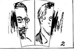
2. OUT-OF-FRAME HORIZONTALLY—Cause: Receiving scanning mechanism in step but slightly out of phase with transmitter. Remedy: If using a synchronous motor rotate field slightly until image is centered or move television lamp around the periphery of the disc until image is centered.
