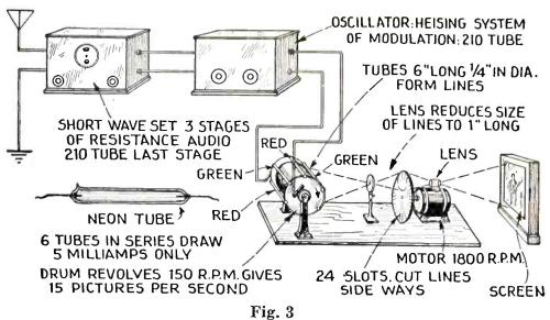
Schematic arrangement of the Gould system of colored television reproduction.
