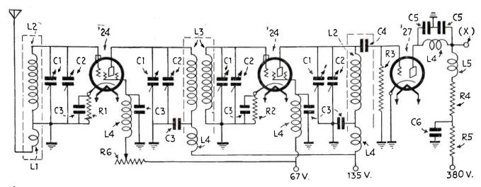
Diagram here with shows the connections of the Jenkins Television receiver or "tuner", utilizing screen grid tubes in two radio frequency stages, end a '27 tube in the detector stage. The output terminal "X" joins with the input terminal "X" of the amplifier shown below.
