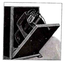
Fig. B The rear of the new radiovisor opened, to show the simple lamp-and-drum arrangement now used.
