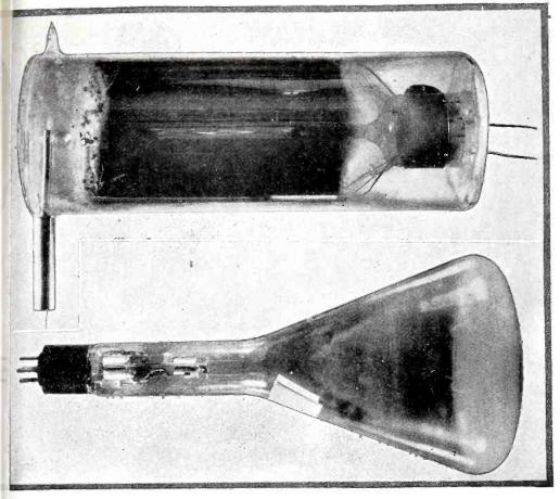
**Fig. A (above)** The "dissector tube," with its "target" shown at the left, is used for transmitting.
