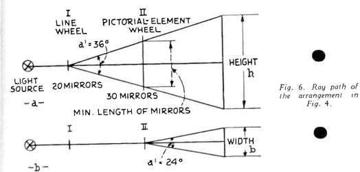
wheel, Av the number of mirrors of the vertical wheel. If we assume the horizontal wheel to have 30 mirrors and the vertical wheel 20, then with thirty-line scanning we get a ratio of 1:0.05. At the rate of  $12\frac{1}{2}$  pictures a second, that gives a ratio of 750-:37.5.
