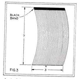
In the Baird system, which scans the image vertically, a part of the line is cut off at the upper end; this serves to create a synchronizing signal.
