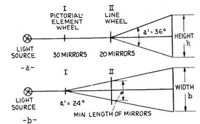
to the passage of a mirror of the line wheel. To be sure, with such a wheel, greater losses in reflection have to be put up with.
