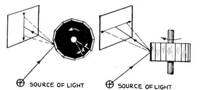
Fig. 1 (right). Horizontal or pictorial element scanning. Fig. 2 (left). Vertical or line scanning.
