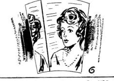
6. SHIFTING IMAGE FROM SIDE TO SIDE— Cause: Receiving and transmitting scanning mechanisms out of step. Often caused by use of synchronous motors at transmitter and receiver being connected to different power systems, whose frequencies slightly differ. Remedy: Impossible to correct with synchronous motor equipment. Can be eliminated by using self-synchronizing devices.
