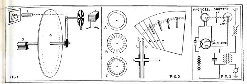
Left) Fundamental principle of the Ahronheim system: light from be image 1 is concentrated by lenses 2 on the scanning disc 3; but taches the photocell 7 only when the proper filter is presented by be disc 5, which is geared (6) to revolve faster than the scanner. Center) The Fries universal scanner: it will be seen, at the left, hat A and B combined as at C give a spiral of square holes. Four
