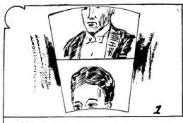
1. OUT-OF-FRAME VERTICALLY—Cause: Receiving scanning mechanism out of phase with transmitting scanner. Remedy: If using a synchronous motor stop and start motor until phase relation is same, as evidenced by the vertical centering of the picture. If using a double spiral disc shift lamp until image is centered.
