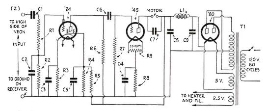
Amplifier for synchronizing motor, the input terminal "Z" connecting to the correspondingly marked terminal in the amplifier shown above.
