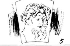
5. "GHOST" IMAGES—Cause: (a) Usually interference of the horizontal component of the transmitted wave being reflected by the Heaviside layer and interfering with the ground or vertical component. (b) Sometimes caused by reflected voltages in the radio receiver due to improperly placed impedances. Remedy: (a) For the first cause, move to different location. (b) Find the offending circuit by process of elimination.
