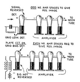
The proper number of amplifier stages for different detectors is shown above.
