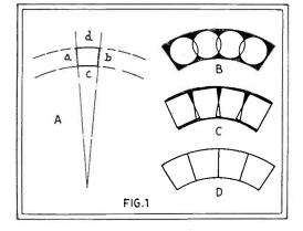
The Mihaly disc has holes (A) bounded by arcs and radii. This overcomes the unevenness of light received through circular (B) or square (C) holes; and gives perfect illumination, as at D. shifting dark lines, which are due to the holes in the scanning disc. The image is evenly illuminated and clear.
