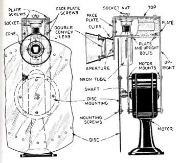
Simple home-made televisor built around an ordinary fan motor and which was successfully used by the Editor in picking up television images.
