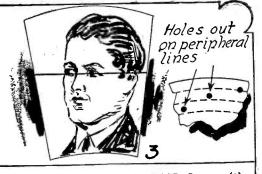
3. BLACK LINES ACROSS IMAGE—Cause: (a) Dirt in the holes of disc. (b) Hole in disc radially "off center," due to inaccurate punching. Remedy: (a) Clean disc. (b) Obtain new disc. Sometimes possible to relocate hole sufficiently to eliminate difficulty by punch and small file.
