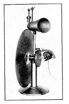
The simplified design of the receiver. In later models, gears replace the friction drive shown. The cone serves to "mask" the gears image.
