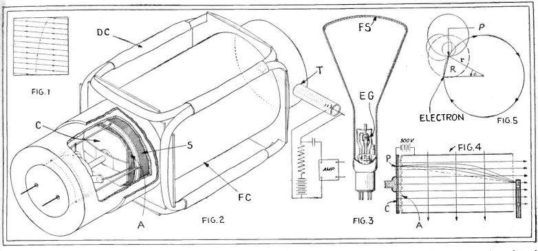
The magnetic scanning at the upper left assumes its shape as a resultant of two moving fields. The "dissector" of Fig. A is shown here internally in Fig. 2; and the "oscillite" of Fig. B in crosssection in Fig. 3. Fig. 4 illustrates the path of electrons from an
