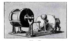
**Fig. E** A close-up of the neon-tube drum and scanner of Fig. D (and Fig. 3); red and green tubes alternate on the drum.
