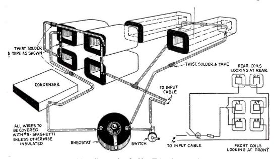
This shows wiring diagram for Jenkins Television scanning disc motor.
