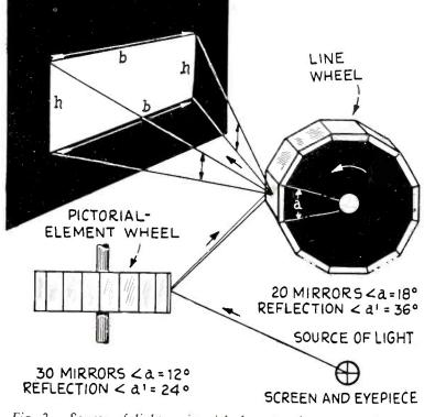
Fig. 3. Source of light-pictorial element wheel-line wheelprojection. ranged perpendicular to that of the pictorial-element wheel. This is true for the German horizontally-scanned image, as well as for the English vertically-scanned image; but for a vertical picture (*i. e.*, one with the long sides vertical) the arrangement of the two wheels must be turned through 90 degrees.
