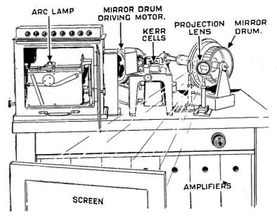
Fig. 4. The "H-M-V" television reproducer, which utilizes five light values to modulate the arc beam and yield a 20 by 24 inch brilliant picture.
