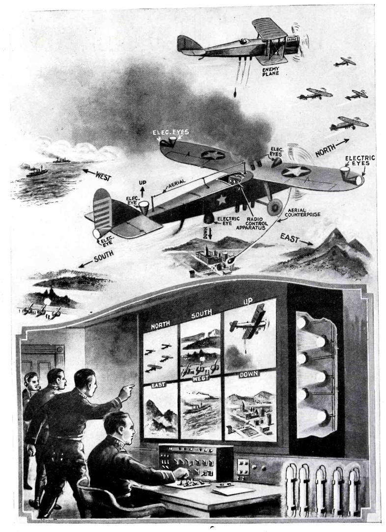
The Pilot-less radio television plane, directed by radio; the plane's "eyes" radio back what they see.
