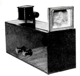
Fig. C (above) One of the models of the Gould spiral-tube television receiver.
