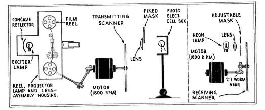
Arrangement of "movie" television projector at left; receiver at right.
