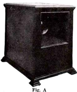
The radiovisor in its plain cabinet; the image is formed at the end of the "shadow box."
