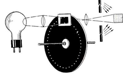
Fig. 2, at left, illustrates how the object to be televised (transmitted) is illuminated by light  $f r \circ m s a y t w \circ$ sources; the reflected light beams are transmitted through the lens, scanning disc, diaphragm, s e c on d lens and on t o photo-cell at extreme left. This cell converts the light pulsations into electric current variations.
