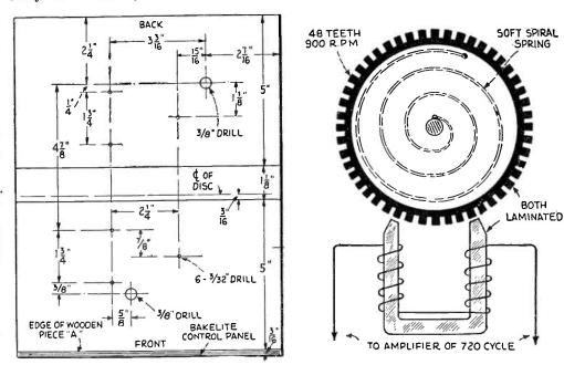
Drawing above shows layout of holes on motor base at left, while diagram at right shows arrangement of synchronizing motor of Jenkins Radiovisor.
