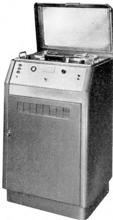
The Mufax tape recorder console, reproduced by courtesy of Muirhead & Co. Ltd., Beckenham, Kent
