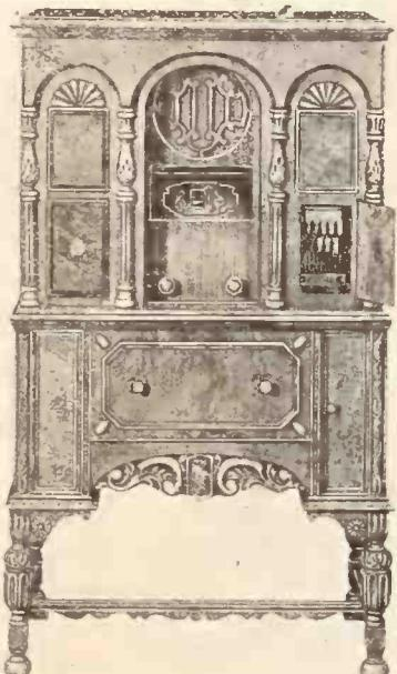
**Zenith Model 37-A** tion with Zenith automatically tuned radio receiver. Special induction-type phonograph motor with control eliminating extraneous noises. Turntable mounted on jeweled bearings, and uniform speed-control is obtained through special control-knob. Built-in dynamic speaker. Instrument employs eight AC tubes, including rectifier, operating on 110-volt 60-cycle alternating current. Retail price, \$625, without tubes.
