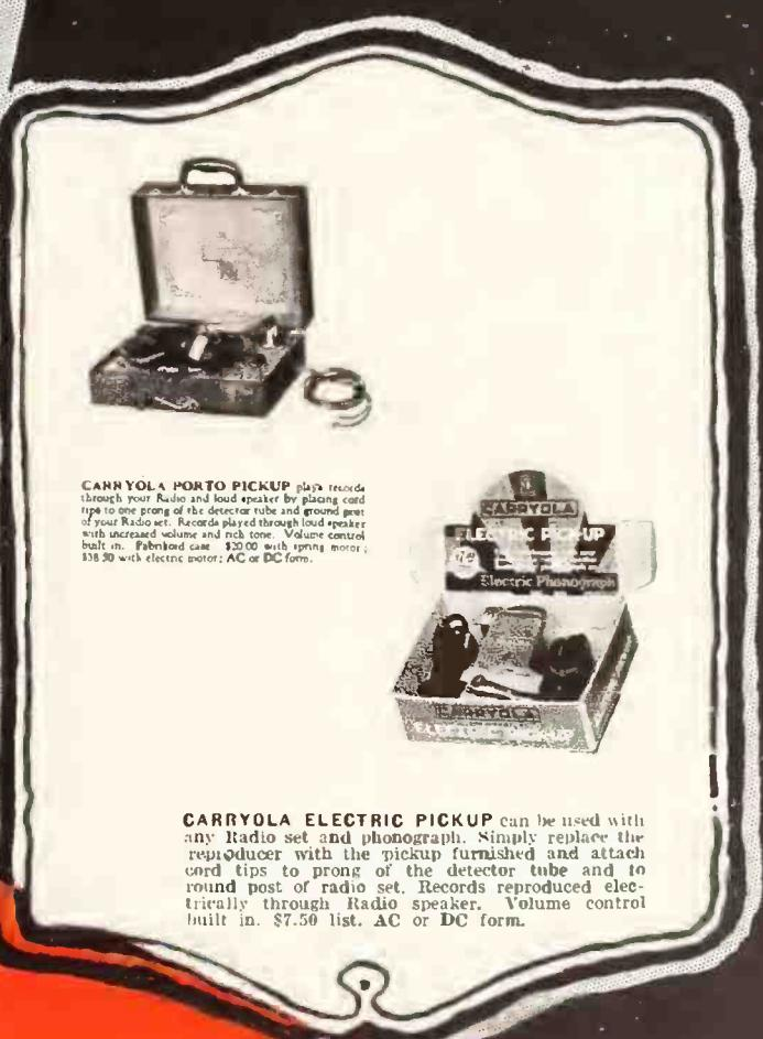
CARRYOLA PORTO PICKUP plays records through your Radio and loud speaker by placing card tips to one prong of the detector tube and ground post of your Radio set. Records played through loud speaker with increased volume and rich tone. Volume control built in. \$7.50 list. \$2.50 with spring motor; \$18.50 with electric motor, AC or DC form.
