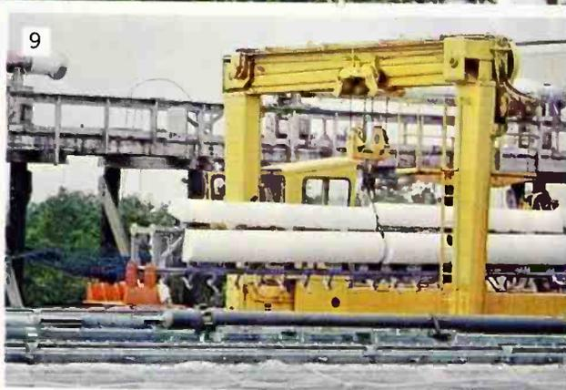
(5) Assembling one of the largest Pylon Antennas ever built. It will provide a base for a large Super Turnstile antenna in a stacked antenna arrangement.
