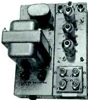
**Low band bridging amplifier, Model BA-254.** Four distribution line outputs. Gain: 20 db (bridging gain to each output). Maximum output level—5 channel operation: +42 dbmv (non-cascaded). Manual gain control and plug-in attenuators provide ample control of gain. Self-
