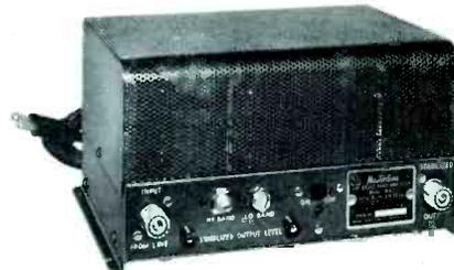
**Automatic gain control** for use with CATV broadband amplifiers, Model MAC. For use with any broadband VHF amplifier having more than 16 db gain and producing an output between 0.6 volts and 2.5 volts per band. It will maintain the output at a constant level (less than 1 db change in output level for a 10 db change in input). In addition to providing AGC the MAC can deliver up to 10 db additional gain. Net: \$121.50.
