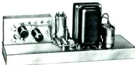
**Low band single channel VHF amplifier, Model VCA-1.** Gain: 40 db. Noise figure: 3 db at Channel 6. Bandwidth:  $\pm .5$  db 6 Mc. 75 ohm input and output impedance. Weatherproof housing with pole or messenger cable mounting for outdoor use. Specify channel. PNS.
