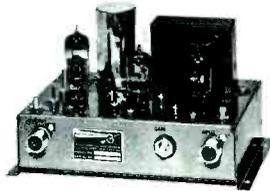
**Low band amplifier, Model ABB-16.** Covers Channel 2-6 and FM. Self-contained power supply. Gain: 35 db midband. Adjustable slope 0 to 4 db rising. Output: .3 volts per channel or 2 volts composite. 75 ohm input and output impedance. Flat bandpass. Net: \$75.00.
