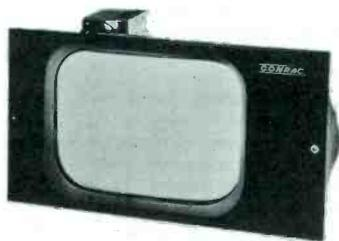
**General purpose video monitor, Model CLB.** Designed for continuous duty operation. Video response flat to 10 Mc for maximum resolution of 800 lines. Horizontal and vertical linearity within 2% of picture height. Taps available on horizontal output transformer—so unit can be operated full scan or reduced scan. Built-in switch allows selection of either composite video or separate video and composite sync. Parallel jacks for loop-thru operation. Net: \$315.00.
