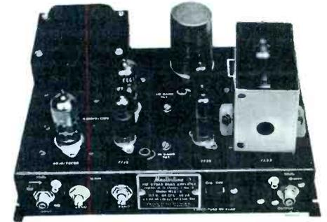
**All-band distribution amplifier, Model TSC-4200.** Gain: 30 db (minimum) low band, 37 db (minimum) high band. Maximum output: 1.7 volts low band (Channels 2-6 for 1% cross modulation), 1.7 volts high band (Channels 7-13 for 1% cross modulation). Tilt control range: 6 db low band, 4 db high band. Covers FM band. Separate high and low band gain controls. Ruggedized tube types. Net: \$71.00.
