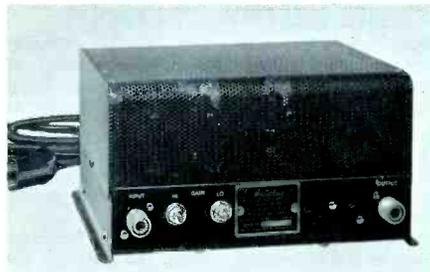
**Line amplifier, Model MLA-C.** Provides at least 40 db gain on all VHF channels. Separate gain controls for channels 7-13 and 2-6. Separate tilt controls. Maximum output (across 75 ohms) 2.0 volts per band for less than 1% cross-modulation. 3.5 volts per band for less than 3% cross-modulation. Net: \$93.50.
