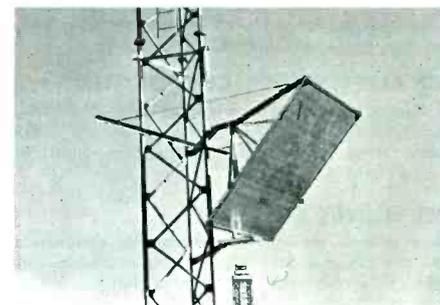
**Microwave passive reflectors.** Made of Reynolds aluminum interlocking extrusions. Three standard sizes; 6 x 8', 8 x 12' and 10 x 15'. Weight of reflectors is 140, 280 and 438 pounds respectively. Easy field assembly.
