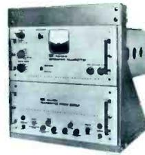
Wide-band microwave equipment for the 5925 to 8100 Mc range and 10,500 to 13,250 Mc range. Equipment is self-duplexing for multi-channel operation without additional equipment. System response within 0.25 db from
