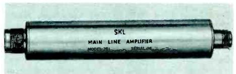
**Low band amplifier, Model 251.** Covers 20 to 100 Mc. Operates from 28 vdc. Noise figure: 8 db at 100 Mc. Cable powered with ALC unit to compensate for temperature changes. Gain: 17-25 db. All transistorized, cascaded. Net: \$310.00
