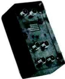
**Low band bridging amplifier, Model TR-4W.** Covers 30 to 110 Mc. Gain: 14 db across bandwidth on 4 outputs. Remote powered from 20 to 30 vac or + DC source. 20 db variable pad on input for gain control. Maximum of 1 db thru loss. Weatherproof aluminum housing. Net: \$58.00.
