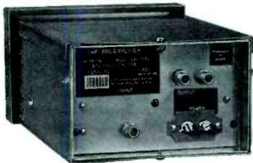
**UHF preamplifier, UAP series.** Six models to cover entire UHF range. Model UAP-7276 especially designed for MPATI areas and has 75 ohm input plus two 75 ohm outputs. Other models have 300 ohm input and output. Gain: 16 db at each of 2 outputs on UAP-7276 and 15 db on other models. Units have remote power supply. RF head is enclosed in rugged, irradiated housing. Stabi-Life circuit for long tube life. PNS.
