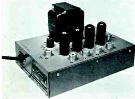
**Low band bridging amplifier, Model BA-4C.** Four distribution line outputs. Factory aligned to provide higher gain on low channels to compensate for normal tilt in the preceding trunkline amplifier. Gain: 3 db at Channel 2 and unity gain at Channel 6. Channel bandwidth. 75 ohm thru line and 75 ohm distribution line output. RF isolation between input and output is 45 db. Net: \$112.50.
