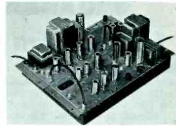
**Push-pull sub-channel amplifier, Model SDX-440.** Covers 4 to 47 Mc. 60 db second order beat suppression. Voltage stabilized transformer. Built-in AGC. Manual gain and tilt control. Built-in filter by-pass. Gain: 25 db (at 47 Mc). 6 db gain control range. Output: 36 dbj (operating). 75 ohm input and output impedance. F-61 fittings. Self-contained power supply. PNS.
