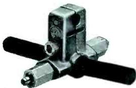
**Tapoff, outdoor type, Model PT.** Will accommodate two tap-offs from single block. Choice of capacitive or resistive inserts. Available for 4 different cable types. 1— for RG-11/U, single shield; 2— for RG-11/U double shield and jacket; 3— for 1/2" Foam or Solid dielectric; 4— for 3/8" Foamflex. PNS.
