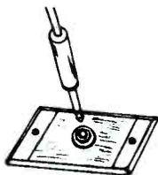
**WBT-4**—Choice of 4 taps (10, 15, 20 and 25 db) by removing parallel capacitors. Mounted on telephone wall plate. 59/U solderless feed-thrus. 1½" x 1½" metal box with phone jack outlet which mates CAS CT-8 transformer cable. (New Product) Net: \$1.45.
