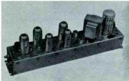
**TV sound originator, Audio Master.** Originates TV signal for any specified VHF channel. Provides crystal-controlled unmodulated video carrier plus sound carrier which may be modulated by any audio source. Audio carrier is 4.5 Mc above video frequency (TV Standards). Output impedance is 75 ohms. Net: \$175.00.
