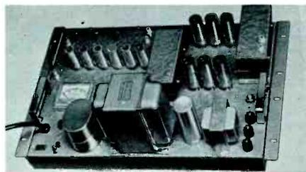
**Low and sub-band amplifier, Model LSA-795.** Built-in variable line equalizer. Built-in voltmeter. Response: 7 to 95 Mc. Voltage regulated power supply and "Stabi-Life" feature. Built-in distribution amplifier. Gain: 36 db maximum at 90 Mc. Noise figure: 8 db. Manual gain control variable over 0-4 db range. Output: 42 dbj at 90 Mc. PNS.
