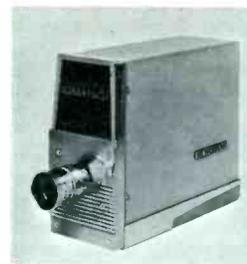
**Automatic transistORIZED camera, Model TTVC-1-1.** Self-contained, rugged, portable (15 lbs.), this camera transmits high definition (650 line resolution, 2 to 1 interlace) pictures. Has built-in automatic light compensator that adjusts for continuously changing light over a 2000 to 1 range. Video output, 1.25 volts. Usable picture may be obtained with as little as ½ foot candle of scene illumination with the standard F/1.9 lens supplied. Net: \$1950.00.
