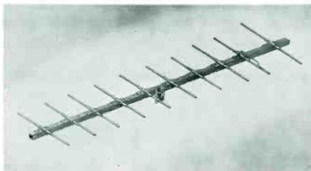
**Single-channel yagis, Y-100 series.** Designed for long lasting trouble-free performance under the most rigid weather conditions. Antennas are twin-driven design. Flat-across-the-channel performance. Extra heavy-duty construction using a 2" square crossarm with 3/4" elements and 7/8" reinforcing sleeves on Y-104 low band antennas. Nominal gain: 11.2 db low band. High band models (Y-103) utilize 1 1/4" square boom
