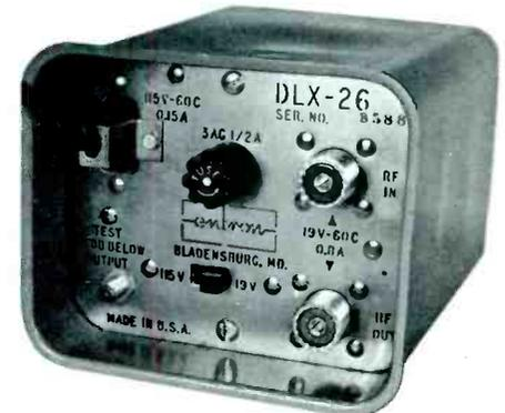
**Low band line extender, Model DLX-26.** Will extend distribution lines up to 2,000' using low loss cable or 1,000' using standard cable such as RG-11/U. Gain: 20 db. Noise Figure: 9 db. Self-contained power supply with power requirement of either 115 vac, 12 watts or 19 vac, 12 watts. (For remote powering use RPS-B power supply.) Output level: +41 dbmv. Net: \$120.00.
