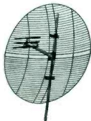
**UHF parabolic dish antennas, 3065 series.** Designed for MPATV areas. Withstands 100 mph winds and heavy icing. Gain: 17 db. 75 and 300 ohm versions. 75 ohm model uses slot-fed dipole. 300 ohm model uses folded dipole with reflector. Dish constructed of 1/8" steel wire, spaced 1" and welded to 1/4" thick cross-members. Dish is coated with heavy vinyl plastic
