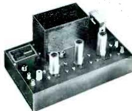
**Line-bridging distribution amplifier, Model UBC-26B.** Covers low band plus FM. Gain: 30 db minimum. Flat response. Maximum output: 47 dbj\* for 5-channel operation. Less than 0.3 of 1%
