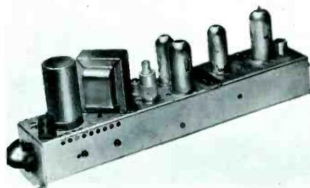
**AGC controlled amplifier, Model MCSc.** For single channel useage except for MCSc-FM which covers the entire FM band. Gain at least 46 db (low band); 38 db (ch. 7-10); 35 db (ch. 11-13). Maximum output; 1.0 volts for less than 1% cross-modulation; 2.0 volts for less than 3% cross-modulation.
