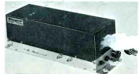
**All-band distribution amplifier, Model A-700.** Will drive up to 150 TV/FM sets. Designed for hotels, large motels, apartments, cable systems. Gain: 44 db on low band and FM; 44 db, high
