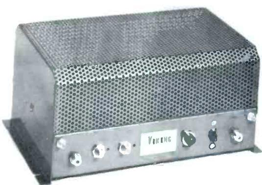
The VIKING BROADBAND AMPLIFIER is an amplifier designed for the future. It amplifies the entire low and high TV band and the entire FM band at 40 db.
