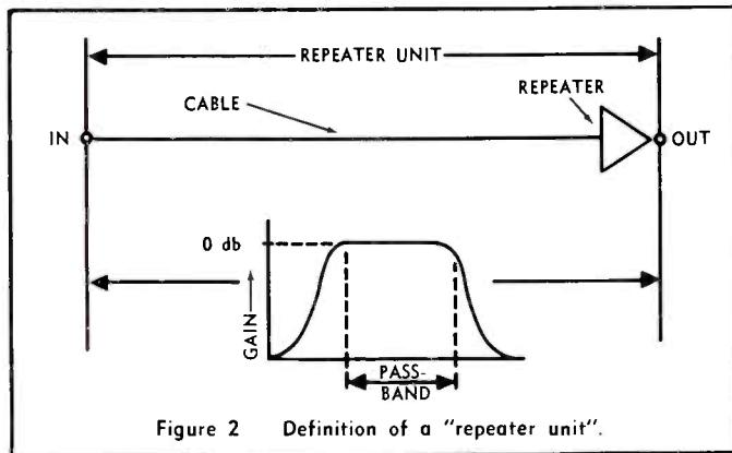
Figure 2 Definition of a "repeater unit".
