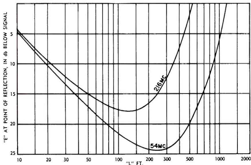
Figure 1. Minimum permissible return loss in RG 11/U coaxial cable as a function of the distance between point of observation and source of echo.
