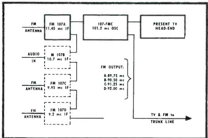
The CAS CATV/HEAD-end system is a method of providing several FM signals from standard FM or any audio source, with one basic system.
