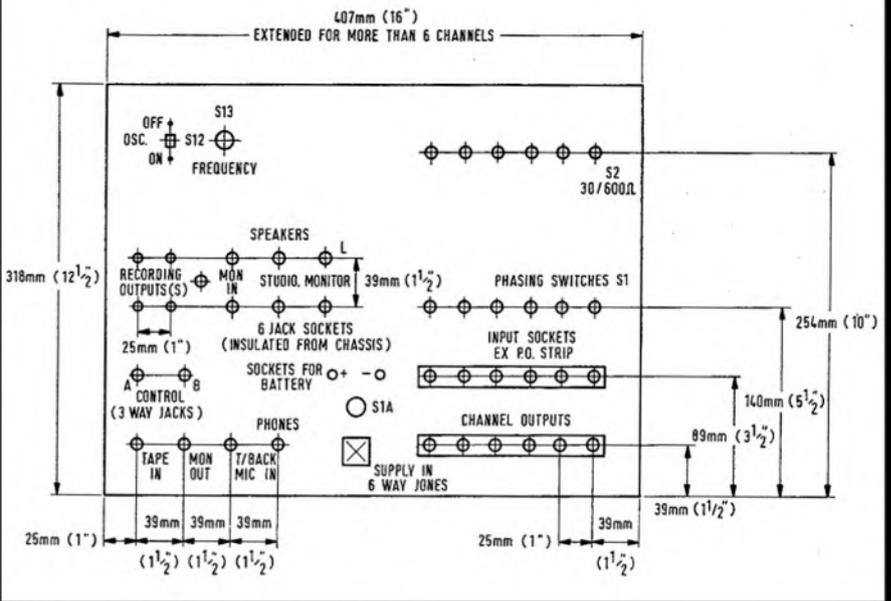
FIG. 5 FRONT PANEL MAIN DIMENSIONS
