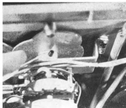
**FIG. 3** Solenoid flap armature held off at its limit.
