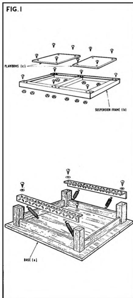
are not given as these depend on the size table available. Next, cut the angled metal as required. In the prototype, it was only necessary to drill four  $\frac{1}{8}$  inch diameter holes for the springs. Large wood screws with washers were used to fix the angle pieces to the base. When the angle pieces have been drilled, screw them into place. Note that the base must be big enough to allow the suspension frame and platforms plenty of clearance. (At least 150 mm all the way round.)
