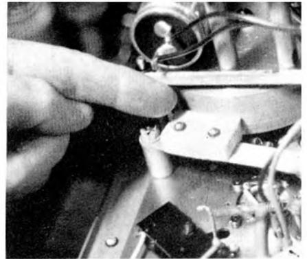
**FIG. 5** Flywheel brake and autostop switch.
